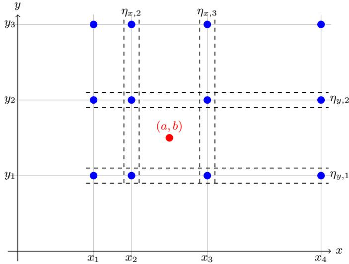
**Figure 2.9:** 2D PWL Approximation to estimate  $f(a, b)$  (adapted from Hoffmann (2014); Angga (2019))
