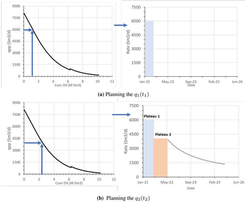
**Figure 2.2:** Production planning with production potential approach
