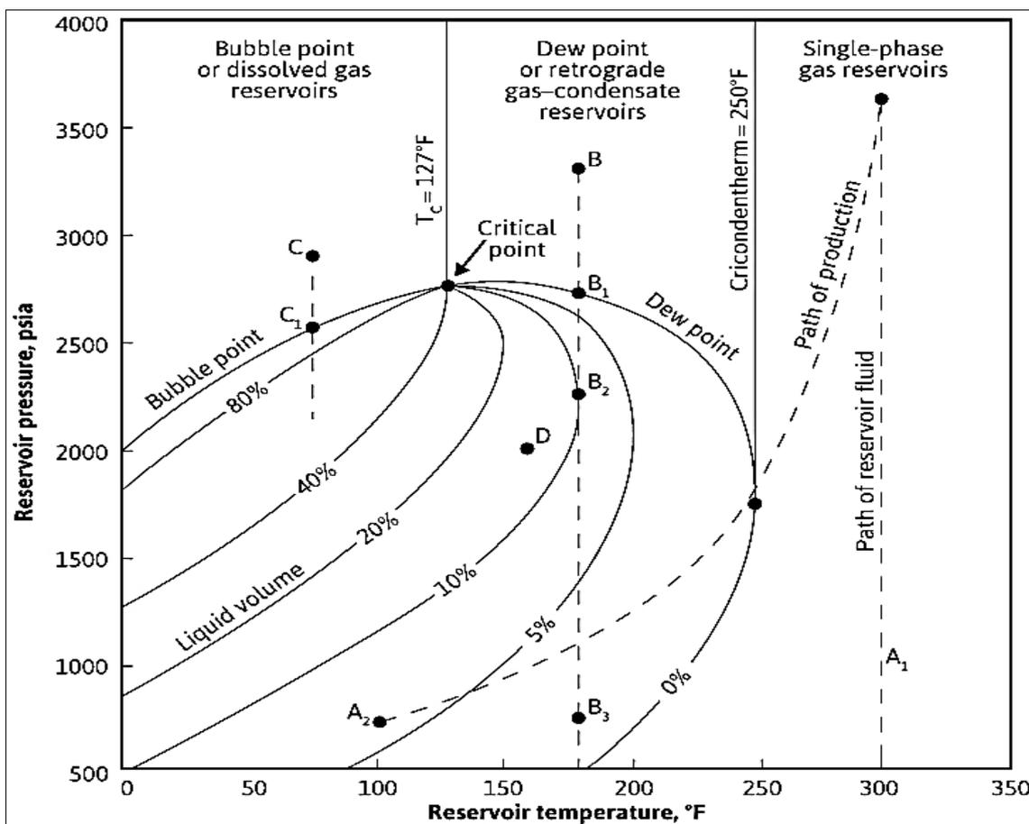
Figure 2. 4 P-T Envelope of Different Depletion Reservoirs[8]
