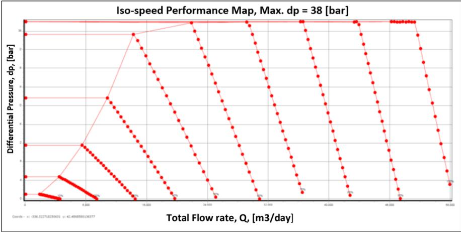
**Figure 3. 8 Typical Iso-Speed Performance Map, Max. dp = 38 [bar], from PIPESIM**
