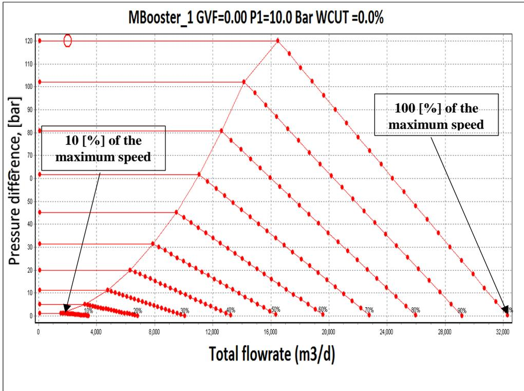
**Figure 3. 2 Multiphase Booster's Iso-speed Performance Map**
