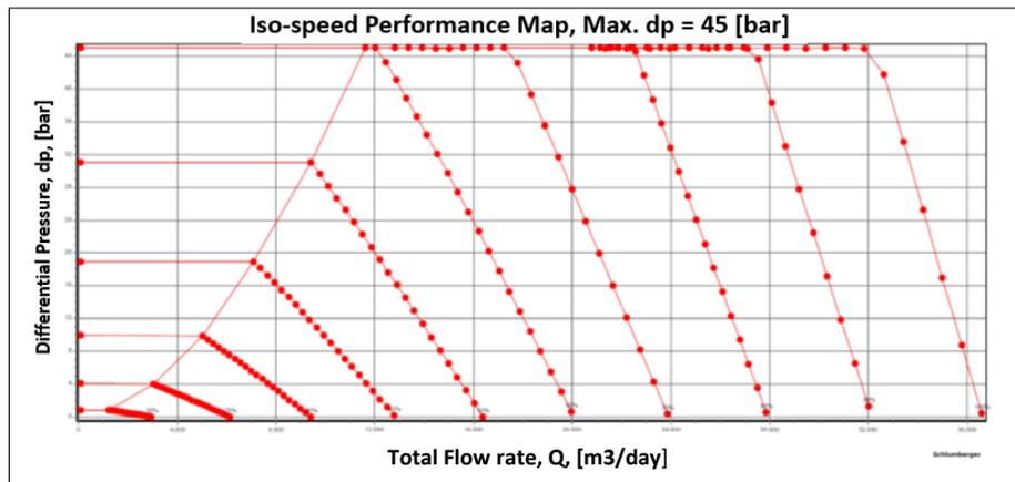
Figure 3. 9 Typical Iso-Speed Performance Map, Max. dp = 45 [bar], from PIPESIM
