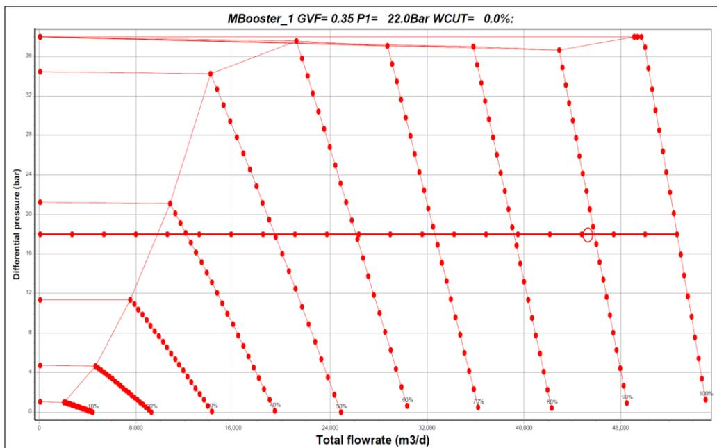
**Figure 3. 24 PIPESIM Output, Iso-speed Performance Map, Test Case 4**
