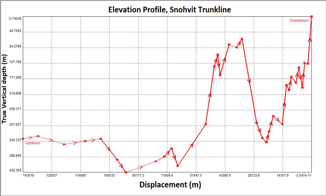
**Figure 4. 11 Elevation Profile Of Trunk Line, Snøhvit Field[23], Set On GAP**
