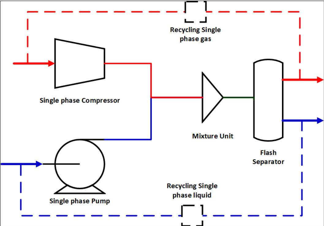
Figure 2. 6 Proposed Hysys Model for Direct Integration Approach(DIA)
