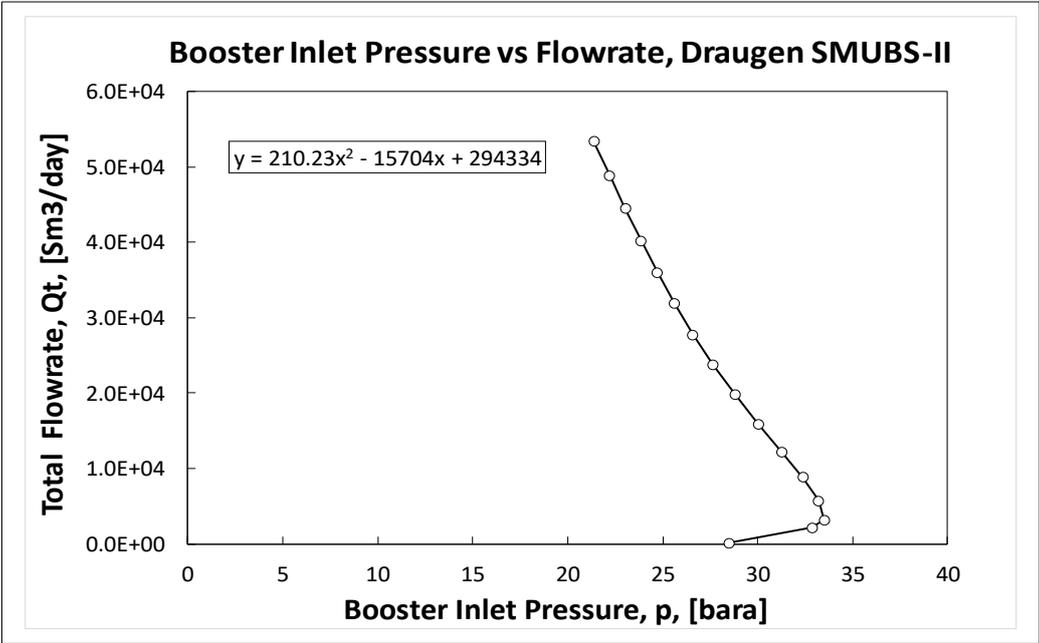
**Figure B 1 Relation Between Booster Inlet Pressure and Producibile Flow rates**
