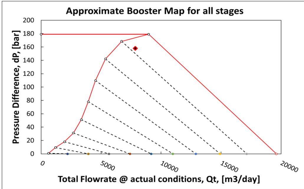
**Figure 3. 21 Approximate Iso-speed Performance Map, Test Case 3**
