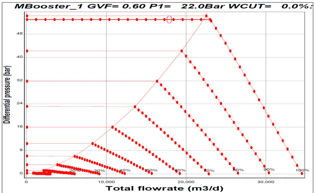
**Figure 3.18 PIPESIM Output, Iso-speed Performance Map, Test Case 1**
