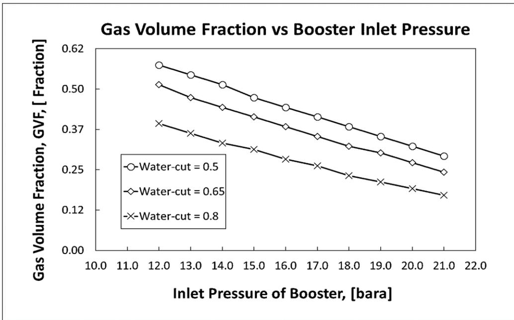
Figure 5. 8 Relation Between Booster Inlet Pressure And GVF
