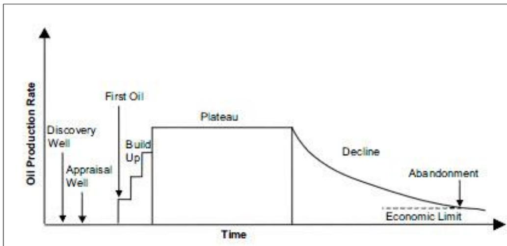
Figure 1. 1 Typical Oil Field's Production Profile[3]
