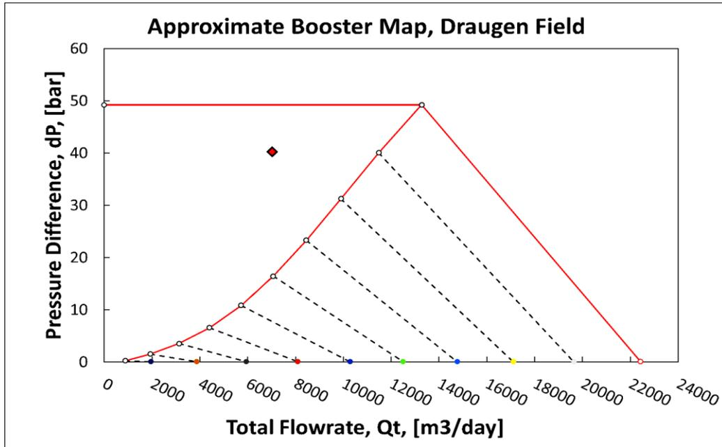
Figure 5. 11 Draugen Field, Generalised Iso-speed Performance Map
