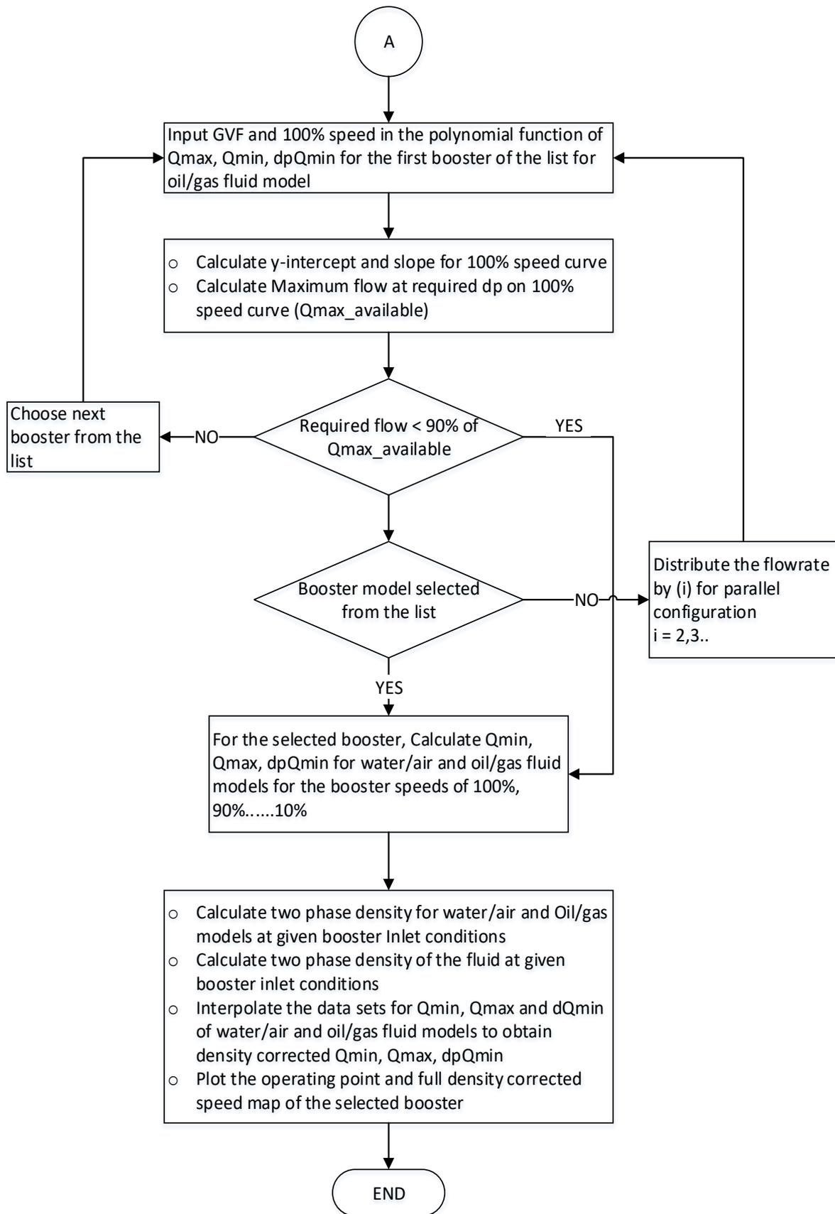
**Figure 3. 16 Process Flow Diagram for The Booster Selection**
