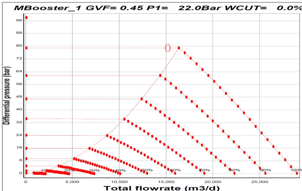
**Figure 3. 20 PIPESIM Output, Iso-speed Performance Map, Test Case 2**
