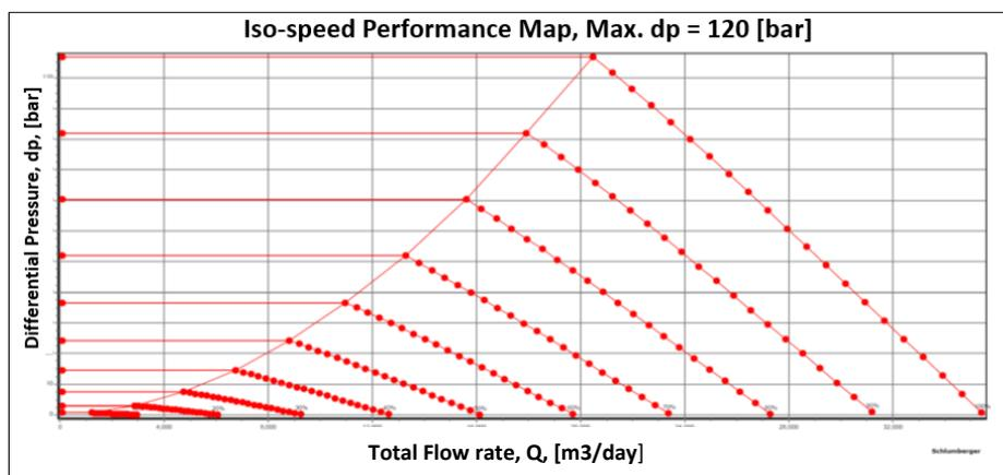
Figure 3. 10 Typical Iso-Speed Performance Map, Max. dp = 120 [bar], from PIPESIM
