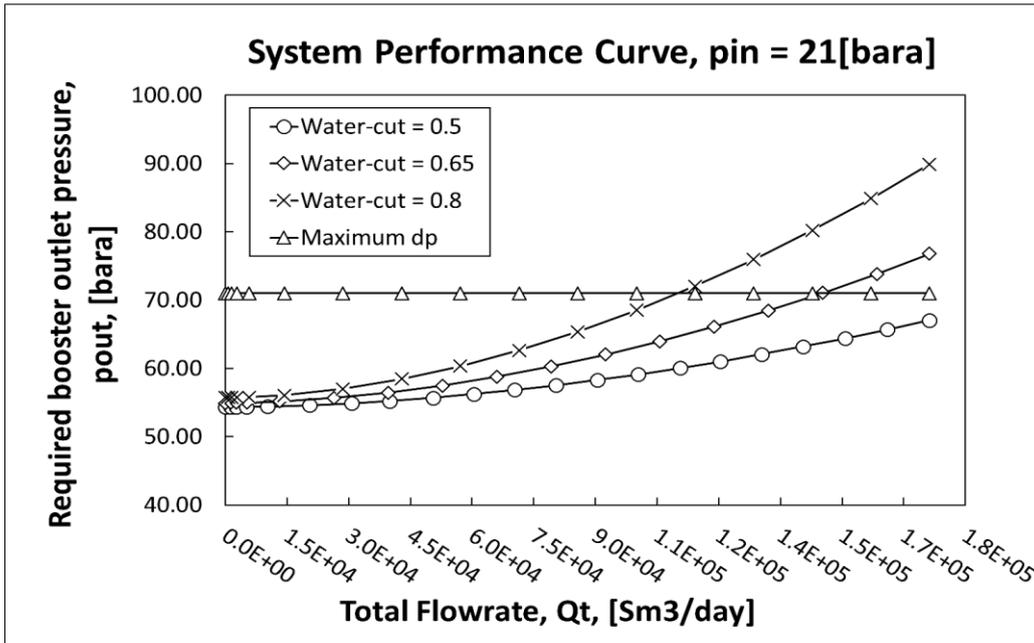
Figure 5. 7 System Performance Curves for Draugen Field
