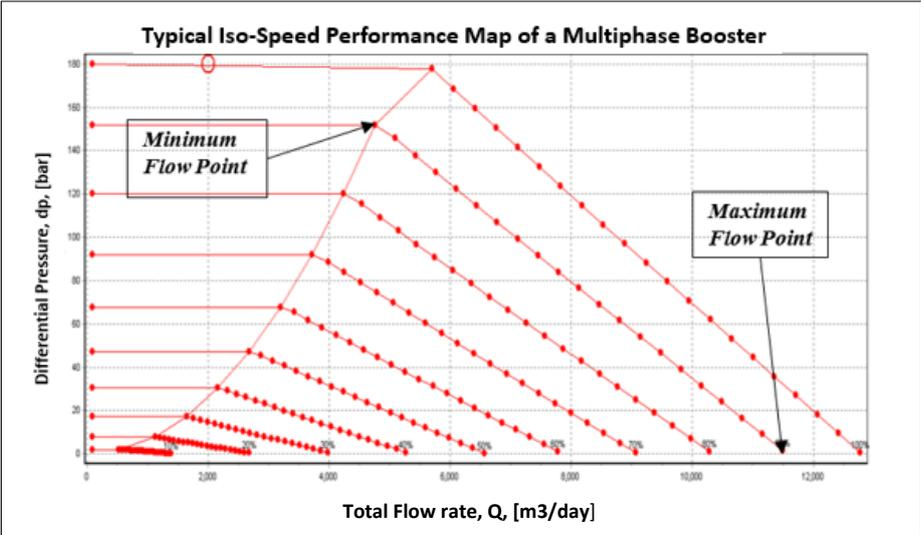
**Figure 3.12 Typical Iso-speed Performance Map of a Multiphase Booster, from PIPESIM**
