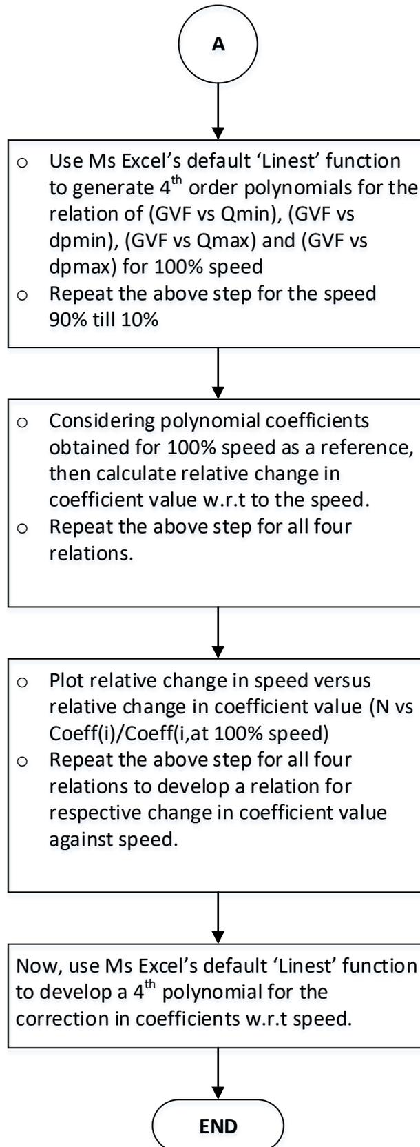
**Figure 3. 13 PFD for Empirical Equation Development for Multiphase Booster's Map, as a Function of GVF and Speed [%]**
