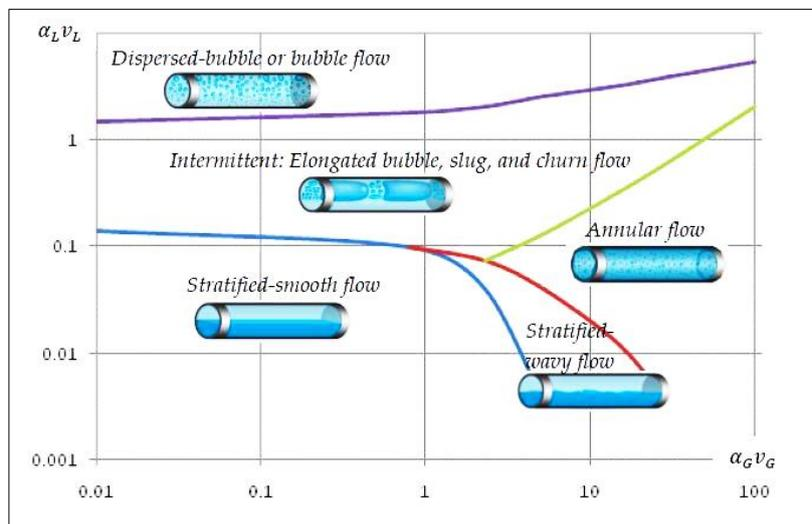
Figure 2. 1 Steady State Flow Regime Map, Horizontal Segment[7]
