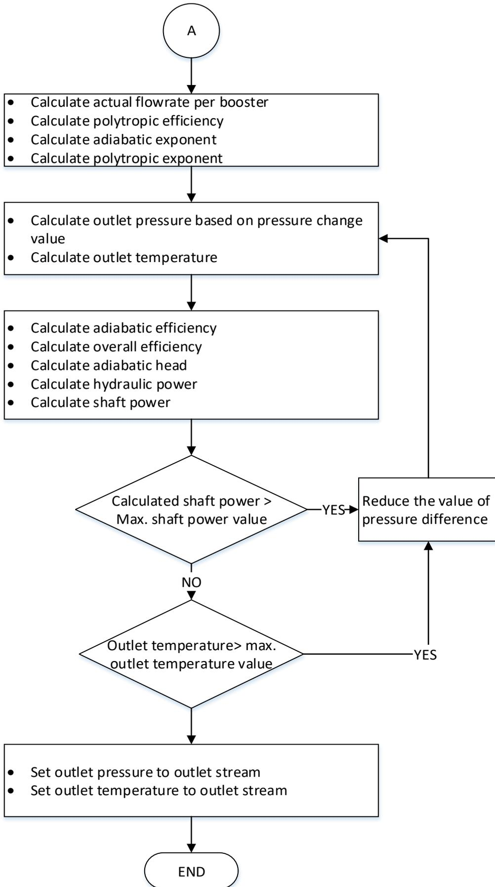
**Figure 4. 12 Process Flow Diagram for GAP Inline Element, Snøhvit Field WGC-4000**
