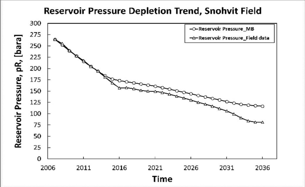
Figure 4. 8 Difference in Pressure Profiles, Snøhvit Field[26]
