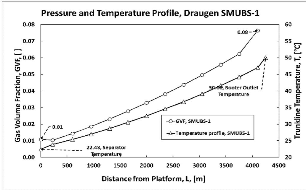
**Figure 5. 6 Pressure and Temperature Profile, Draugen SMUBS-I**
