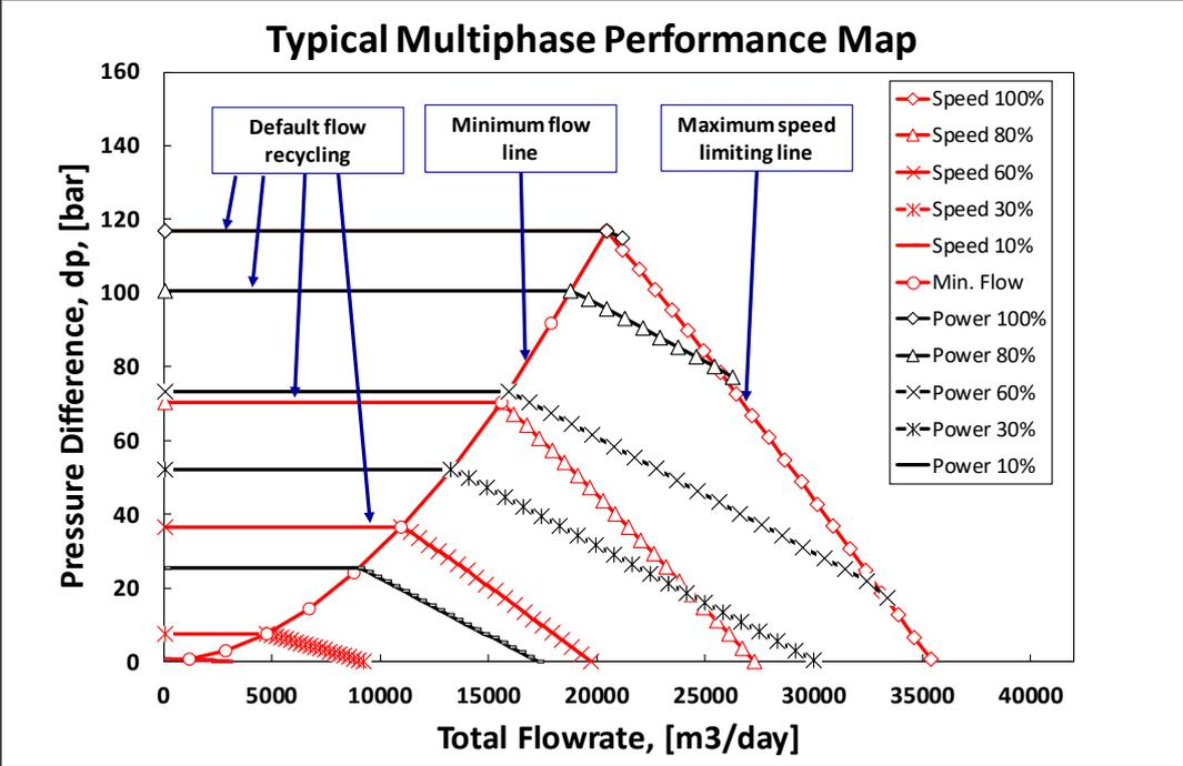
Figure 2.7 Generic Multiphase Performance Map, Obtained from PIPESIM
