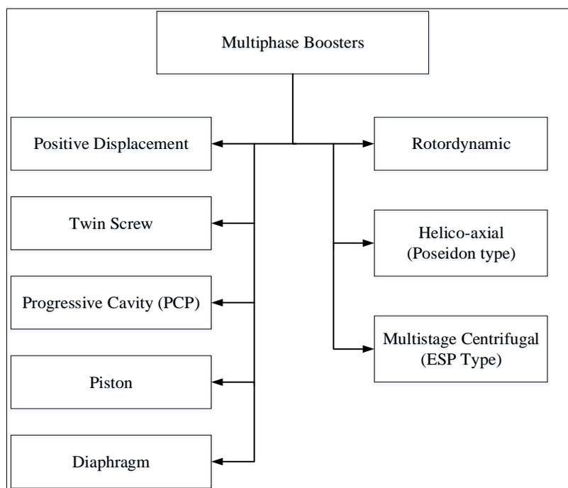
**Figure 2. 5 Classification of Multiphase Boosters[10]**
