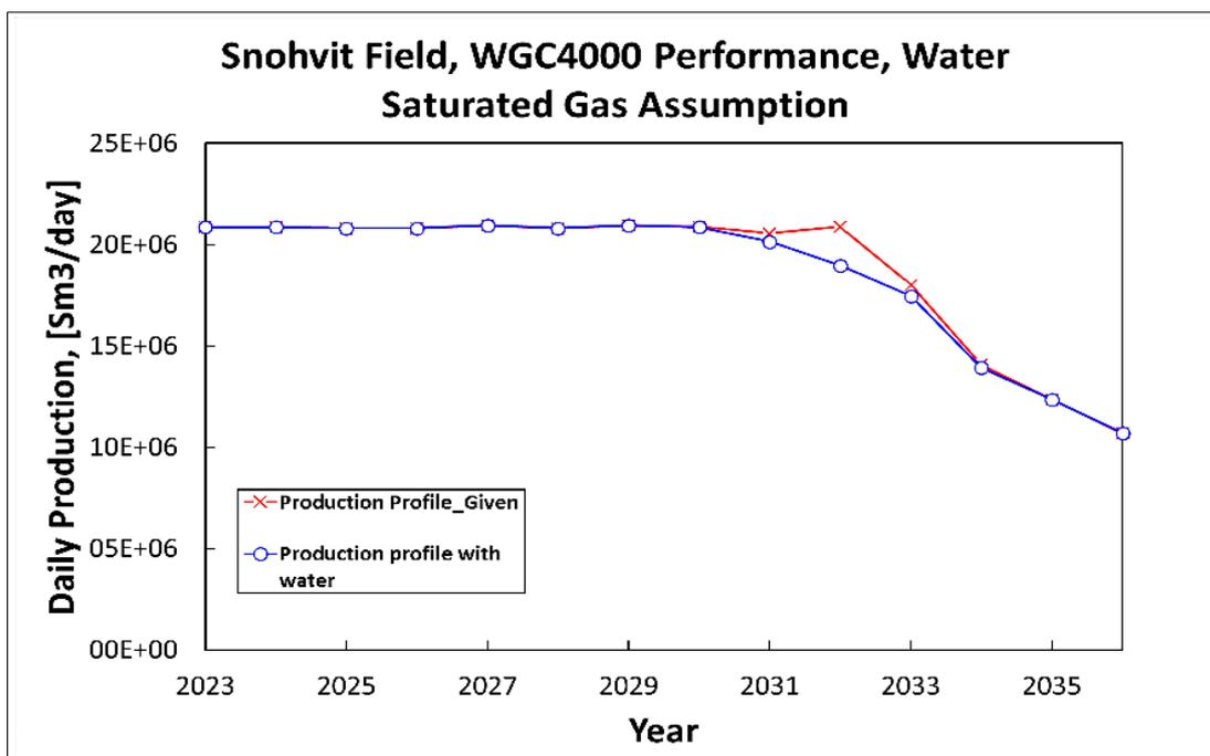
**Figure 4.15 WGC-4000 Performance, Snøhvit Field, Gas Saturated with Water[23]**
