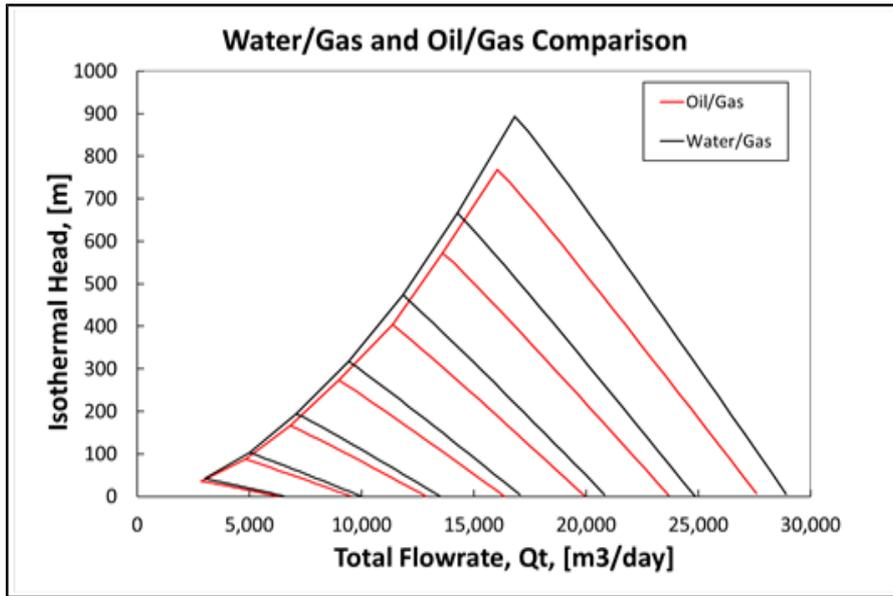
**Figure 3. 5 Iso-speed Performance Map for Oil/Gas and Water/Gas, GVF=40[%]**
