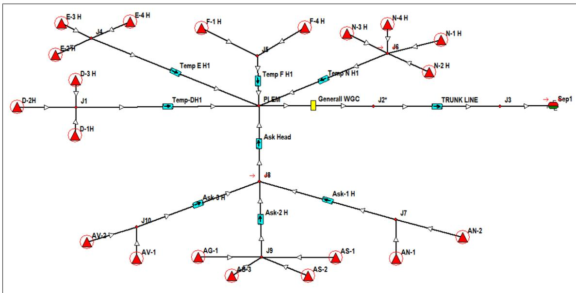
Figure 4. 13 Gap Network Simulation Model, Snøhvit Field
