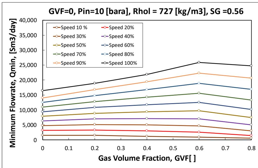
**Figure 3. 3 Variation in Minimum Flow Line w.r.t GVF**
