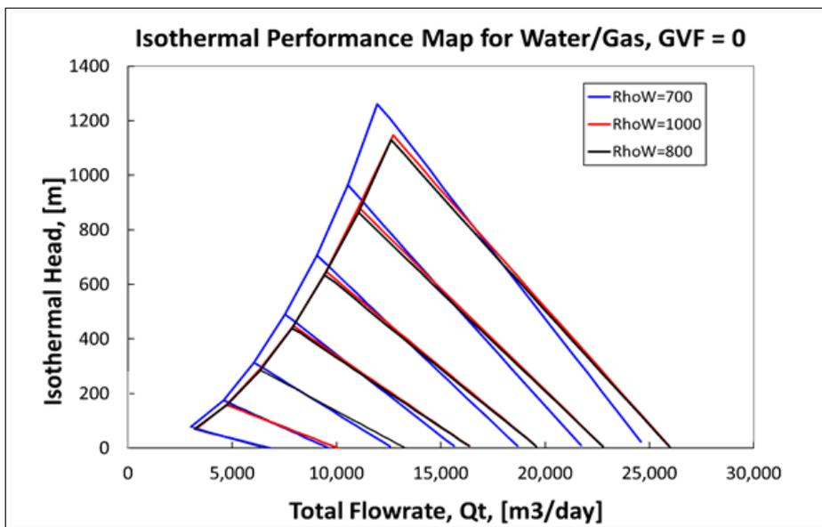
**Figure 3. 6 Iso-speed Performance Map with Different Water Densities, GVF=0[%]**
