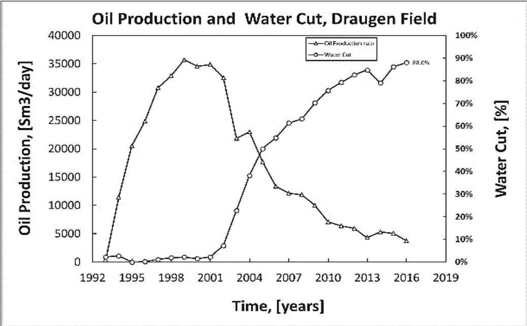
Figure 5. 3 Production Profile and Water-Cut, Draugen Field[29]
