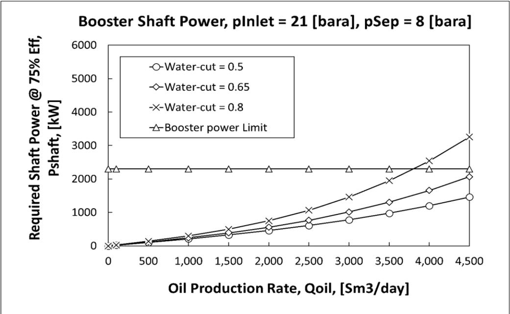
Figure 5. 10 Power Defined Oil Rates, Draugen Field, Sep. Pressure =8 [bara]
