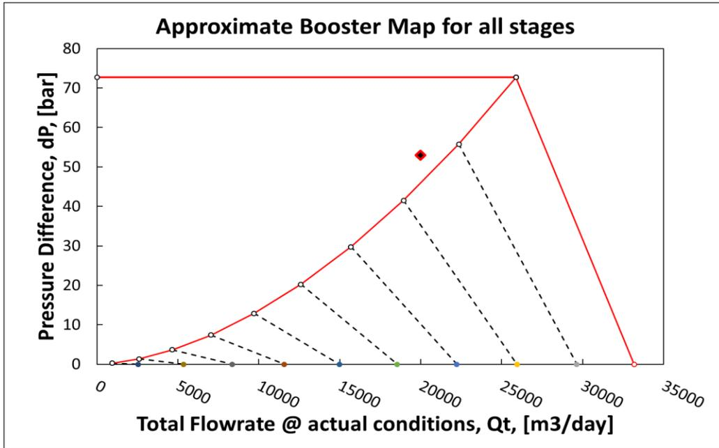
**Figure 3.17 Approximate Iso-speed Performance Map, Test Case 1**
