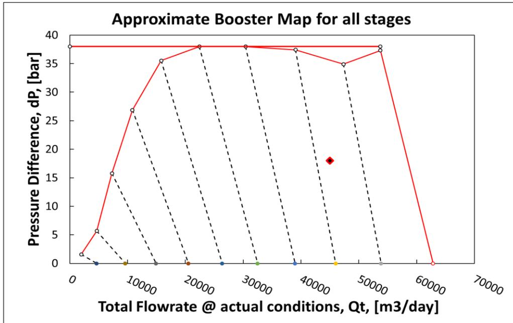
**Figure 3. 23 Approximate Iso-speed Performance Map, Test Case 4**
