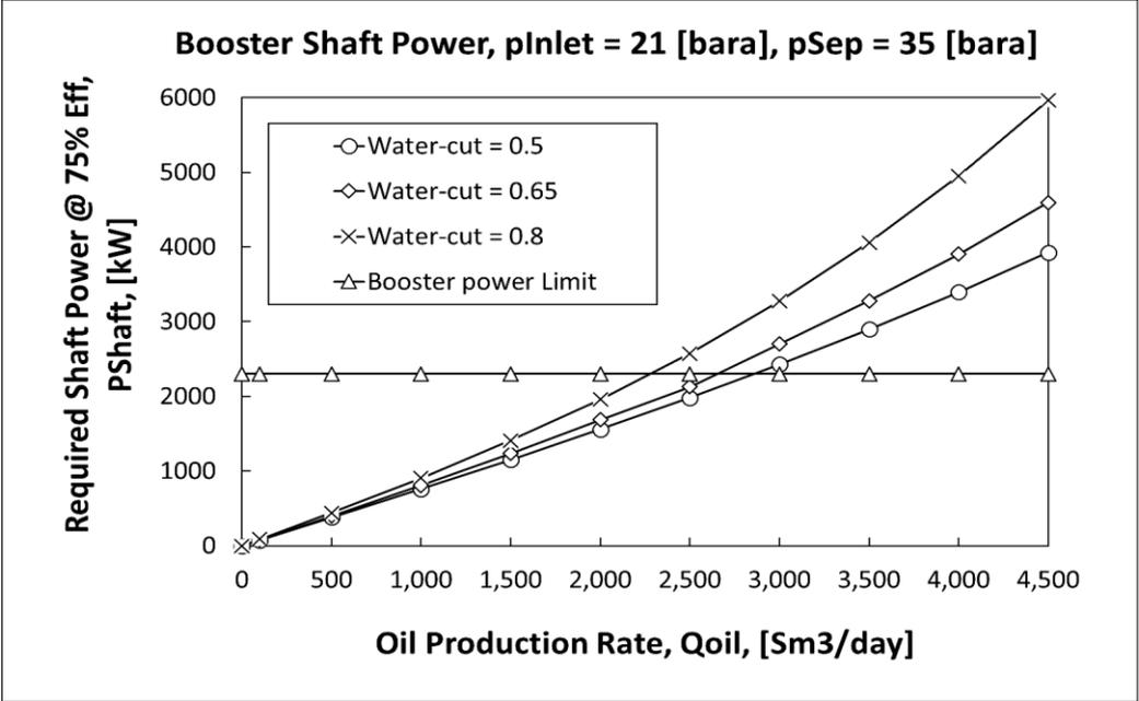
Figure 5. 9 Power Defined Oil Rates, Draugen Field, Sep. Pressure=35 [bara]
