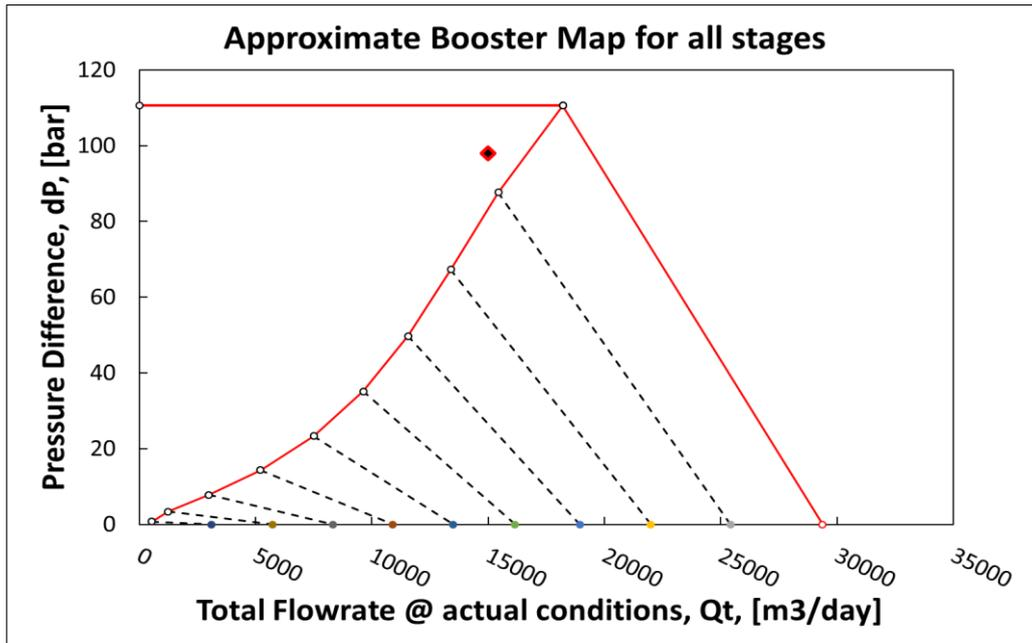
**Figure 3. 19 Approximate Iso-speed Performance Map, Test Case 2**
