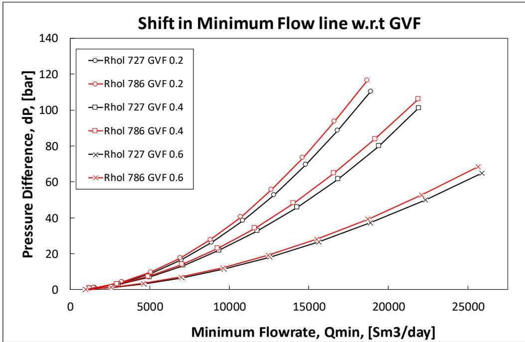
**Figure 3. 4 Decline in Minimum Flow Line w.r.t Density**
