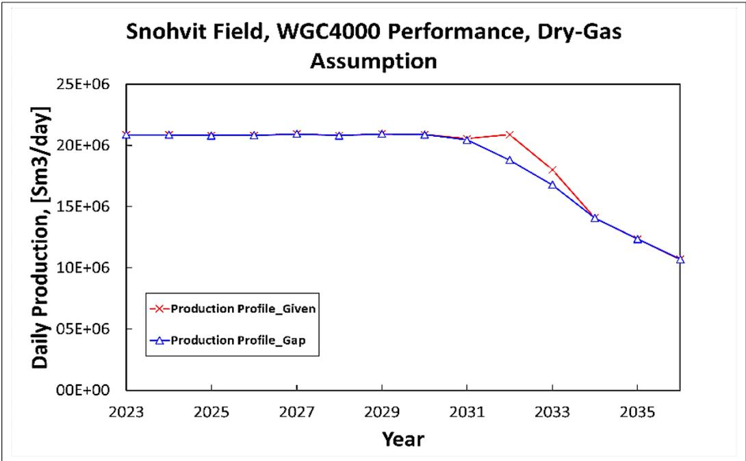
Figure 4. 14 WGC-4000 Performance, Snøhvit Field, Gas Under Saturated with Water[23]
