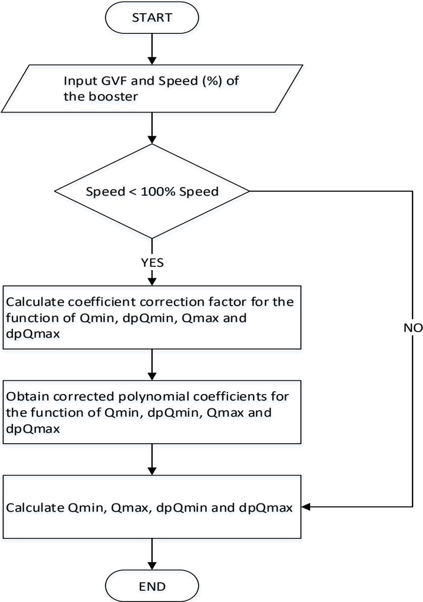
**Figure 3. 14 Process Flow Diagram to Generate Iso-Speed Performance Map**
