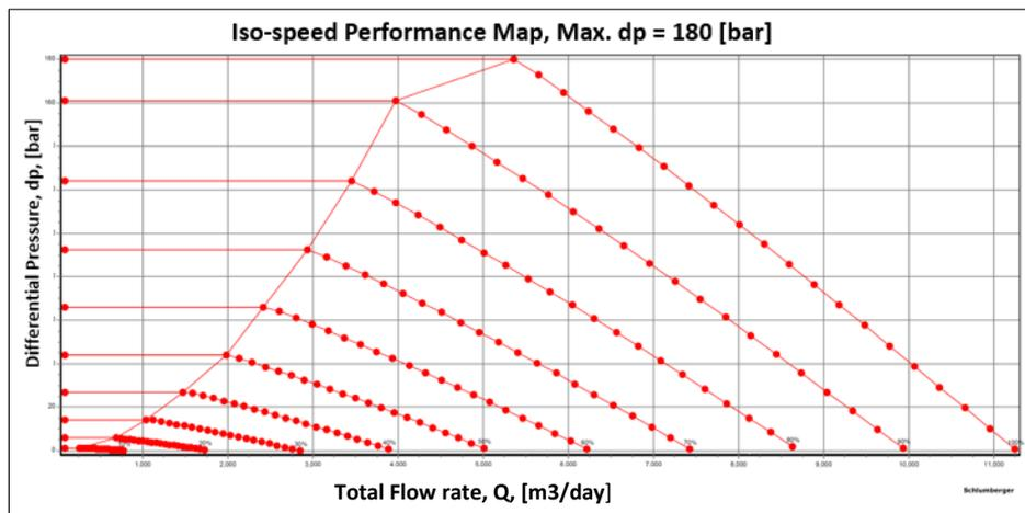
Figure 3. 11 Typical Iso-Speed Performance Map, Max. dp = 180 [bar], from PIPESIM
