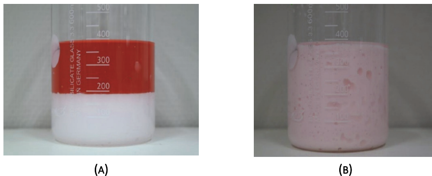
FIGURE 7-22. A) OIL (RED) AND WATER (WHITE) ORIGINALLY SEPARATED, B) OIL AND WATER EMULSION AFTER VIGOROUS STIRRING IN A BLENDER. PHOTOS TAKEN BY HONG [7-4]
