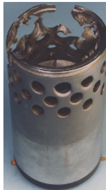
FIGURE 7-13. EROSION DAMAGE IN A CAGE-TYPE CHOKE [SOURCE UNKNOWN]
