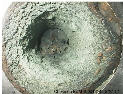
FIGURE 7-12. SCALE ACCUMULATION IN CHOKE (IMAGE TAKEN FROM SANDENGEN [7-2] )
