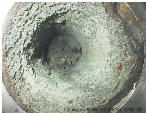
FIGURE 7-12. SCALE ACCUMULATION IN CHOKE (IMAGE TAKEN FROM SANDENGEN [7-21] )
