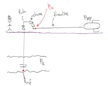
Assume that the wellhead choke is 20% closed and that the system is producing a dry gas rate of 2.0 E6  $Sm^3/d$ .
