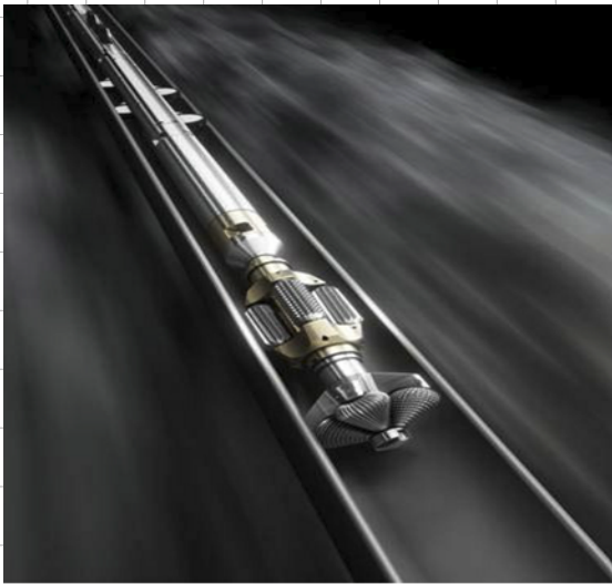
5.23 Cable tractor, equipped for milling (Aker solutions 2010)
