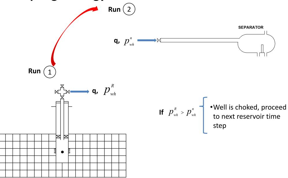
• Loose coupling with bottom-hole coupling –most typical
