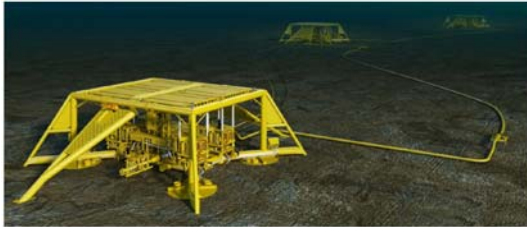
Figure 3.3 Typical NCS tie-back solution (Image: Statoil ASA)
