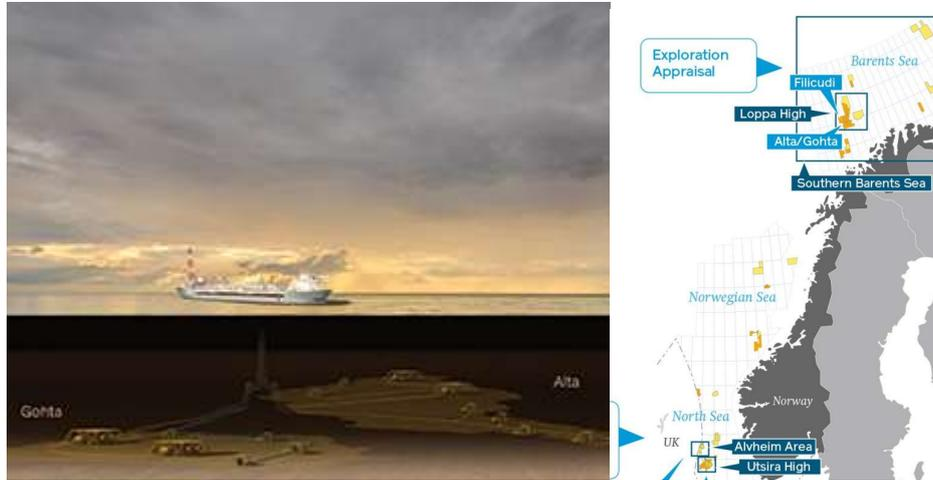
The reservoir management team of Lundin is currently developing the field. They are evaluating to produce the field with **field plateau rate** of 12 000 Sm<sup>3</sup>/d. Each reservoir will be produced independently to the FPSO, via a separate pipeline. The oil production potential **of each individual reservoir versus its cumulative oil production and its number of wells** can be estimated with following expression (available as a VBA function in the Excel sheet provided):
