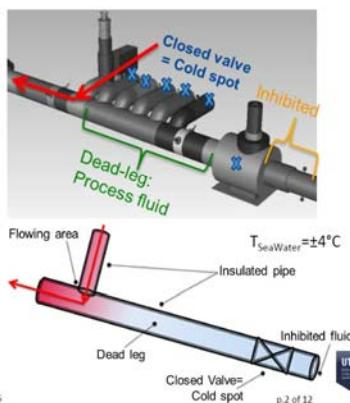
design of dead-leg geometry must be analyzed during FEED studies.
