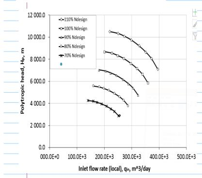
this map is made with measured performance conditions generated at a test facility
