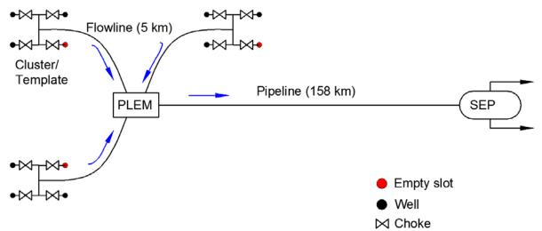
You are asked to perform a steady-state, 1D simulation using the simulator Hysys to compute pressure and temperature drop along the main transportation pipeline from the PLEM to the slug catcher. The main goal is to assess hydrate formation. You have to perform your calculations for two points in time of the system: plateau and decline.
