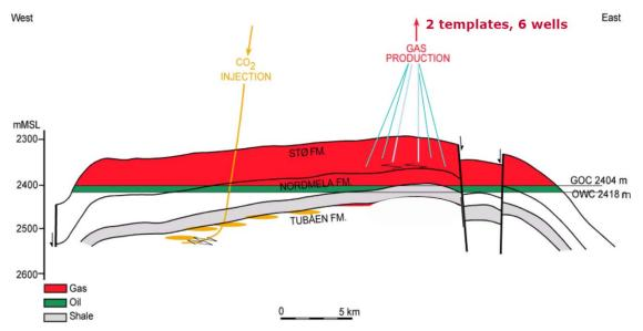
The development details are still very uncertain but the initial proposal is to develop the field using 6 subsea wells and a long pipeline to shore, to an LNG plant located on Melkøya. Due to the fact that it is a standalone development, and that the LNG plant is very costly, the
