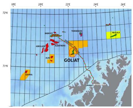
The field consists mainly of a single reservoir unit located in the Stø formation with a initial gas in place of 270 billion standard cubic meter, at an initial reservoir pressure of 276 bara and temperature of 92  $^{\circ}$ C.
