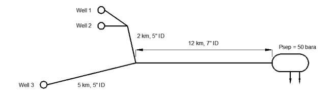
The wells have the same layout as the well created in the previous section, but with different GOR, WC and PI as specified in the table below:
