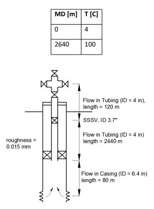
**Overall heat transfer coefficient** = 45 W/m<sup>2</sup> K
