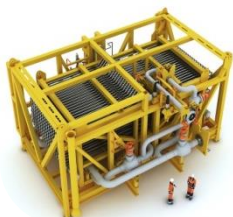
Inlet/antisurge cooler 235 tons 15x10x7m
