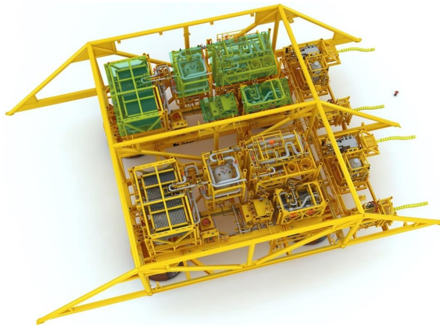
Compressor 289 tons 11x9x10m
