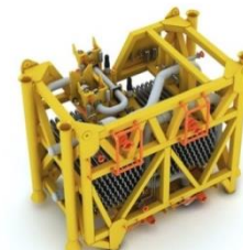
Outlet cooler 107 tons 9x7x5m
