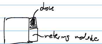
in shore wells the choke is placed in a special module to make it easy to retrieve
