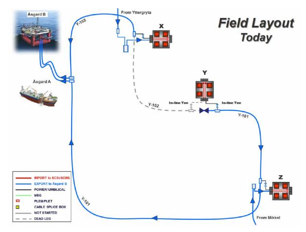
The subsea well templates are typical 4-well slot templates with the manifold module located in the center of the template. There is one well producing in template Z, 4 wells in template Y and 4 in template X. Your tasks are as follow:
