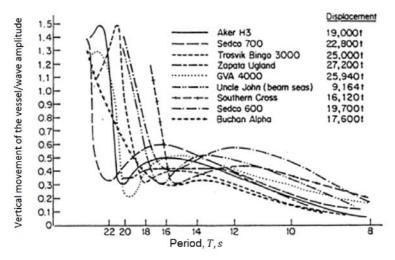
Your task is: if a wave with the peak period and the dominant wave amplitude found in part 1 impacts the semisub Sedco 600, what would be the expected vertical movement (heave) of the vessel?
