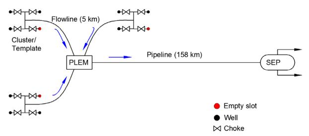
**TASK 1.** For initial reservoir pressure, compute the available pressure curve at the wellhead as a function of single well rate and the required pressure curve at the template as a function of single well rate. Plot the two curves and calculate the intersection point. What does this rate represent?
