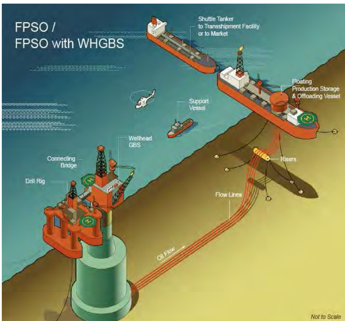
Figure 1.7-3: Floating Production, Storage and Offloading Facility with Wellhead Gravity Base Structure
