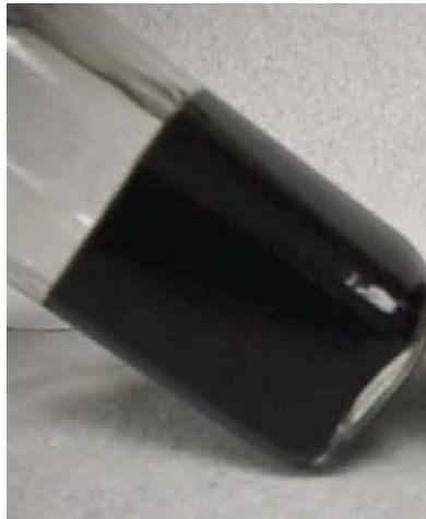
Fig. 16. Crude oil not flowing once the pour point is reached
