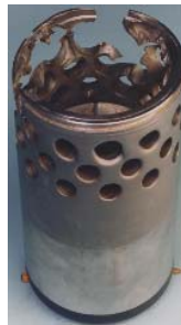
Fig. 10. Erosion damage in a cage-type choke.
