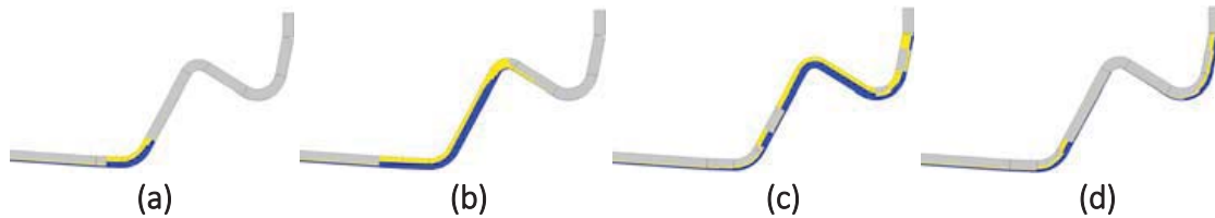
Fig. 8. Stages of severe slugging in an S-shaped riser.
