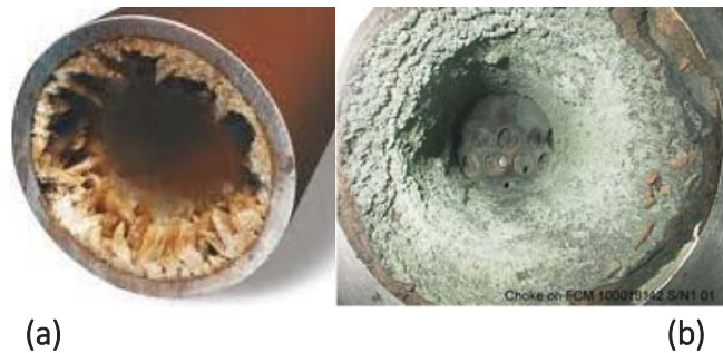
Fig. 9. Scale accumulation in a a) pipe, b) choke
