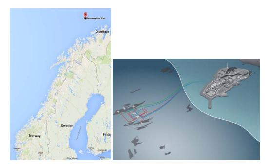
According to the base case Scenario (BCS) selected for the study, the field is completed subsea with three subsea templates, each with 4-slots.
