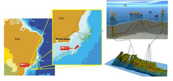
The field is developed with two fixed platforms from which wells are drilled and completed. There are 40 producing wells in total. The production is taken to an FPSO where the processing takes place. The separated water is transported back to the platforms and injected in the lower part of the formation.
