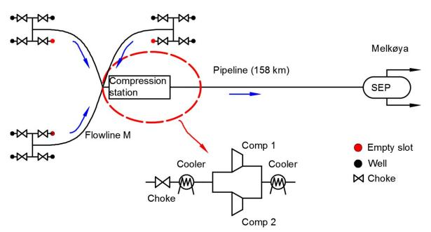
The compression station has a choke valve, a cooler and two identical compressors in parallel. In normal operating conditions, the choke is fully open. Some operational constraints are the following:
