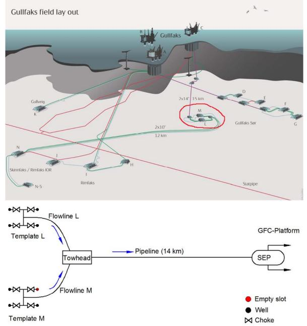
The field have been producing oil and gas since 1999. Due to the depletion of the oil layer in the formations, the wells from templates M and L have been recompleted in 2009 to produce liquid rich gas. The liquid comes from gas condensate in one formation and from mobile liquid oil in the bottom of the reservoir of the other formation. From 2009, the field is produced in plateau mode with a total rate of 10 E6  $\text{Sm}^3/\text{d}$ .
