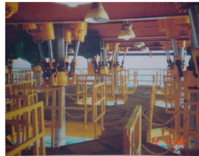
Figure 5.3: Production riser tensioner system at the TLP Joliet (National Oilwell Varco, 2007b).
