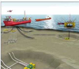
Satellite well system with subsea well. MODU or drill ship.
