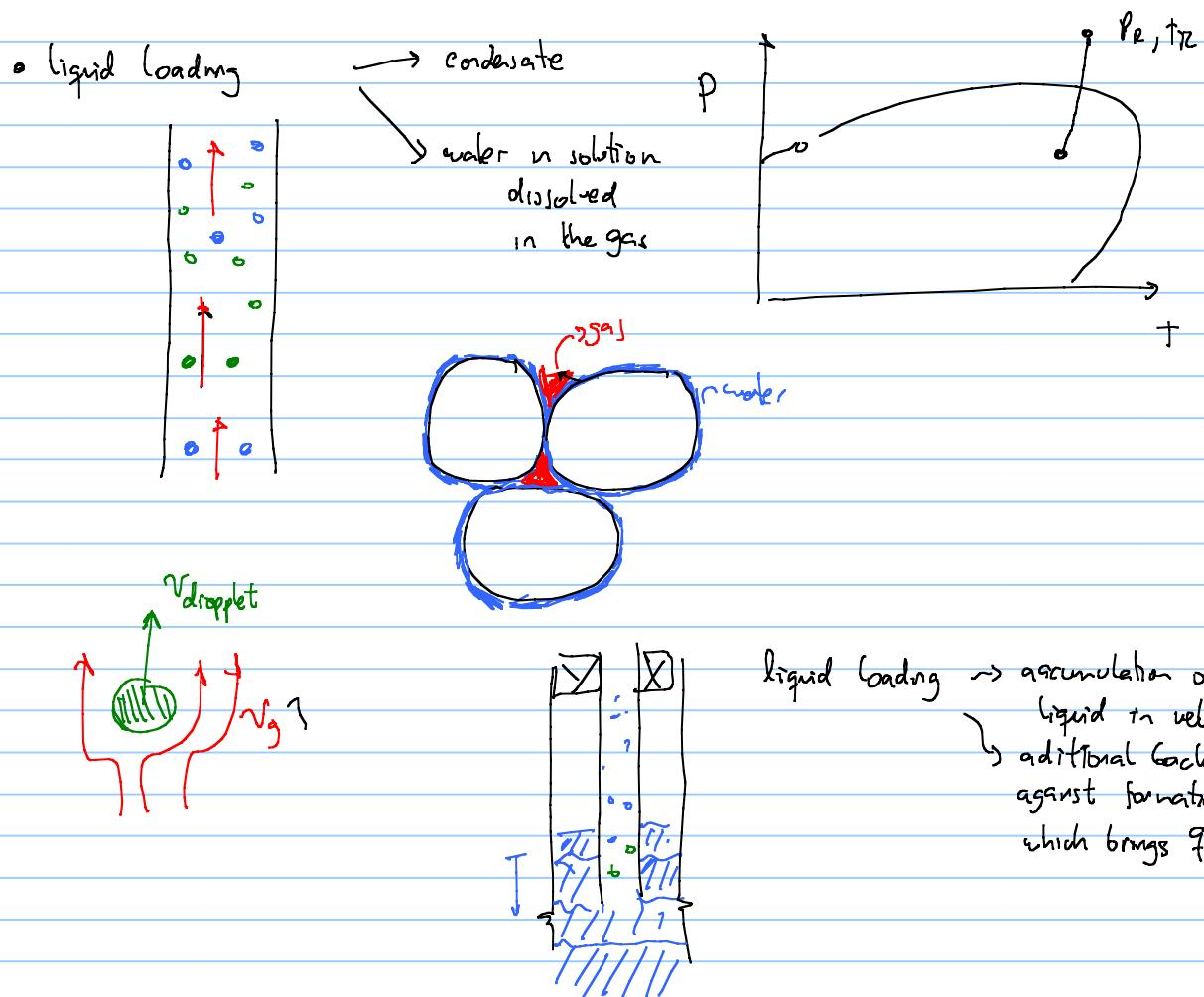
Select  $\phi$  of tubing such that  $V_g$  is high enough to lift droplets of liquid
