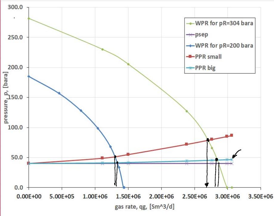
• pipeline sizing  $\rightarrow$  minimize  $\Delta p$ , maximize rate  $q_g$
