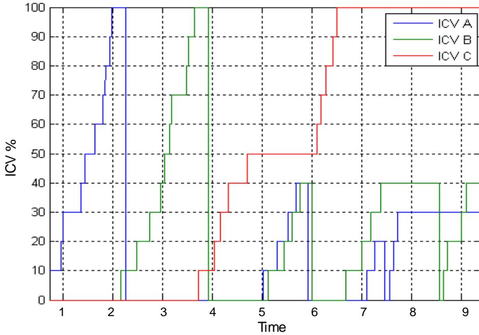
Figure 5: ICV testing sequence for a three zone well.
