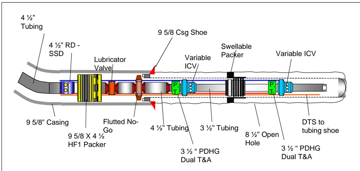
Figure 2: A typical smart well completion with two zones.
