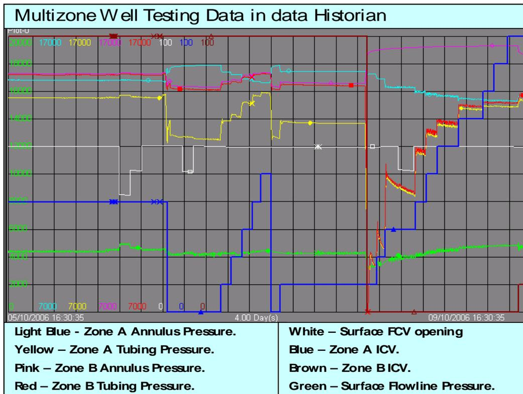
Figure 3: Typical multizone well test for a two zone well (Zone A and Zone B). The downhole and surface data is stored in a data historian and then retrieved into FW PU for modelling.
