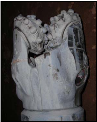
Figure 16: The side view of the insert bit with worn shirt tails.
