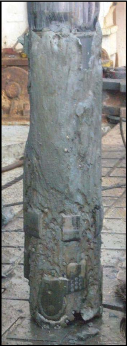
Figure 24: Lower rotating part of RSS BHA and drill bit from Well A. Clays in this area are very sticky and attach to the BHA.
