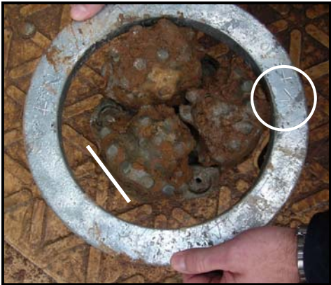
Figure 15: A dull bit in 8 1/2" ring indicates that the bit was more than 1" undergauge.
