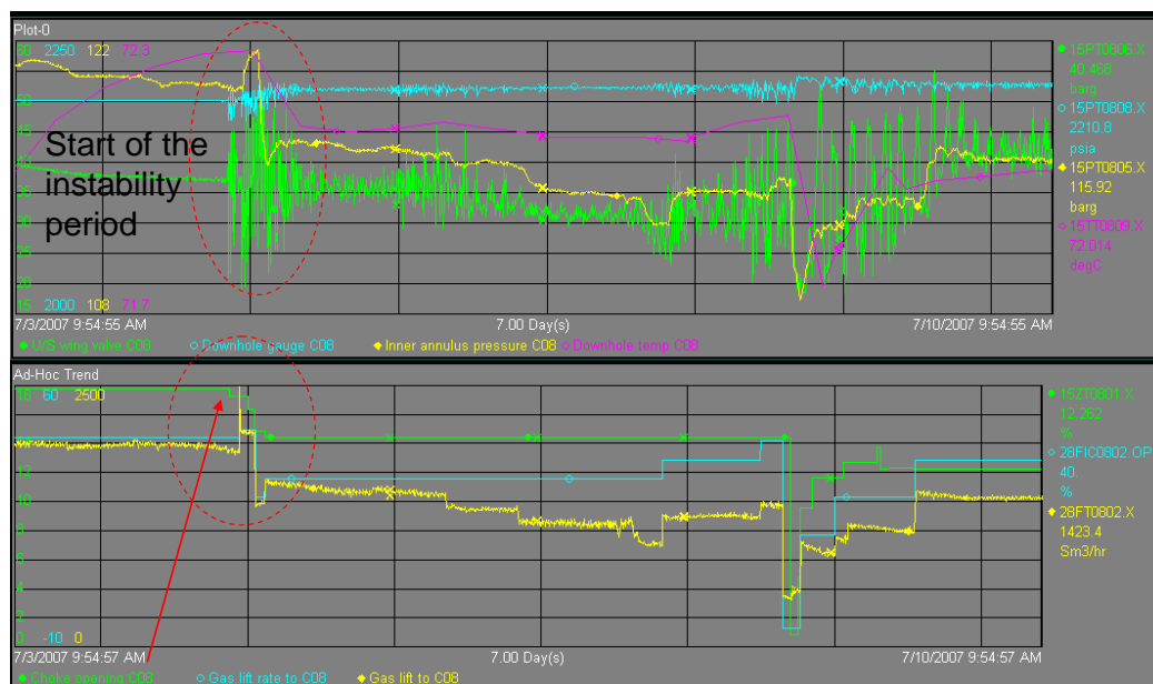
Figure 14 Real-time well slugging recognition
