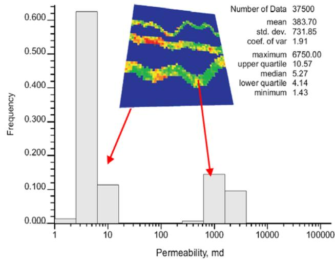
Fig. 4: Permeability distribution for the 5 model realizations [7]
