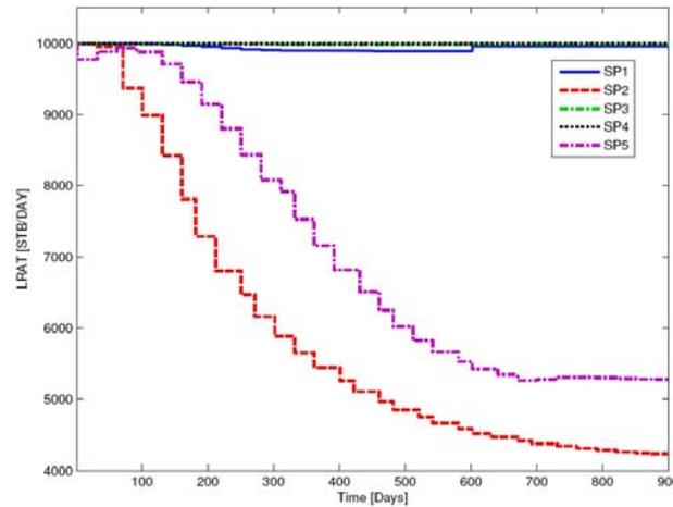
Fig. 8: Optimal liquid production rates
