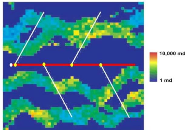
Fig. 3: Fluvial reservoir model [7]
