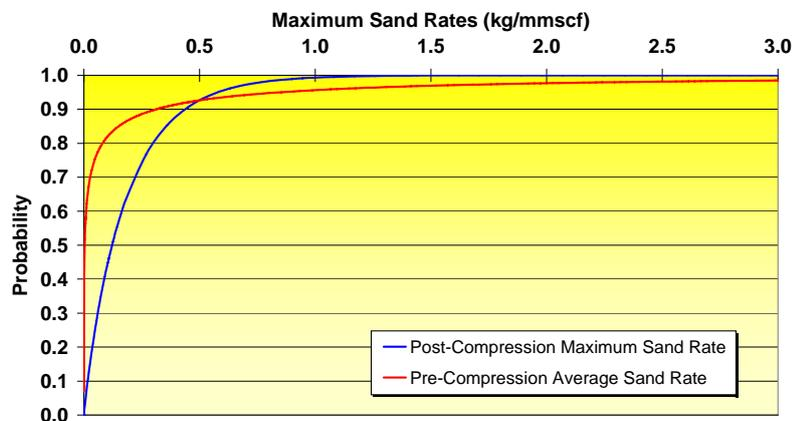
Figure 6. Estimated probability distributions for sand rates pre- and post-compression (2020) based on Lunskeye- 517 predictions for 100% perforated completion.
