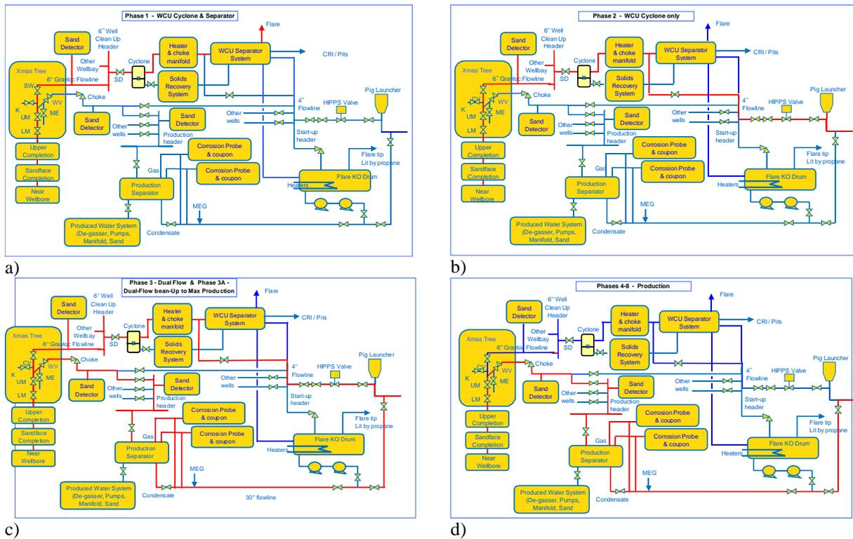
Figure 5. Different phases of production used to identify associated failure modes and assess risks: a) Clean-up, b) Clean-up with cyclone only, c) Bean-up to plateau with dual flow, d) Plateau production.
