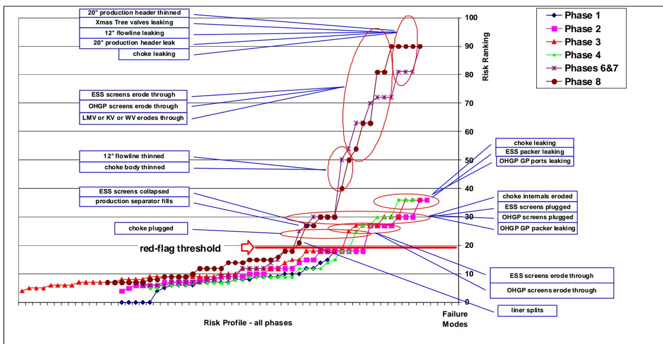
Figure 9. Risk Profile chart illustrating the risk ranked potential failure modes for the Lunskeye big bore gas wells and production system: Base case design and alternative completion scenarios.
