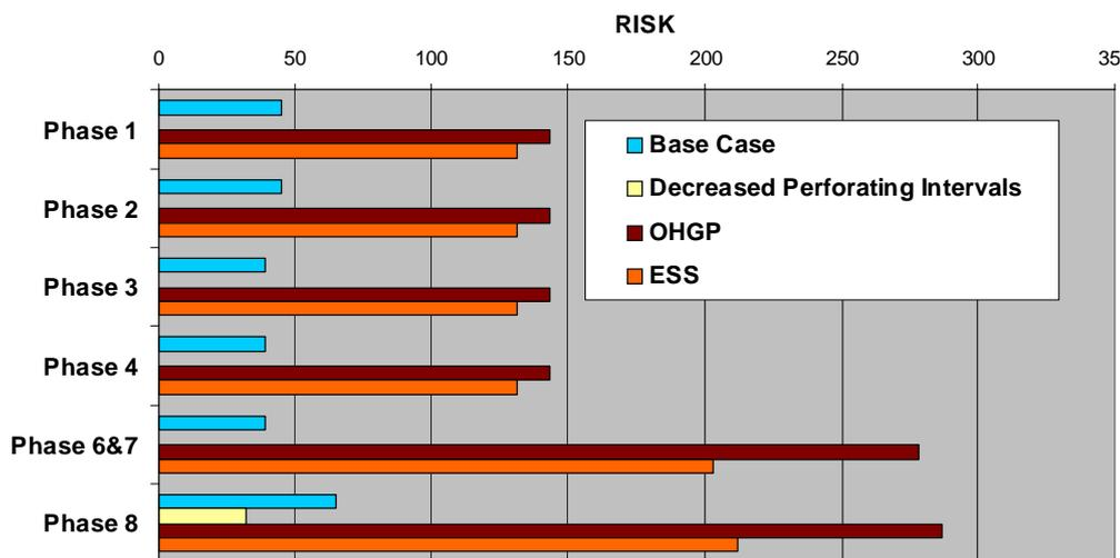
**Figure 10 - Comparison of the risks associated with Alternative Sand-Face Completions**
