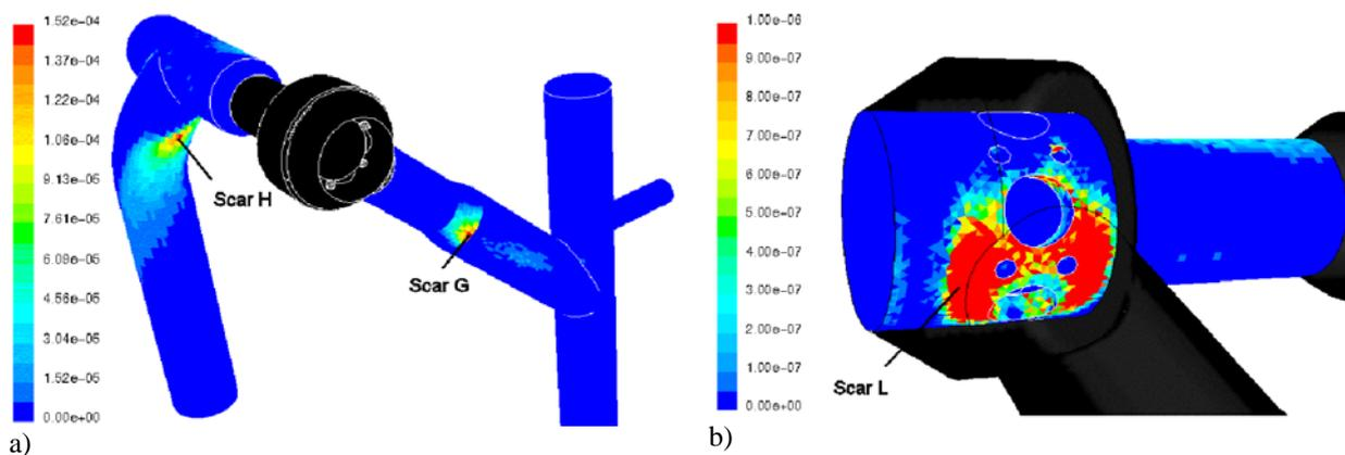
**Figure 8. Erosion rates (mm/kg of  $d_{50}=100 \mu\text{m}$  sand) estimated using Computation Fluids Dynamics modeling of the a) Xmas Tree and 12” flowline, and b) the choke gate for Lunskeye-A big bore gas wells (290MMscf/d) (Barton, 2003).**
