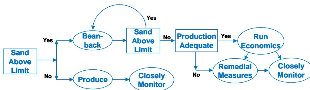
**Figure 11. Generic decision tree in the event of an indication of excessive sand production**
