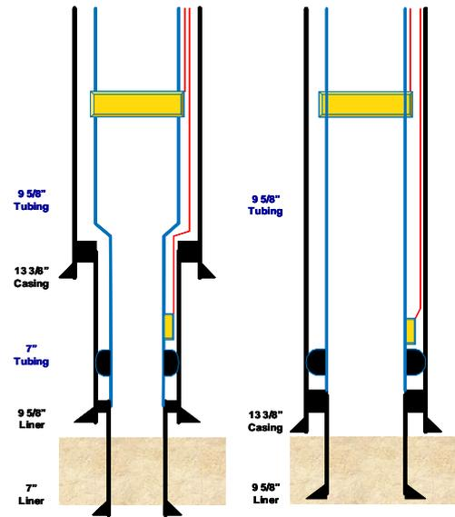
Figure 3. Completion designs for the initial Lunskeye field, big bore gas wells.
