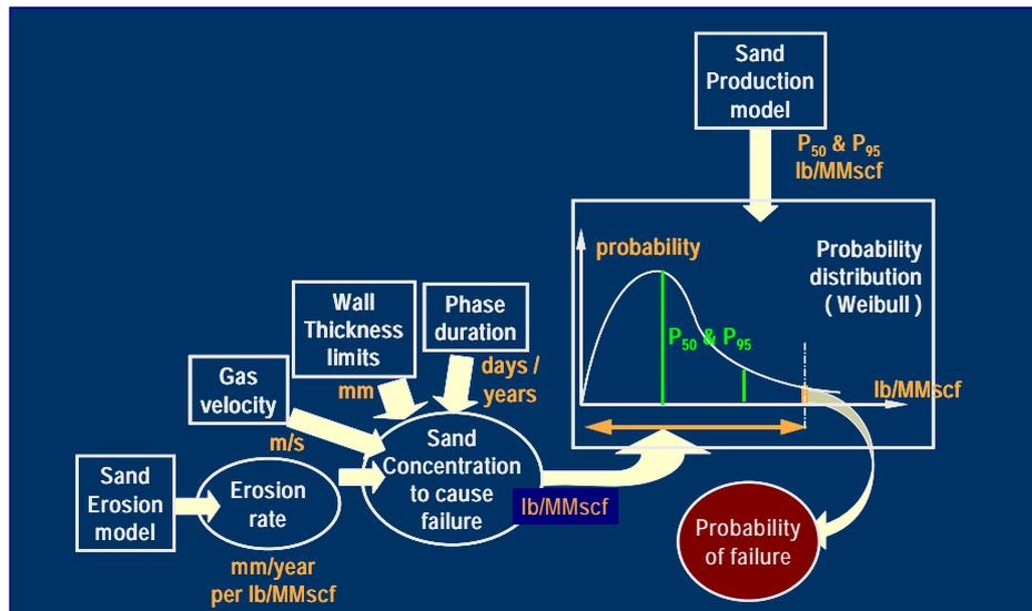
**Figure 7. Estimating Probability of Occurrence of Erosional Failures**
