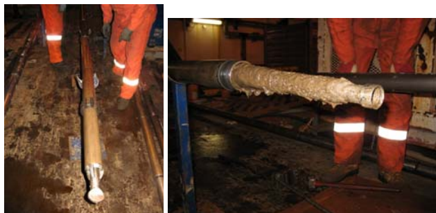
Figure 6a & 6b. Liquid environment cleaner before RIH (left) and debris chamber (bailer) filled with sand after cleaning (right).
