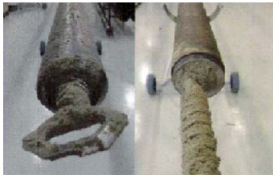
Figure 8. Dry environment cleaner with paddle head and auger (left) used in surface tests. Bailer section filled with sand (right).
