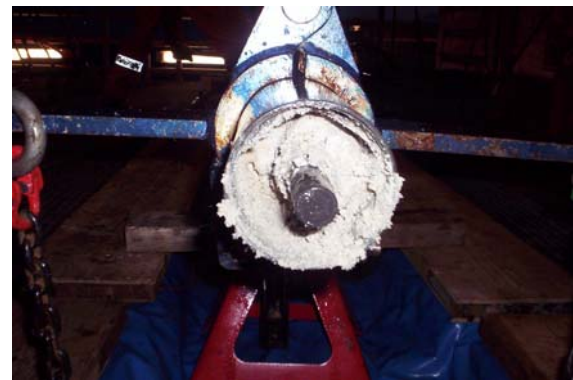
Figure 9. Bailer section filled with Barium Sulphate scale and sand fill from Case History 2.
