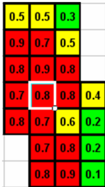
Figure 12: Graphic representation of the probability map p(kh>600 \text{ mDm}) (top view) derived from ten independent realizations of the stochastic geological model. The outlined square corresponds roughly to the geological target for the well, compare Figure 13.
