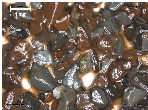
Figure 4: Photographic example from offshore digital microscope: Mixed claystone assemblage; Brick red, fg, claystone, mod Hd, v. slightly calcareous, (caving?); Olive-green black, fg, claystone, soft, non-calc; Rare micas, graphite, lmst (LCM material; Rarely pyritic.
