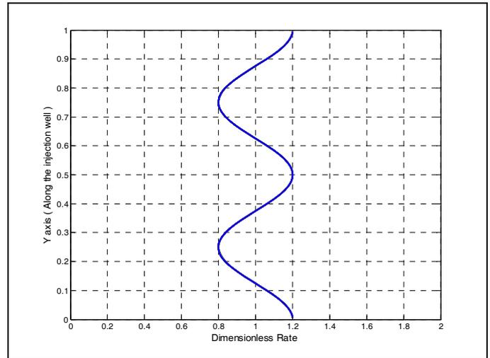
**Figure.6a** Injection rate profile that produces the front location as a function of time specified in Fig. 3a.  $R_L = 0.01$
