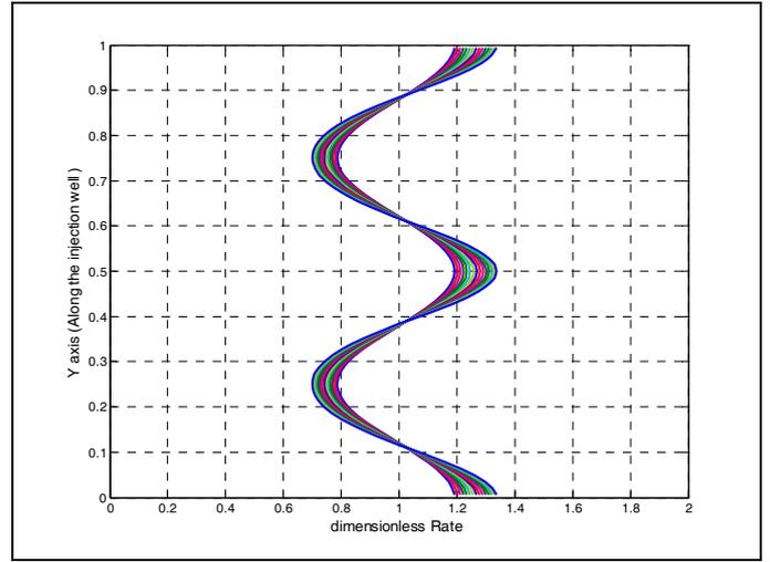
**Figure.5a** Injection rate profile that produces the front location as a function of time specified in Fig. 3a.  $R_L = 0.1$
