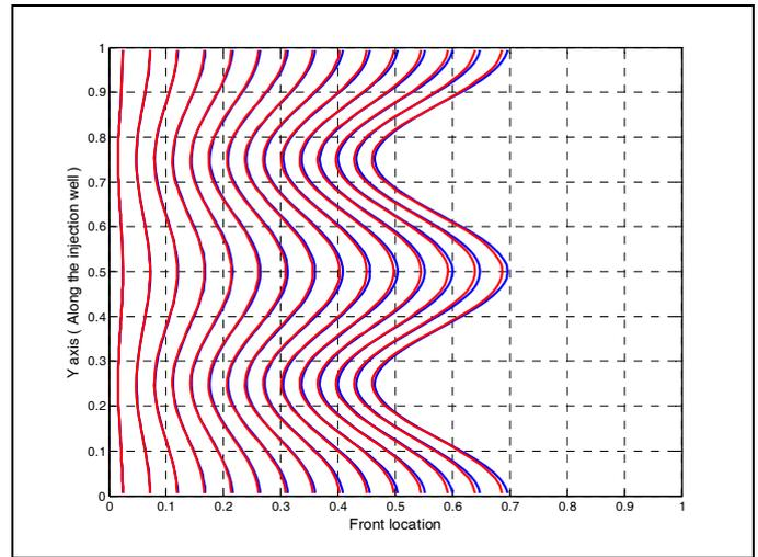
**Figure 5b.** Comparison between desired (blue color) (Fig. 3a) and achieved front dynamics (red color) using the profile of Fig. 5a.  $R_L = 0.1$
