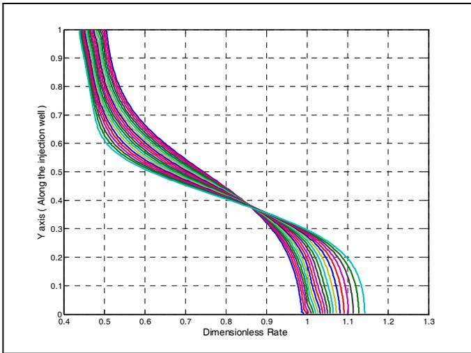
**Figure.4b** Injection rate profile that produces the front location as a function of time specified in Fig. 4a. ( $R_L = 1$ )
