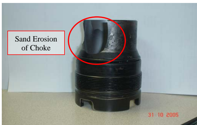
Figure 8 –Eroded choke of MA-12
