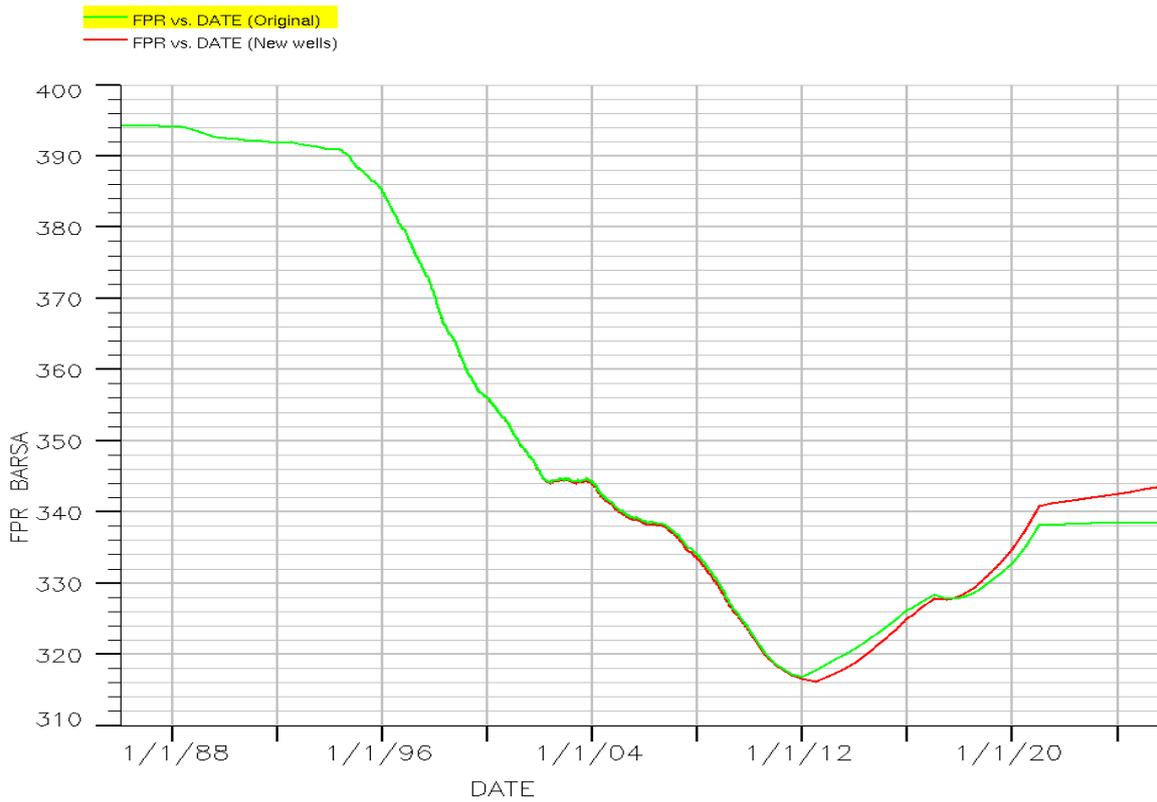
**Figure 2.37: Comparison of reservoir average pressure with and without new wells in faults sealed model**
