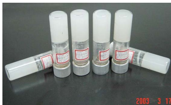
Figure 16 Inorganic gel produced from the reaction of Abio gel and injection brine (130 °C) 7
