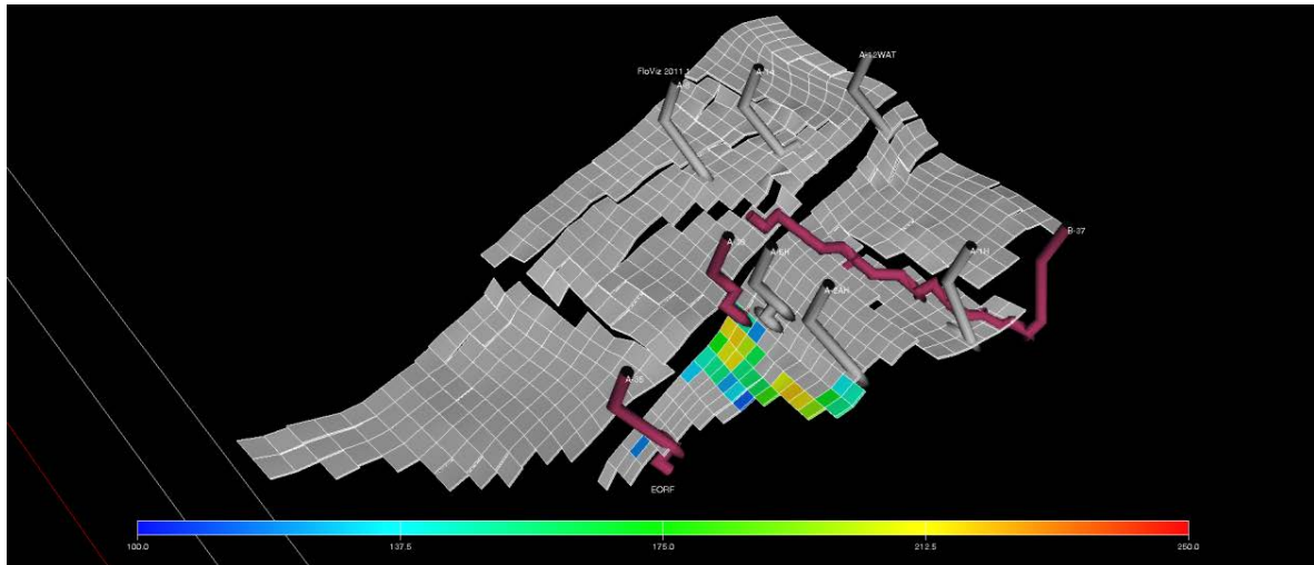
Figure 33 Position of tracer which has concentration between 100 and 250 at timestep January 2013
