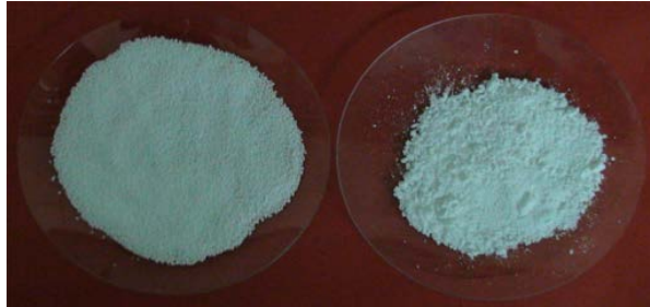
Figure 15 Abio gel powder and particles 7
