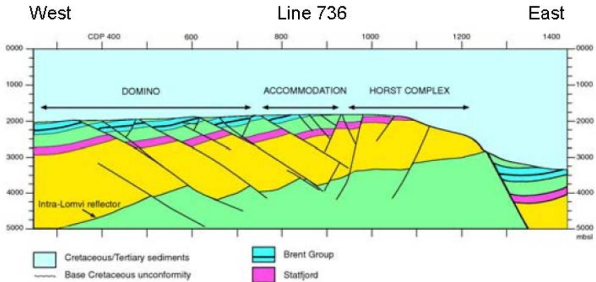
**Figure 1** Structural setting of the Gullfaks main field (Talukdar & Isntefjord, 2008)
