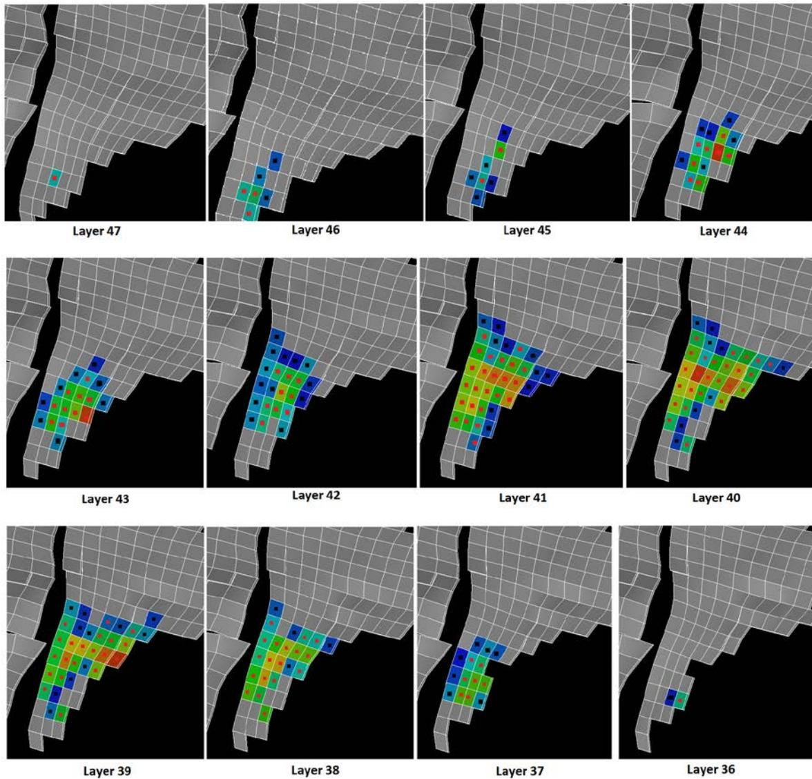
**Figure 18** Tracer concentration distribution for layers 36 to 47 (time step 1. June 2012) for case with lowered threshold value
