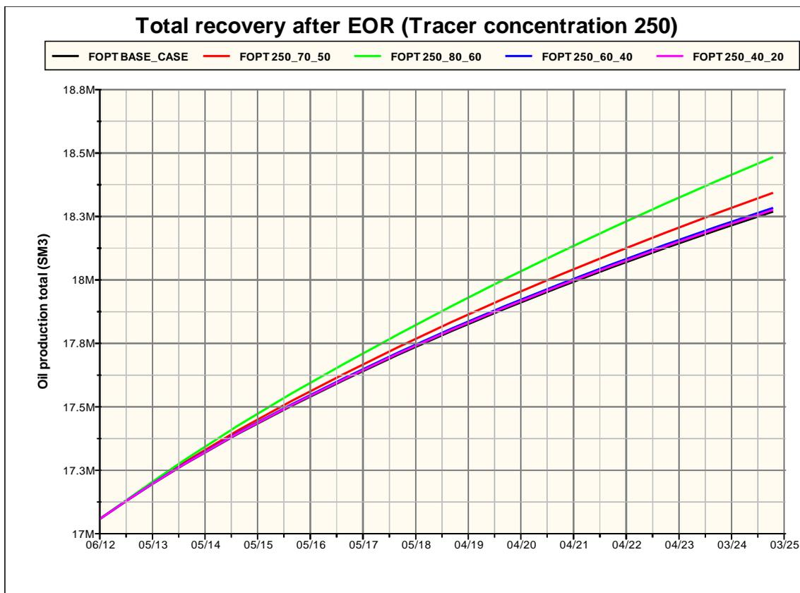
**Figure 8** Total recovery of oil after EOR, with Tracer concentration of 250 from 2012 to 2025
