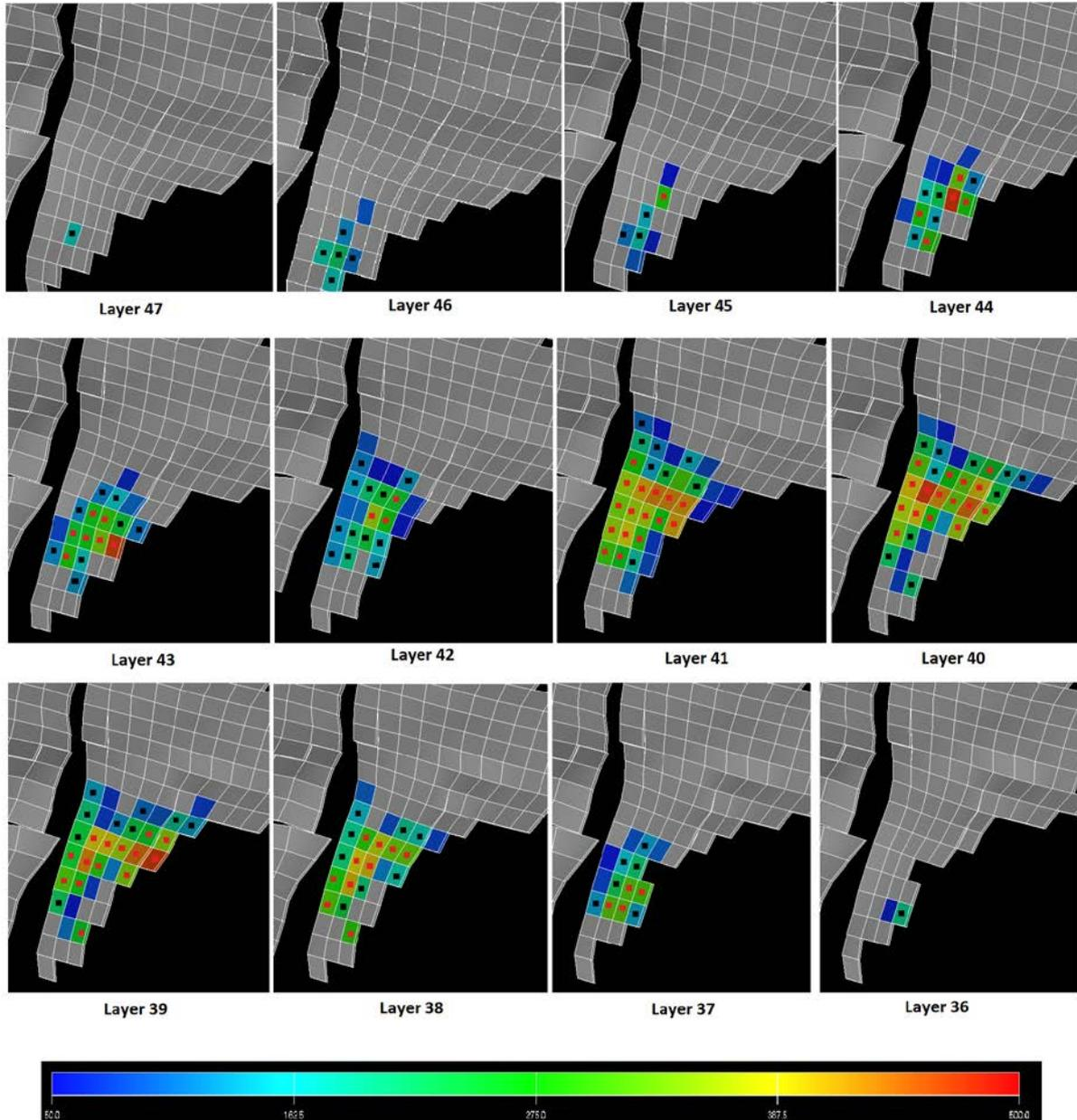
**Figure 17** Tracer concentration distribution for layers 36 to 47 (time step 1. June 2012)
