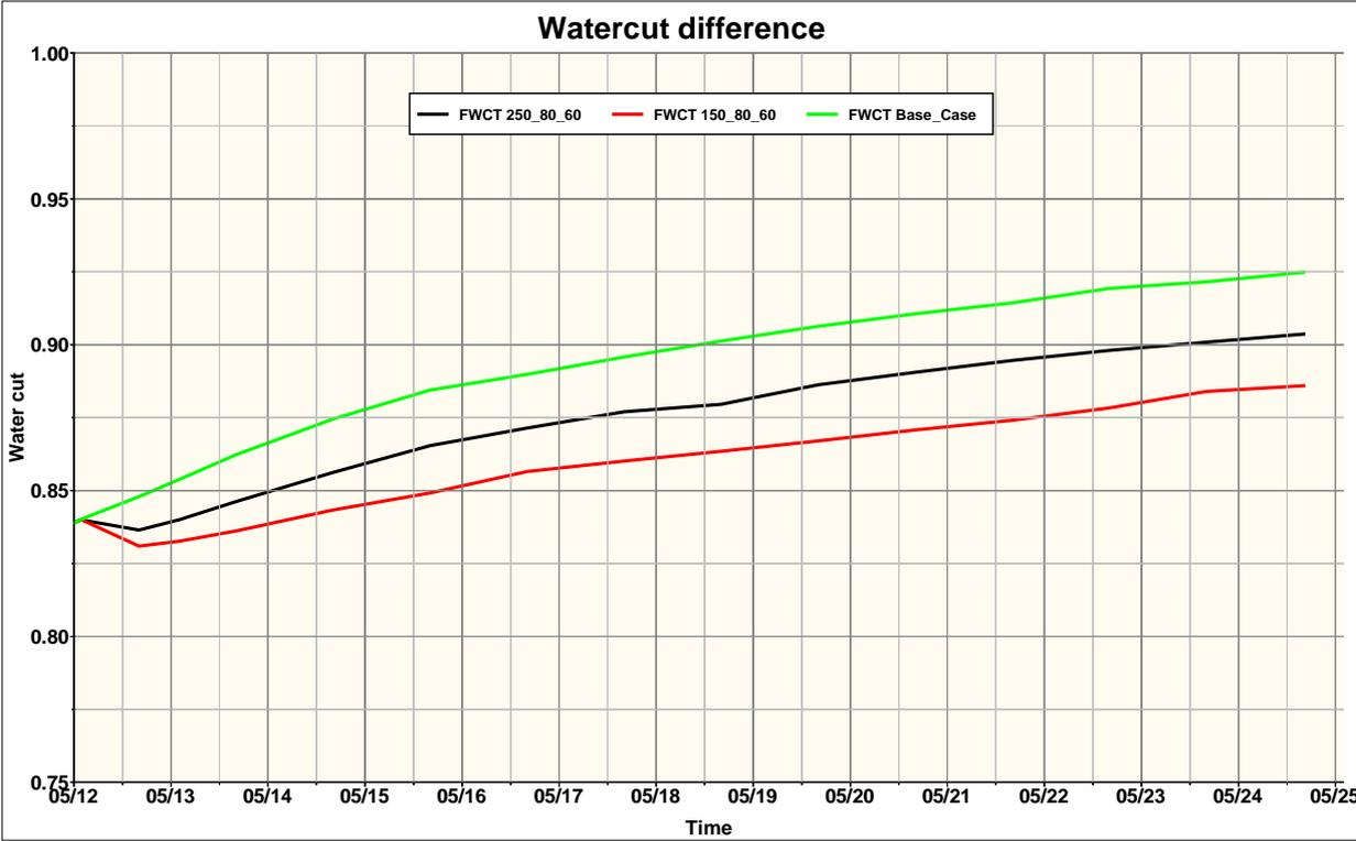
**Figure 9** Water cut in 80%-60% permeability reduction with tracer concentration of 150 and 250 compared to Base Case from 2012 to 2025
