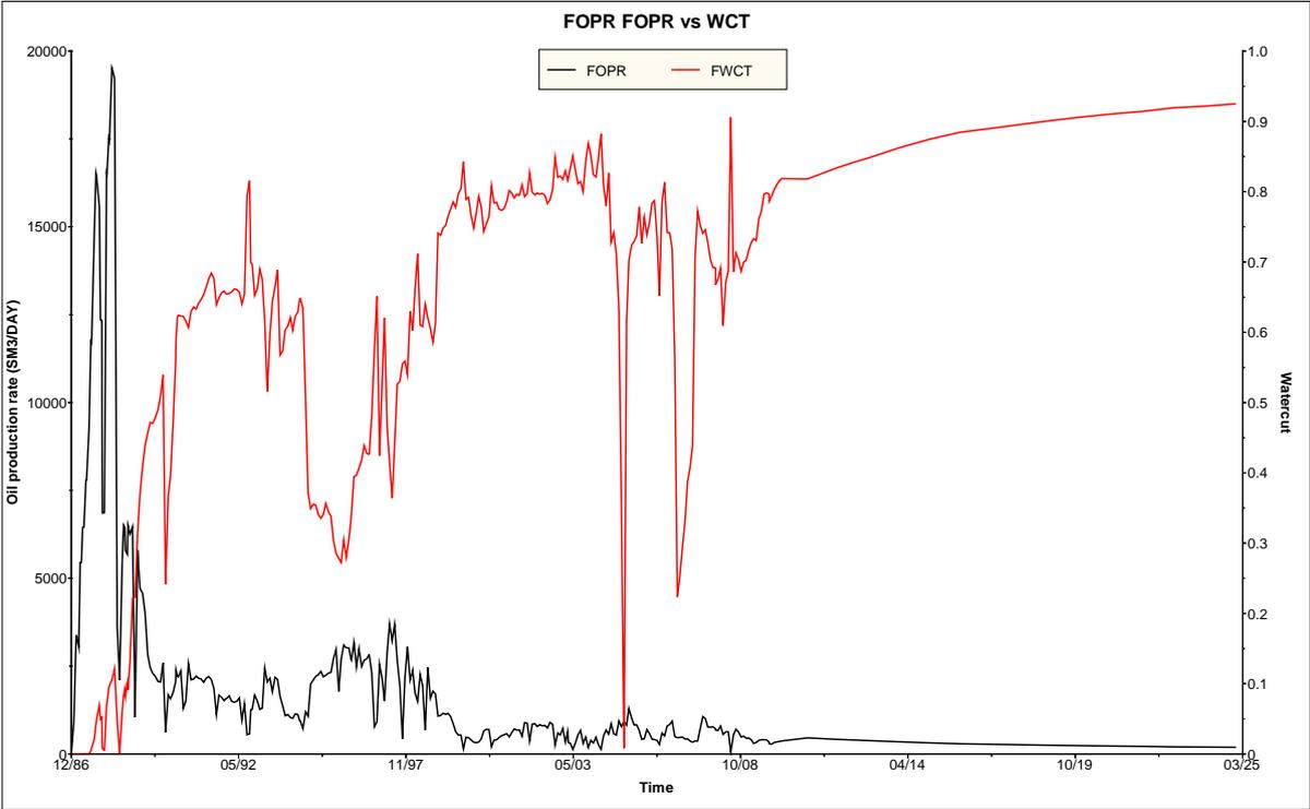
Figure 6 Base case simulation of water cut and oil production
