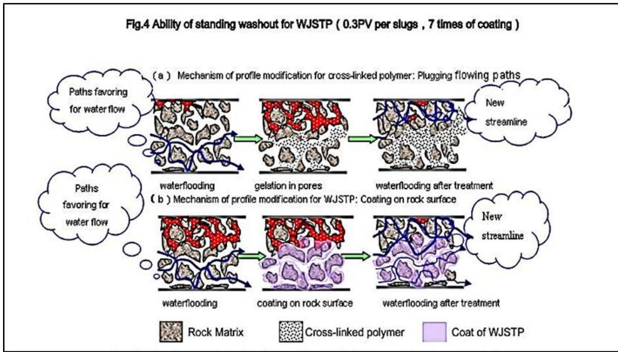
**Figure 20** Different mechanism of profile modification for inorganic gel and cross-linked polymer Sensitivity Analysis of the Project
