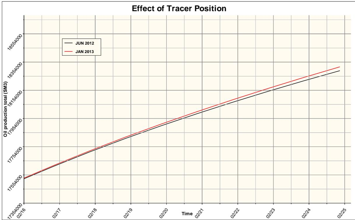
**Figure 11** The effect of position of tracer on total oil production from 2016 to 2025
