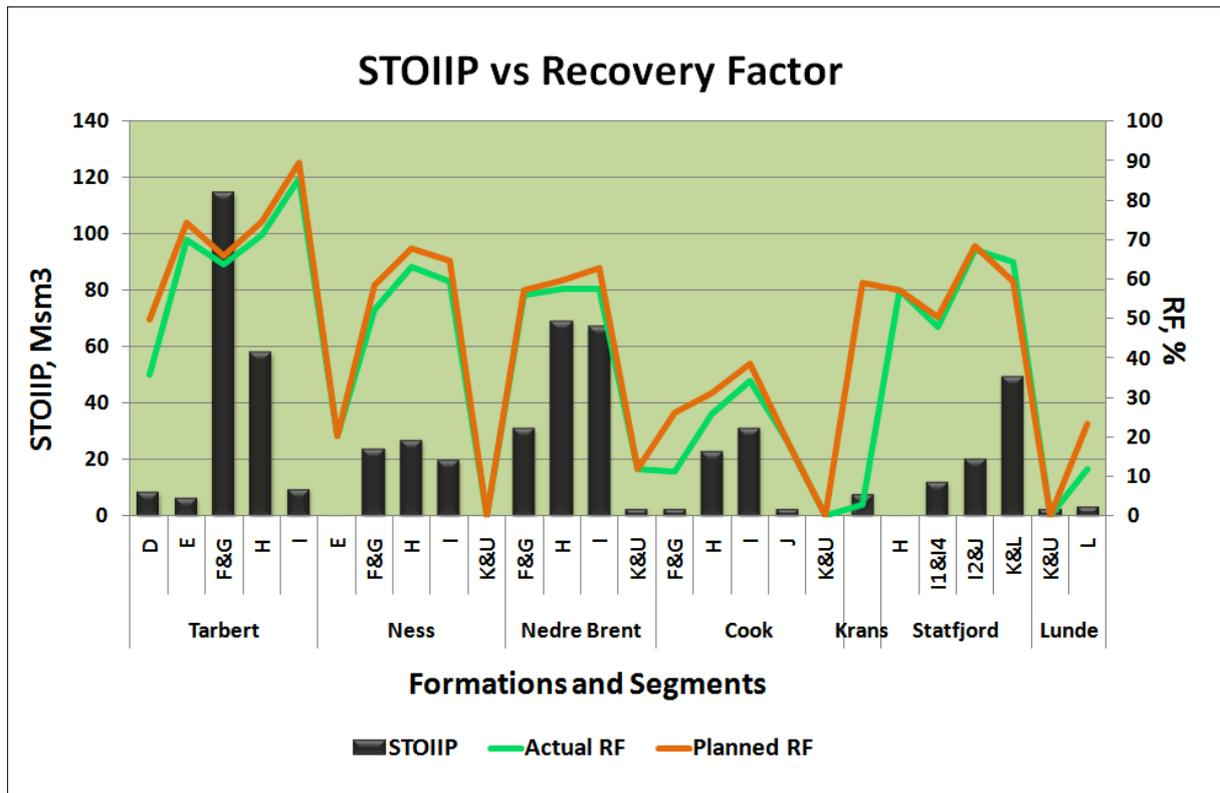
**Figure 4** STOIIP vs Actual and Planned recovery factor in the different segments at the Gullfaks main field (Statoil, 2008)
