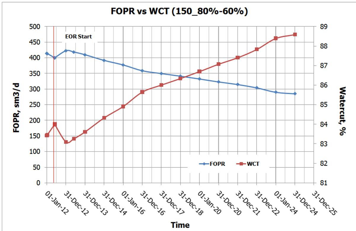
**Figure 12** Field oil production rate (sm<sup>3</sup>/day) vs. Water cut (%) with a concentration of 150 and 80-60% permeability reduction, 01 January 2012-31 December 2025
