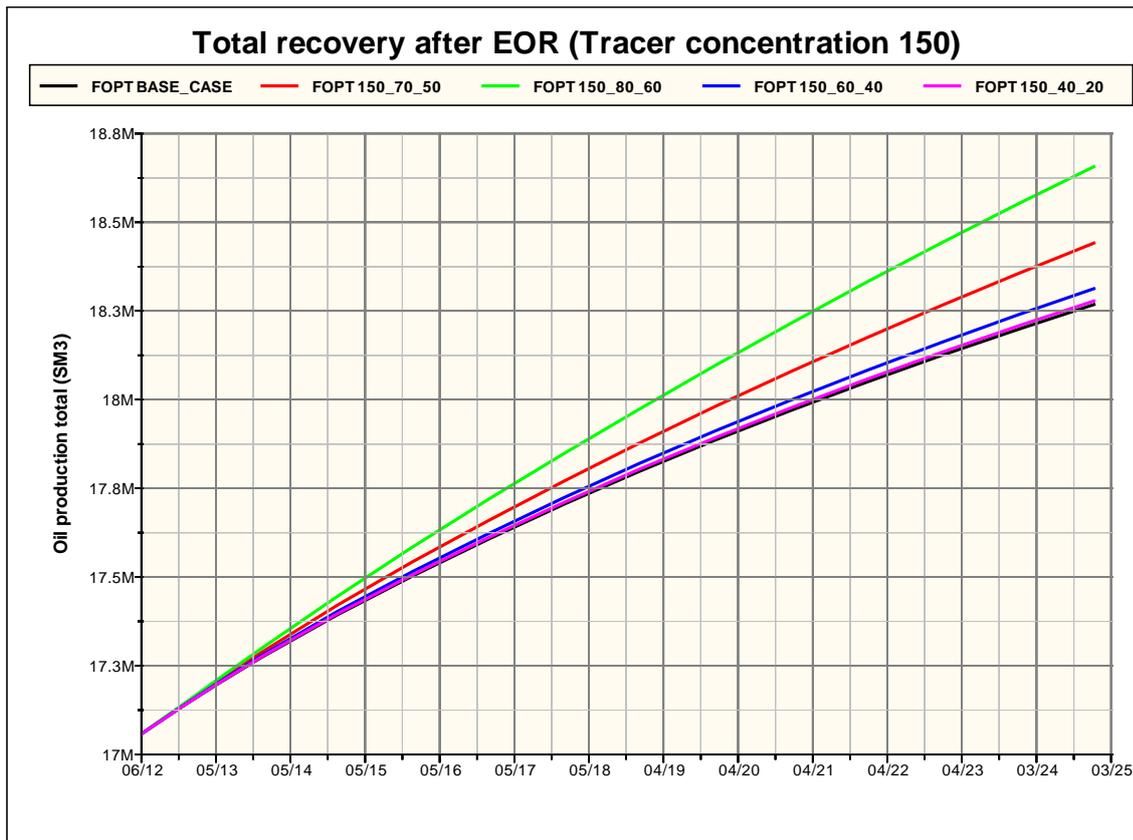
**Figure 7** Total recovery of oil after EOR, with Tracer concentration of 150 from 2012 to 2025
