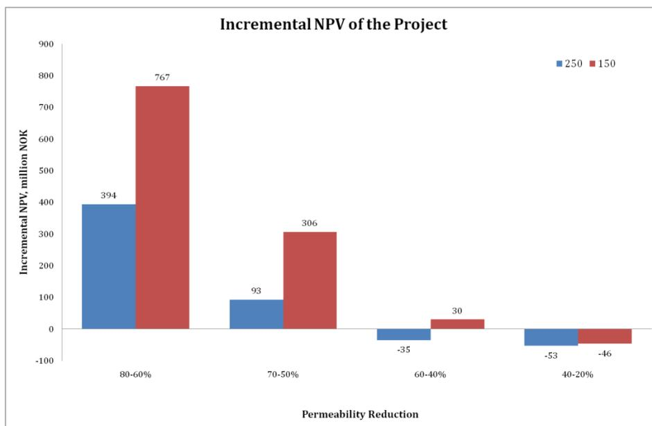
**Figure 13** Incremental NPV of the Project at various permeability reductions and tracer concentrations
