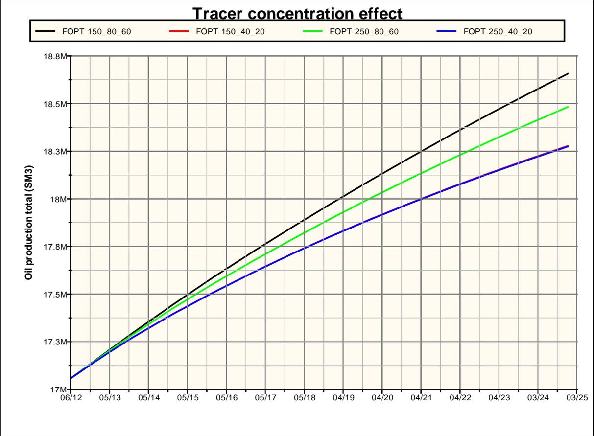
**Figure 10** The effect of choosing different tracer concentration on total oil production from 2012 to 2025.
