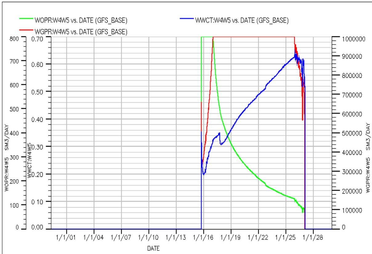
Figure 19: Well Oil Production Rate, Well Gas Production Rate and Well Water Cut for well W4W5.
