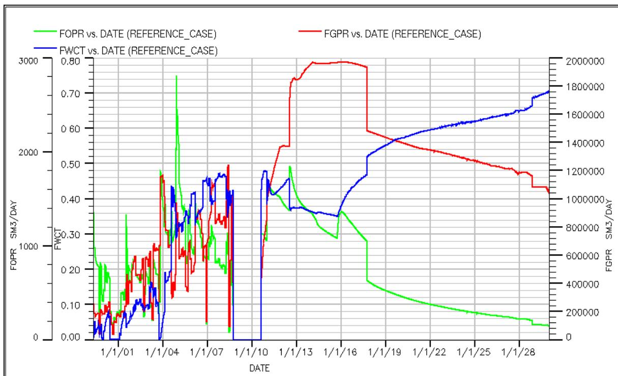
Figure 10: Field Oil Production Rate, Field Gas Production Rate and Field Water Cut.
