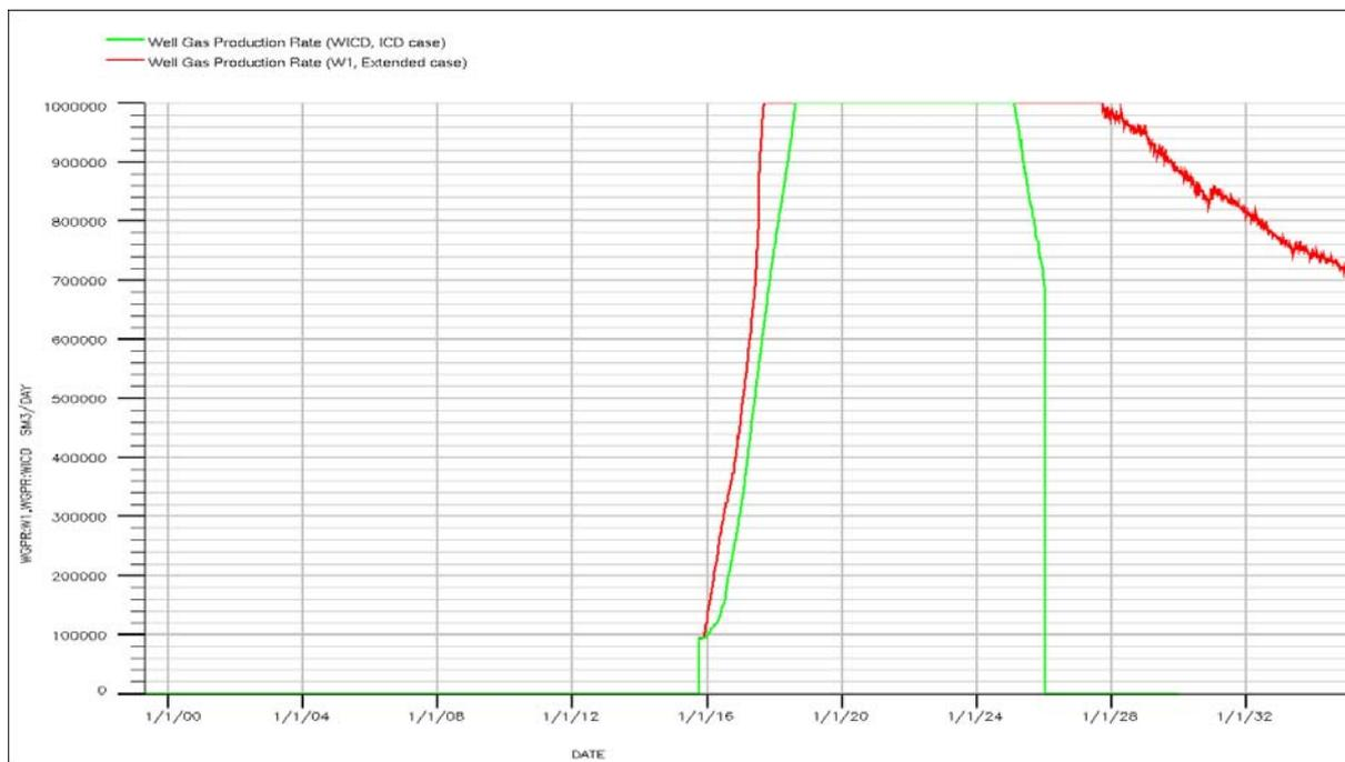
**Figure 49: Well Gas Production Rate of wells WICD and W1.**
