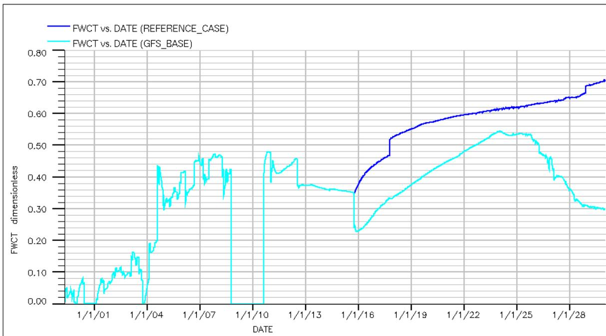
Figure 26: Field Water Cut for the Reference Case and the Extended Case.
