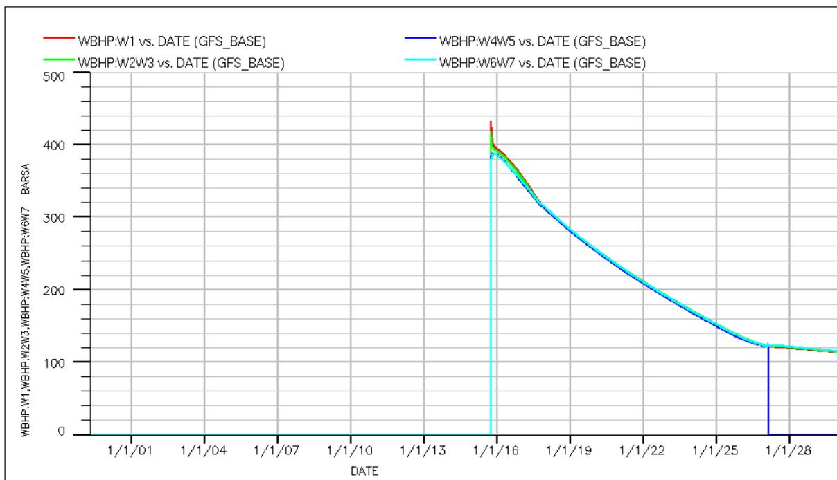
Figure 16: Well Bottom Hole Pressure W1, W2W3, W4W5 and W6W7.
