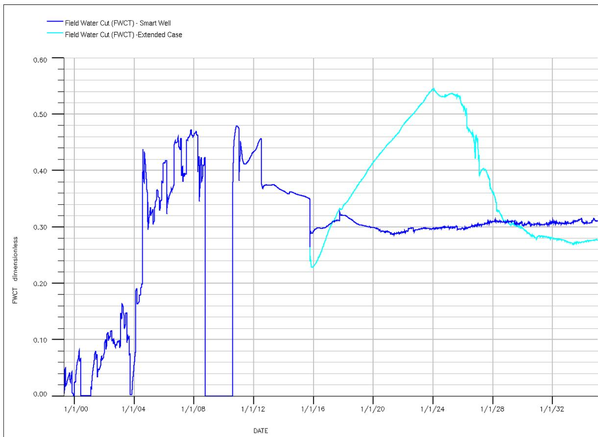
Figure 45: Field Water CuT for Smart Well case and Extended Case.
