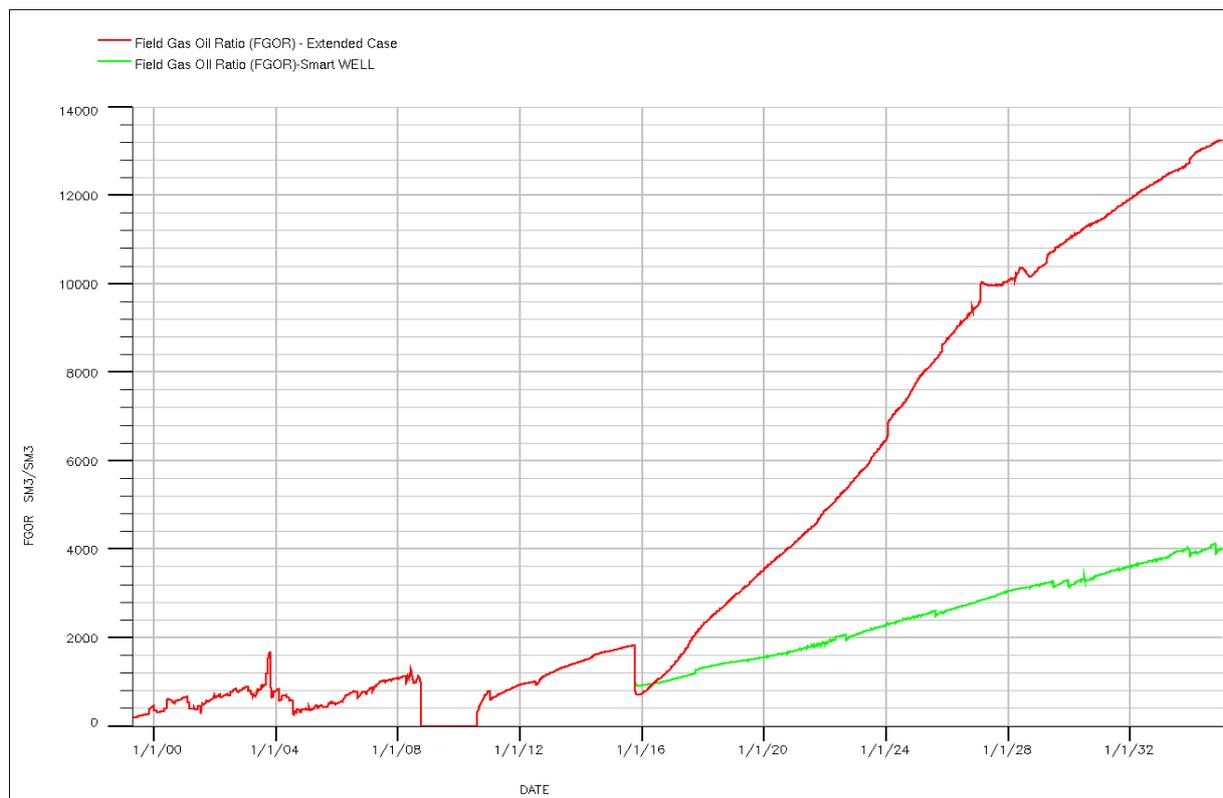
**Figure 43: Field Gas-Oil Ratio for Smart Well case and Extended Case.**
