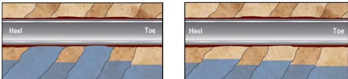
**Figure 37: Heterogenous reservoir. Left: Early water/gas breakthrough without ICD. Right: No early water/gas breakthrough with ICD (Halliburton).**
