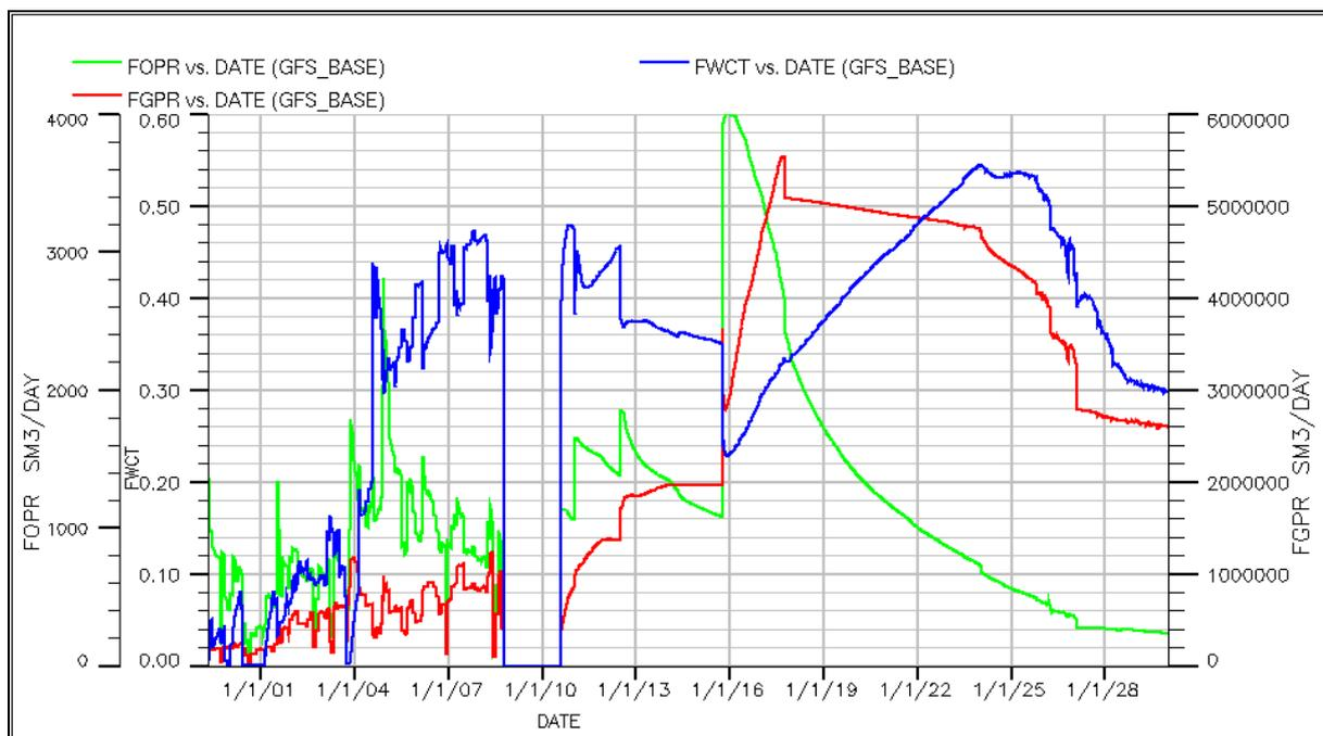
Figure 11: Field Oil Production Rate, Field Gas Production Rate and Field Water Cut.
