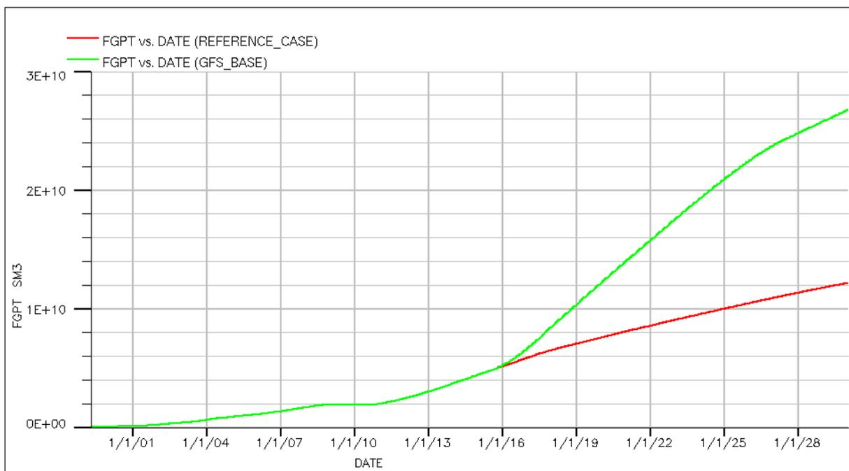
Figure 24: Field Gas Production Total for the Reference Case and the Extended Case.
