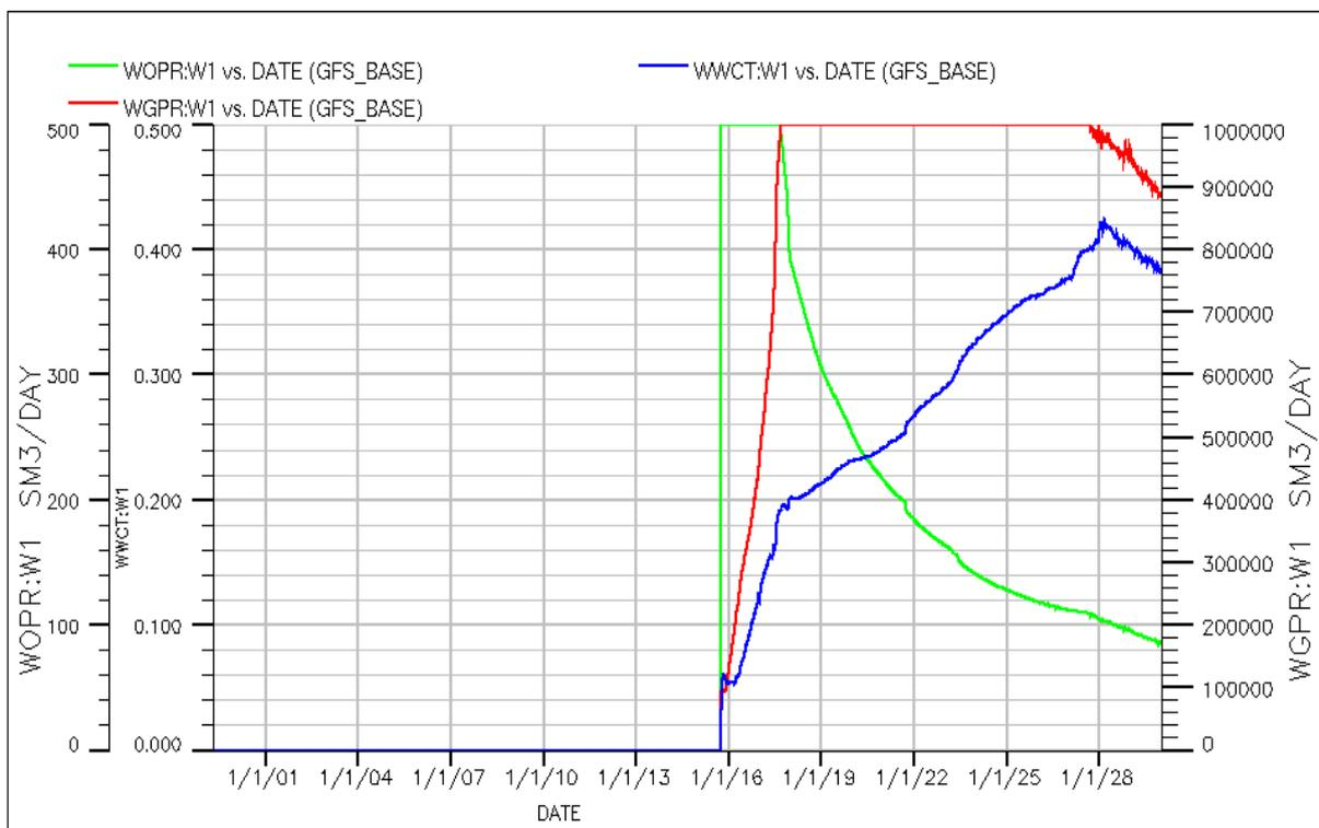
**Figure 17: Well Oil Production Rate, Well Gas Production Rate and Well Water Cut for well W1.**
