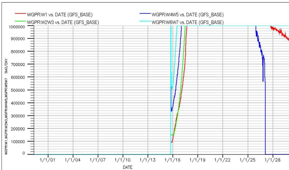
**Figure 13: Well Gas Production Rates W1, W2W3, W4W5 and W6W7.**
