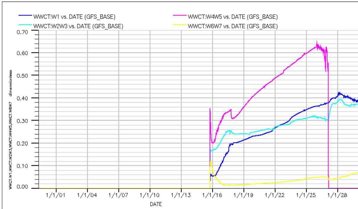
Figure 15: Well Water Cut W1,W2W3, W4W5 and W6W7.
