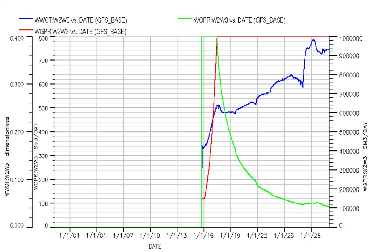
**Figure 18: Well Oil Production Rate, Well Gas Production Rate and Well Water Cut for well W2W3.**
