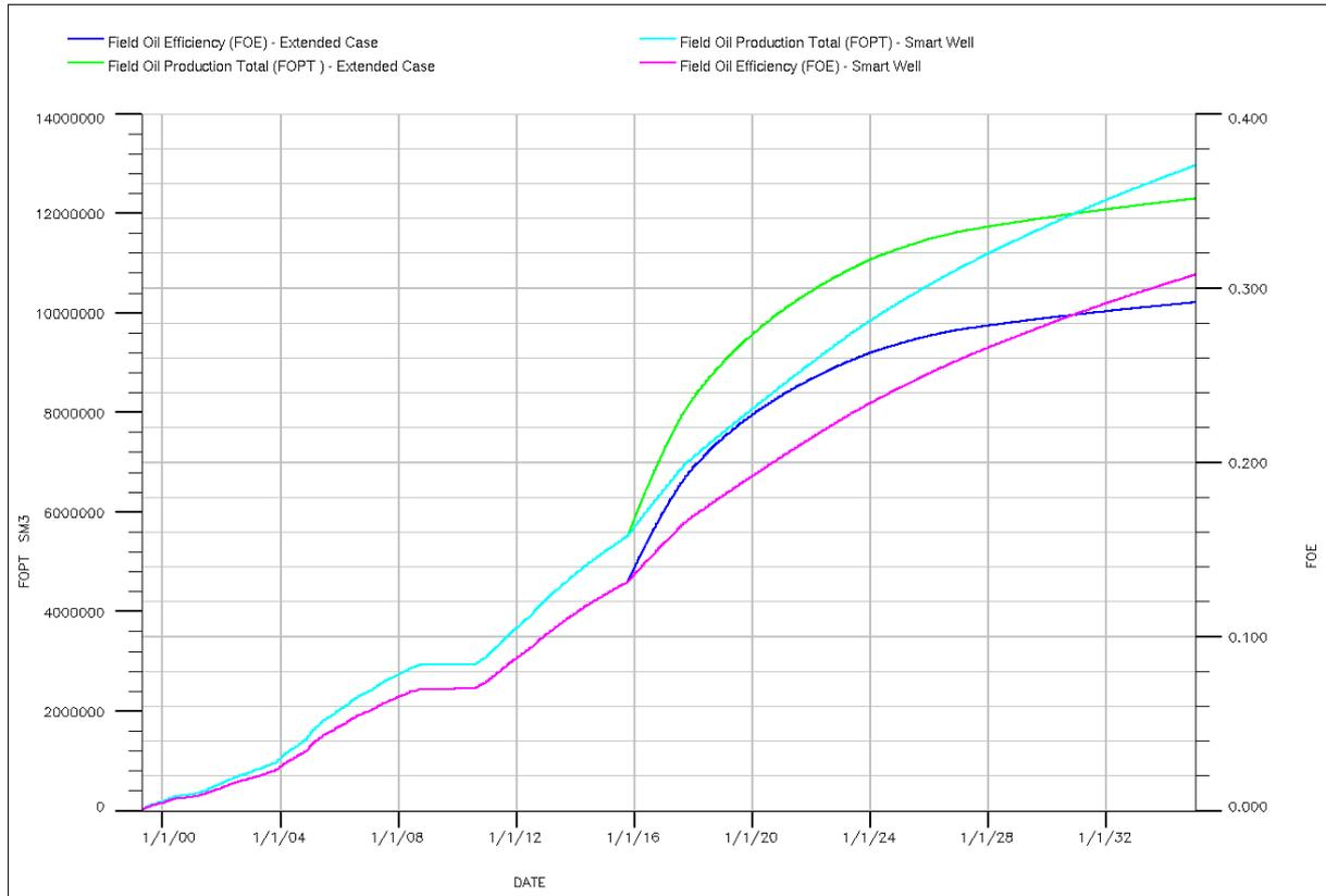
**Figure 47: Field Oil Production Total and Field Oil Efficiency for Smart Well case and Extended Case.**
