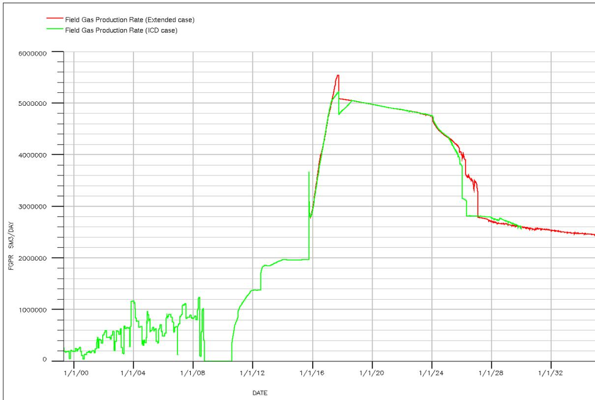
Figure 53: Field Gas Production Rate of ICD case and extended case.
