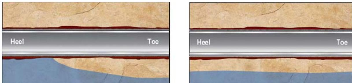
**Figure 36: Homogenous reservoir. Left: Early water and/or gas breakthrough in the heel may occur without ICD. Right: No early water/gas breakthrough with ICD (Halliburton).**
