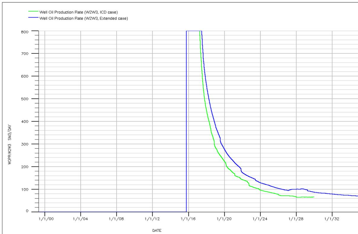
**Figure 56: Well Oil Production Rate of well W2W3 in the ICD case and the extended case.**
