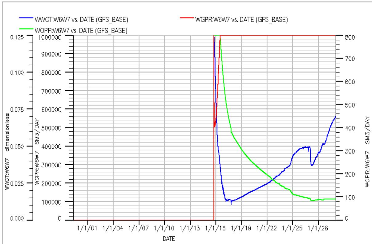
Figure 20: Well Oil Production Rate, Well Gas Production Rate and Well Water Cut for well W6W7.
