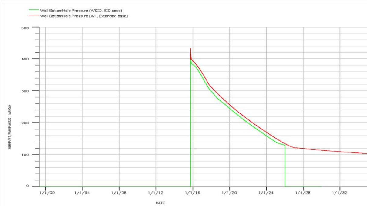
Figure 51: Well Bottom Hole Pressure of wells WICD and W1.
