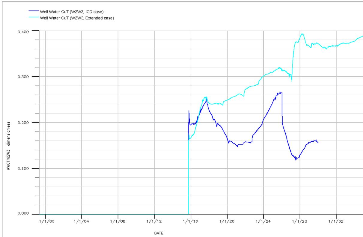
Figure 58: Well Water CuT of well W2W3 in the ICD case and the Extended case.
