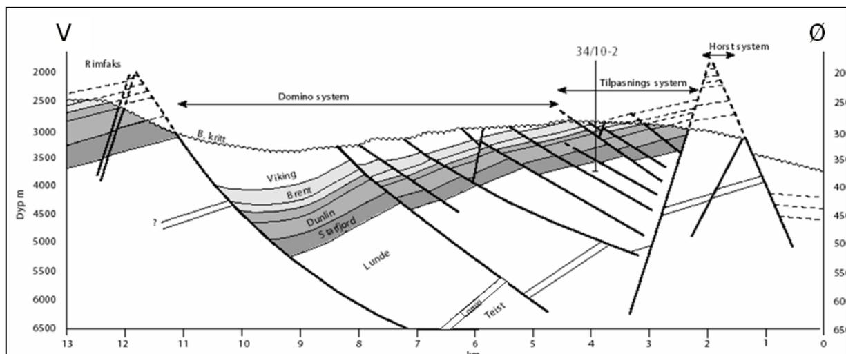
Figure 3: General cross-section of Gullfaks South (Statoil, 2007).
