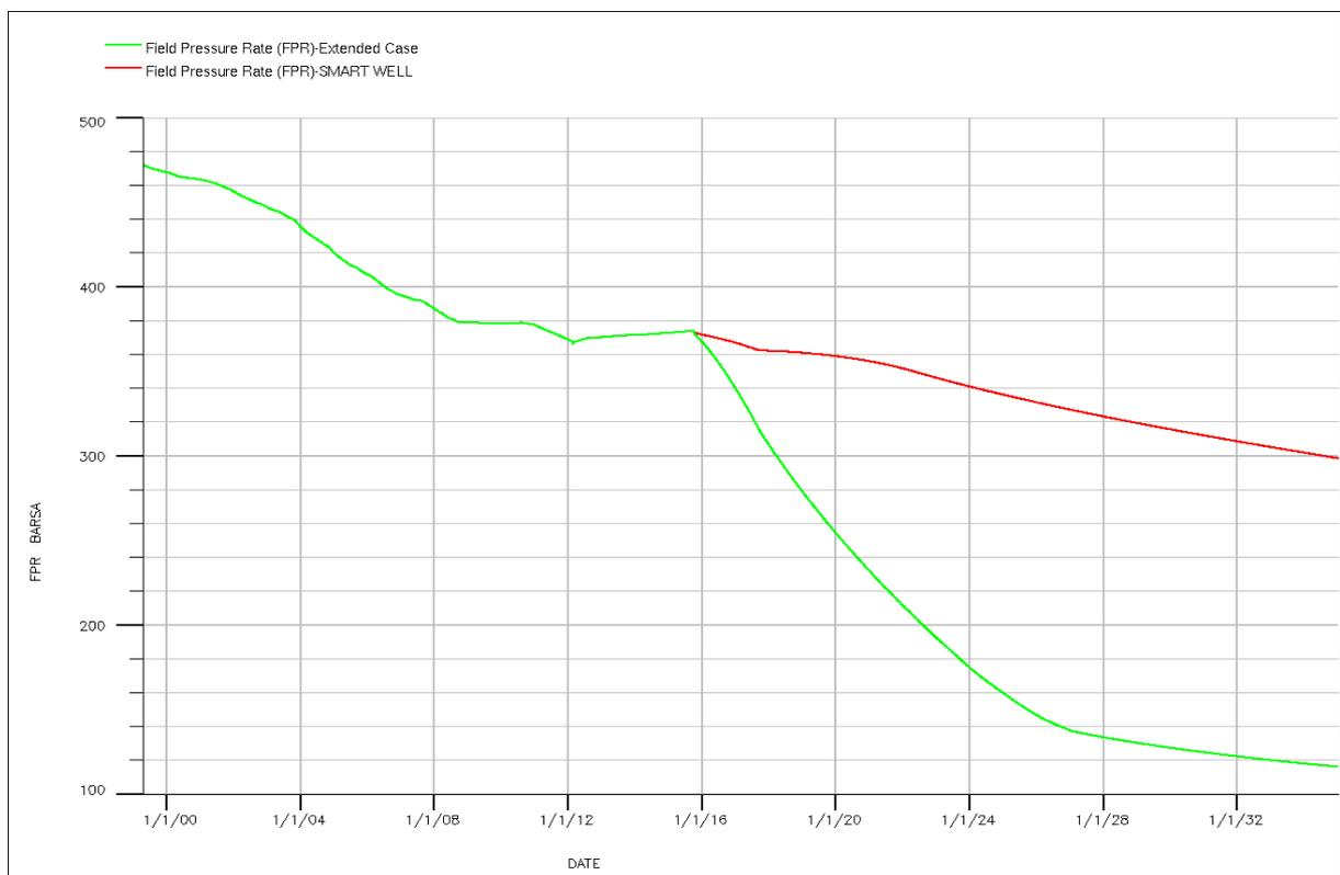
Figure 42: Field Pressure Rate for Smart Well case and Extended Case.
