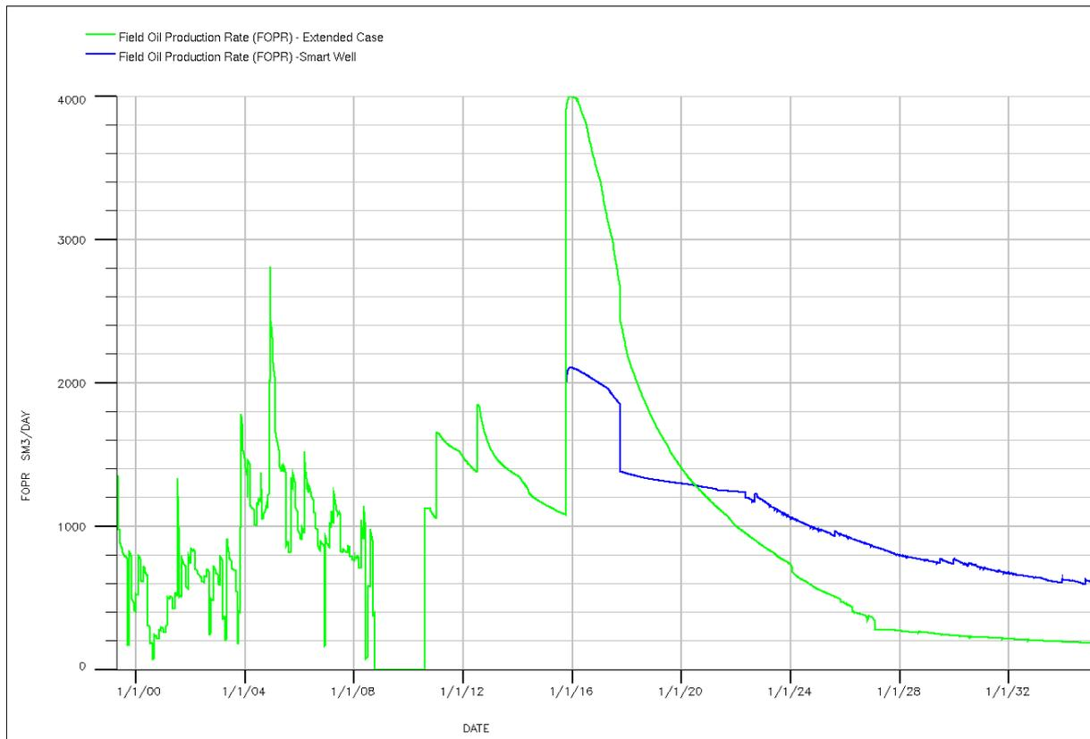
**Figure 46: Field Oil Production Rate for Smart Well case and Extended Case.**
