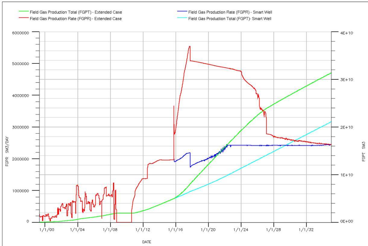
Figure 44: Field Gas Production Total and Field Gas Production Rate for Smart Well case and Extended Case.
