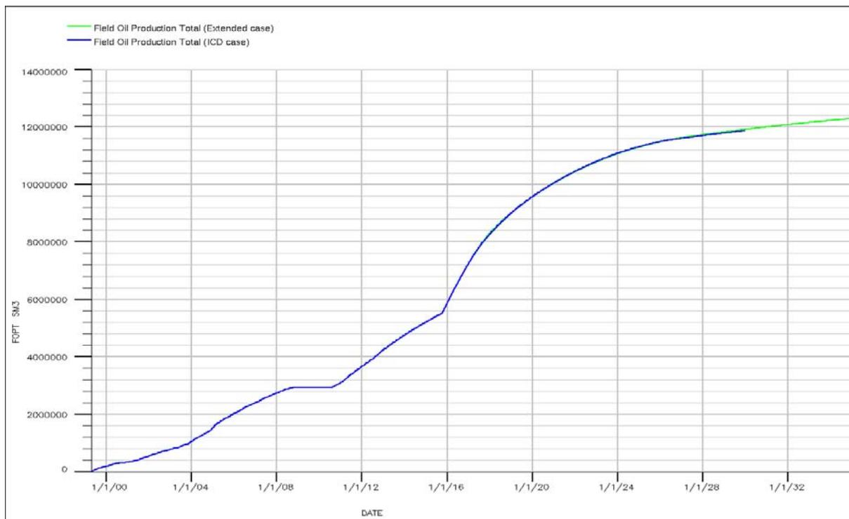
**Figure 55: Field Oil Production Total of ICD case and extended case.**
