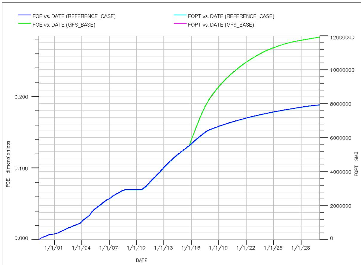
Figure 22: Field Oil Production Total for Reference Case and the Extended Case.
