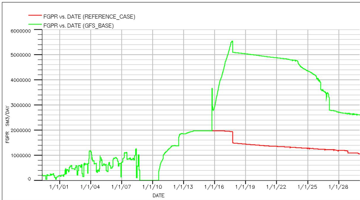
Figure 23: Field Gas Production Rate for the Reference Case and the Extended Case.
