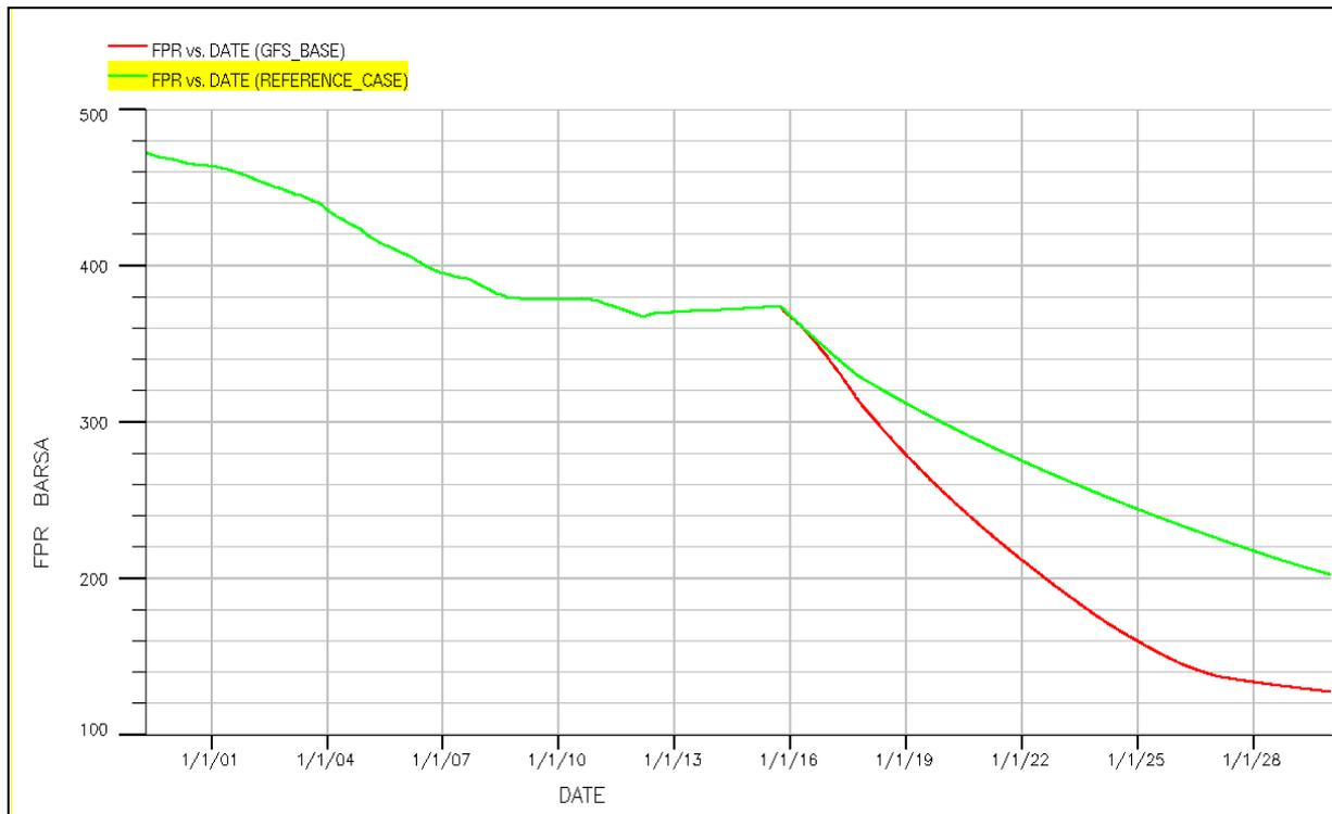
Figure 27: Field Pressure Rate for the Reference Case and the Extended Case.
