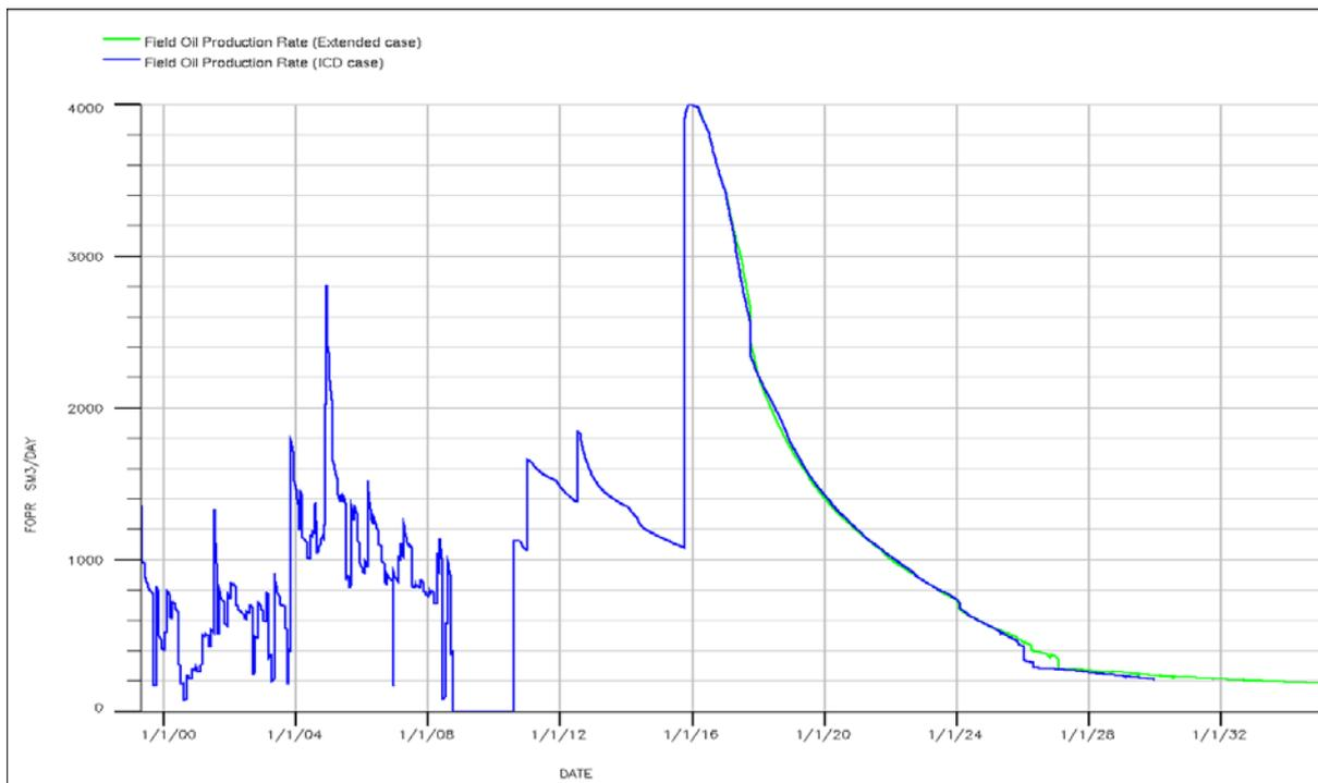
Figure 52: Field Oil Production Total of ICD case and extended case.
