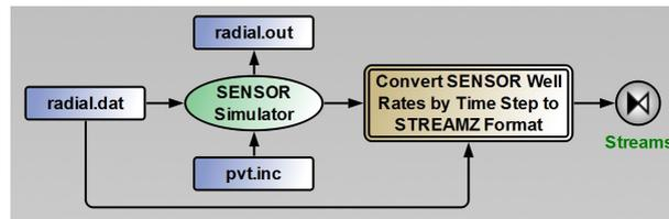
**Fig. 3.10:** Reservoir Simulator composite which launches SENSOR reservoir simulation and converts SENSOR output into *Streamz* format compatible with Pipe-It.
