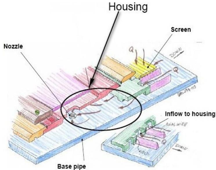
**Fig. 2.6:** Schematic of the elements included in the nozzle-based ICD [Moen 2005].
