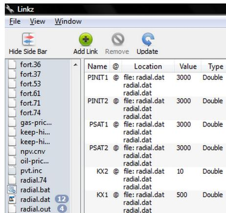
**Fig. 3.4:** Image of *Linkz* feature (included in Pipe-It) which enables users to locate variables inside files and update them automatically.
