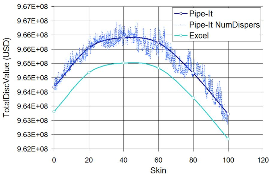
(b) Total Discounted Value versus skin revealing numerical dispersion due to SENSOR implicit calculations.
