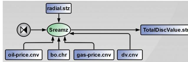
(b) Organization of Streamz Calculations composite. All Streamz executions are brought together inside one process called *Streamz*.
