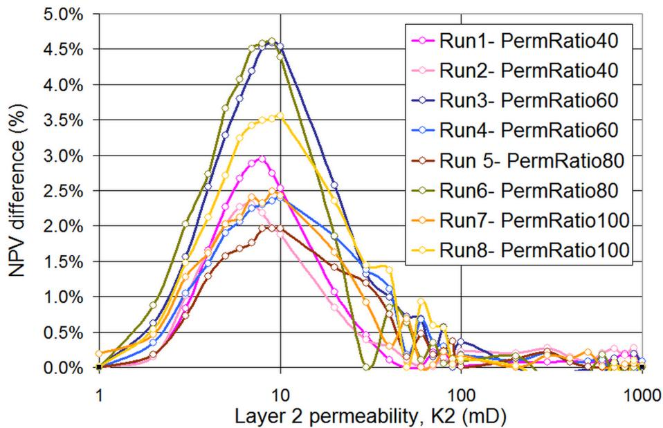
**Fig. 4.8:** Total Discounted Value increase versus *Layer 2* permeability. This plot is obtained using height different reservoirs (height Master cases). *Layer 2* permeability vary between 1 mD and 1000 mD (on a log scale) while permeability ratio  $\frac{K_1}{K_2}$  is maintained constant and equal to 40. Results show that not only permeability ratio counts but values of permeabilities have also a significant importance.
