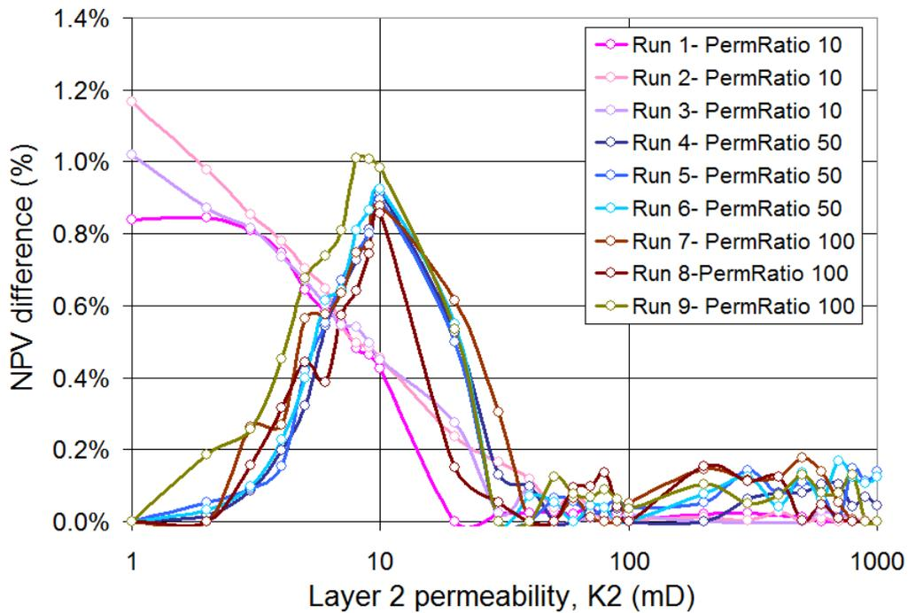
**Fig. 4.9:** Total Discounted Value increase versus *Layer 2* permeability. This plot is obtained using nine different reservoirs (nine Master cases after last filtering constraint introduction). *Layer 2* permeability varies between 1 mD and 1000 mD (on a log scale) while permeability ratio  $\frac{K_1}{K_2}$  is maintained constant for each run. Results show that not only permeability ratio counts but values of permeabilities have also a significant importance.
