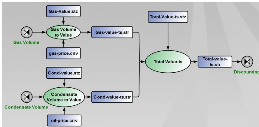
**Fig. 3.13:** First sub-composite, Value Calculation. Based on price assumptions for oil and gas, it returns a total value (not discounted) per time step called "Total-value-ts.str".
