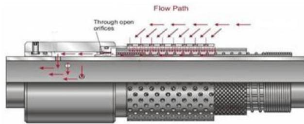
**Fig. 2.7:** ICD based on orifice concept. Orifices perforated on ICD chamber provide required pressure drop [Alkhelaiwi 2007].
