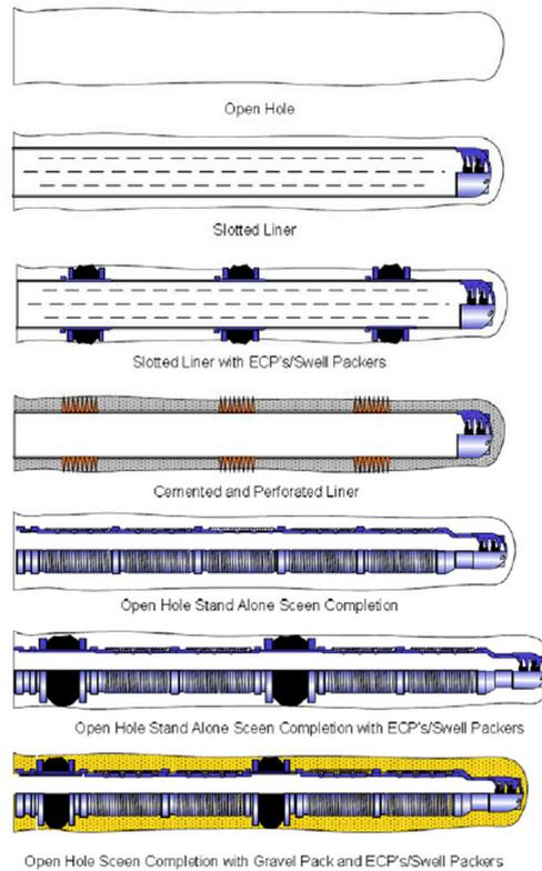
**Fig. 2.1:** Different Open Hole completion options. ICD is generally associated with sand screens and packers.
