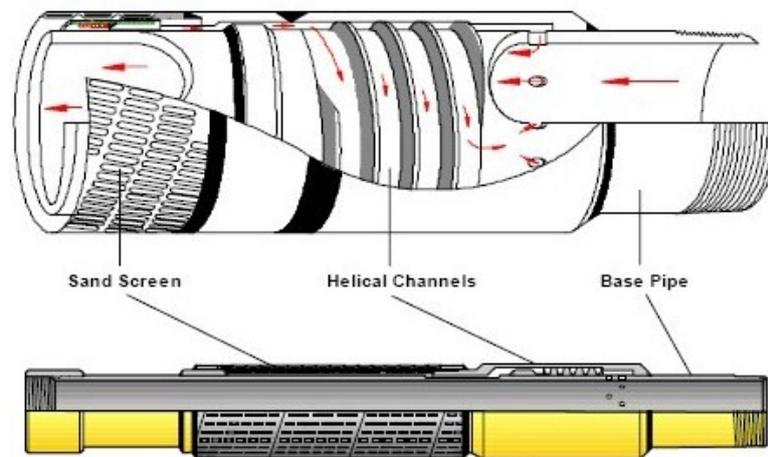
**Fig. 2.4:** ICD based on channel concept. Helical channels provide required pressure drop [Qudaihy 2003].
