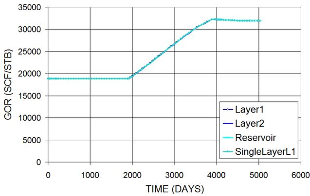
(c) Production Gas Oil Ratio from different reservoir zones.
