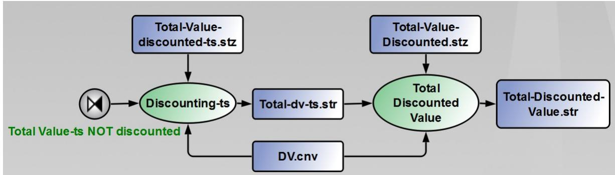
Fig. E.10: Second sub-composite, Discounted Value Calculation. Given a discount factor value, it calculates the total discounted value of the project which is the objective function for optimization.
