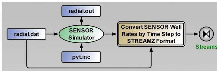
**Fig. E.5:** Reservoir Simulator composite which launches SENSOR reservoir simulation and converts SENSOR output into *STREAMZ* format compatible with Pipe-It.
