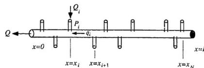
**Fig. 2.2:** Schematic of horizontal perforation model. In varying  $\Delta x = x_{i+1} - x_i$ , we can make perforation density not uniform and counterbalance uneven inflow [Landman 1991].
