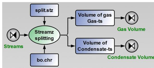
**Fig. 3.11:** Products Separation composite. Hydrocarbons stream is divided in two streams, Oil stream and Gas stream, using a Black-Oil characterization.
