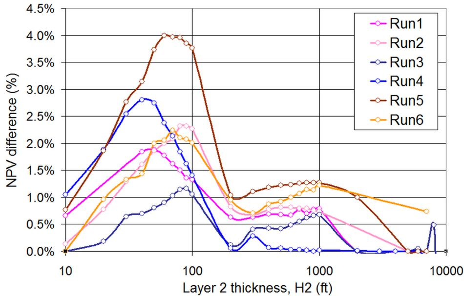
**Fig. 4.10:** Total Discounted Value increase versus *Layer 2* thickness. This plot is obtained using seven different reservoirs (seven Master cases after last filtering constraint introduction). *Layer 2* thickness varies between 10 ft and 10000 ft (on a log scale) while thickness ratio  $\frac{H_1}{H_2}$  is maintained constant for each run. Results show that not only thickness ratio counts but values of layer thickness have also a significant importance.
