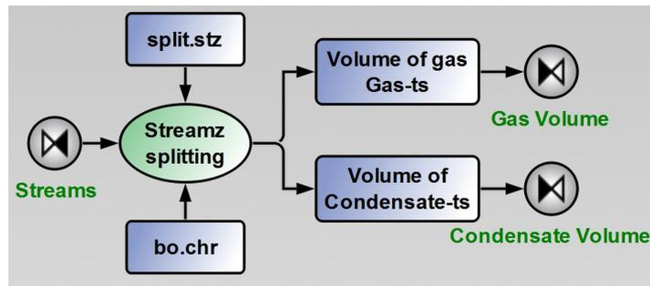
Fig. E.7: Products Separation composite. Hydrocarbons stream is divided in two streams, Oil stream and Gas stream, using a Black-Oil characterization.
