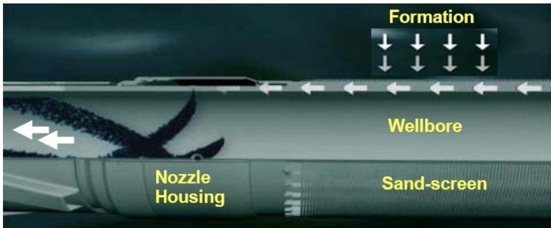
**Fig. 2.5:** ICD based on nozzle concept. Nozzles perforated in the base pipe provide required pressure drop [Shahri 2009].
