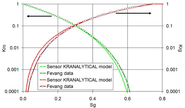
(e) Oil and gas relative permeability versus gas saturation on a semi-logarithmic scale.
