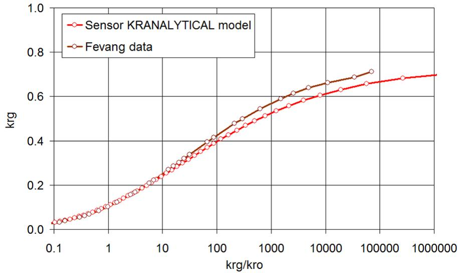
(a) Gas relative permeability versus relative permeability ratio  $\frac{K_{rg}}{K_{ro}}$  on a semi-logarithmic scale.
