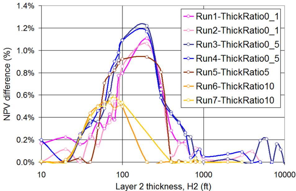
**Fig. 4.11:** Total Discounted Value increase versus *Layer 2* thickness. This plot is obtained using seven different reservoirs (seven Master cases after last filtering constraint introduction). *Layer 2* thickness varies between 10 ft and 10000 ft (on a log scale) while thickness ratio  $\frac{H_1}{H_2}$  is maintained constant for each run. Results show that not only thickness ratio counts but values of layer thickness have also a significant importance.
