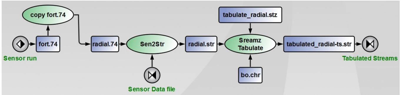
Fig. E.6: Sub-composite of Reservoir Simulator composite showing the details on how SENSOR output is converted into *STREAMZ* format.
