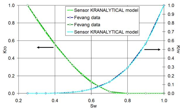
(b) Oil and water relative permeability versus water saturation on a linear scale.
