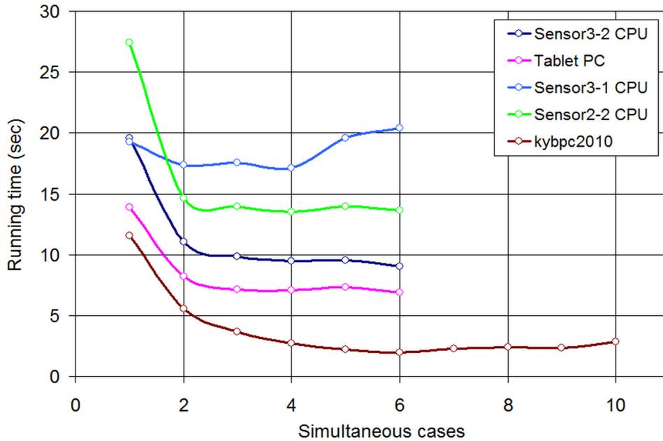
**Fig. 4.7:** Running time versus number of cases executed simultaneously for different computers. This plot shows that for computers comprising more than one CPU, running a single case at a time is not the most efficient strategy.
