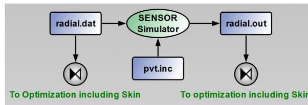
**Fig. E.2:** Organization of the inside of Reservoir Initialization composite which launches SENSOR reservoir simulation.
