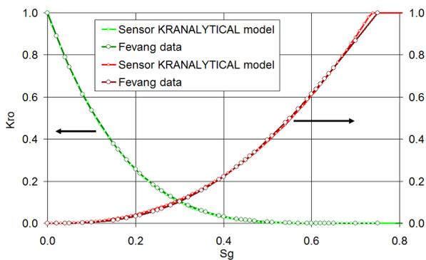
(d) Oil and gas relative permeability versus gas saturation.
