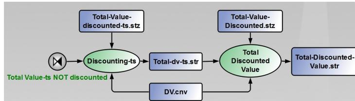
**Fig. 3.14:** Second sub-composite, Discounted Value Calculation. Given a discount factor value, it calculates the total discounted value of the project which is the objective function for optimization.
