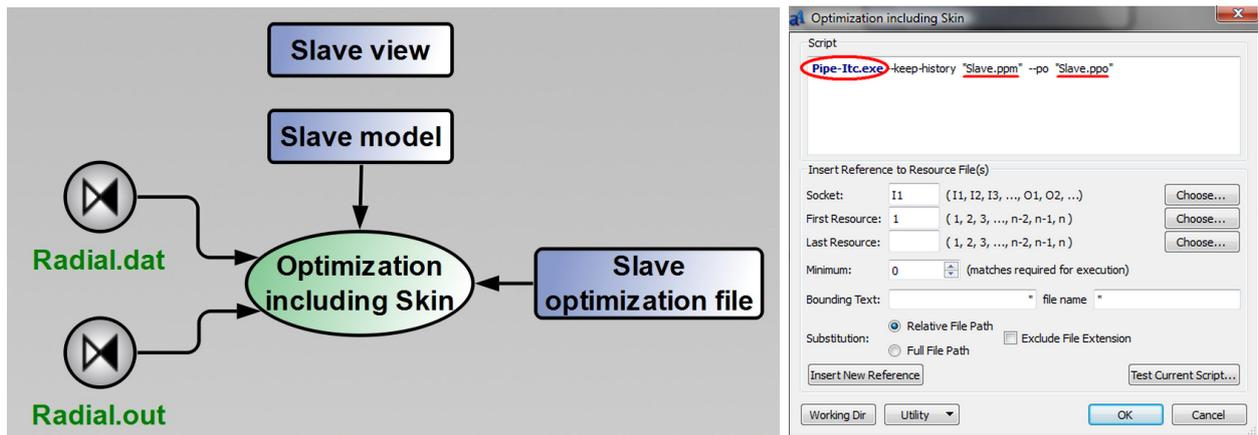
(a) Link to Slave project structure. The process "Optimization including Skin" executes Pipe-ItC to run Slave project and optimization. (b) Script associated to Optimization Including Skin process. Using PipeItC, it executes Slave project run and optimization.
