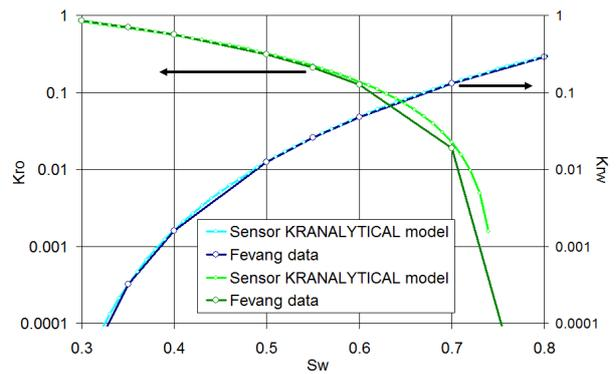
(c) Oil and water relative permeability versus water saturation on a semi-logarithmic scale.
