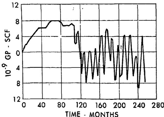
FIG. 5 — CUMULATIVE GAS PRODUCTION AS A FUNCTION OF TIME.
