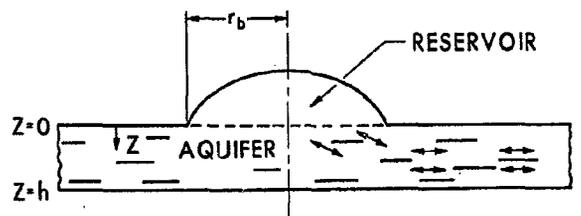
FIG. 2b — IDEALIZED FLOW MODEL FOR BOTTOM-WATER-DRIVE SYSTEM.
