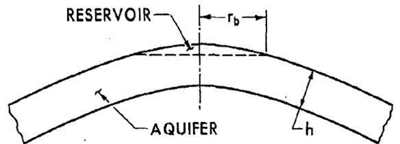
FIG. 2a — BOTTOM-WATER-DRIVE FLOW SYSTEM.
