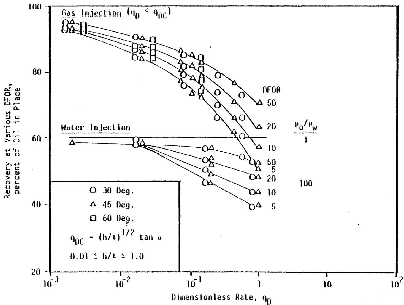
Figure 13. Correlation of Recovery with Dimensionless Rate for Dip Angles Between 30 and 60 Degrees
