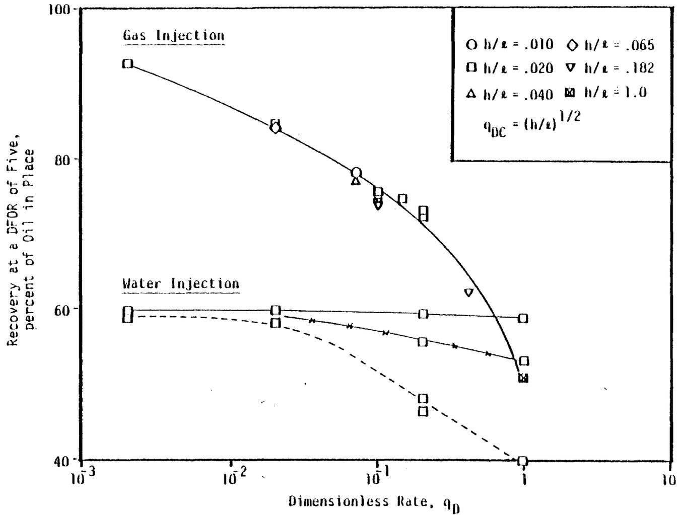
Figure 12. Comparison of Oil Recovery from Gas and Water Injection Runs at a Dip of 45 Degrees for Various Values of the Height to Length Ratio
