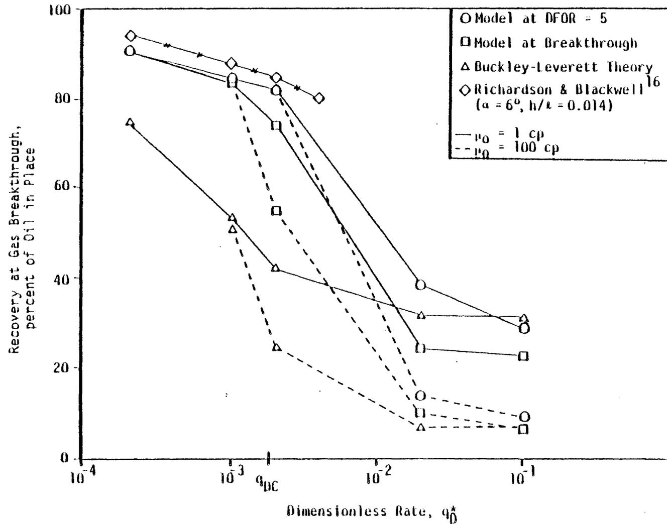
Figure 6. Comparison of Oil Recovery from Base Case Gas Injection Runs at a Dip of 5 Degrees
