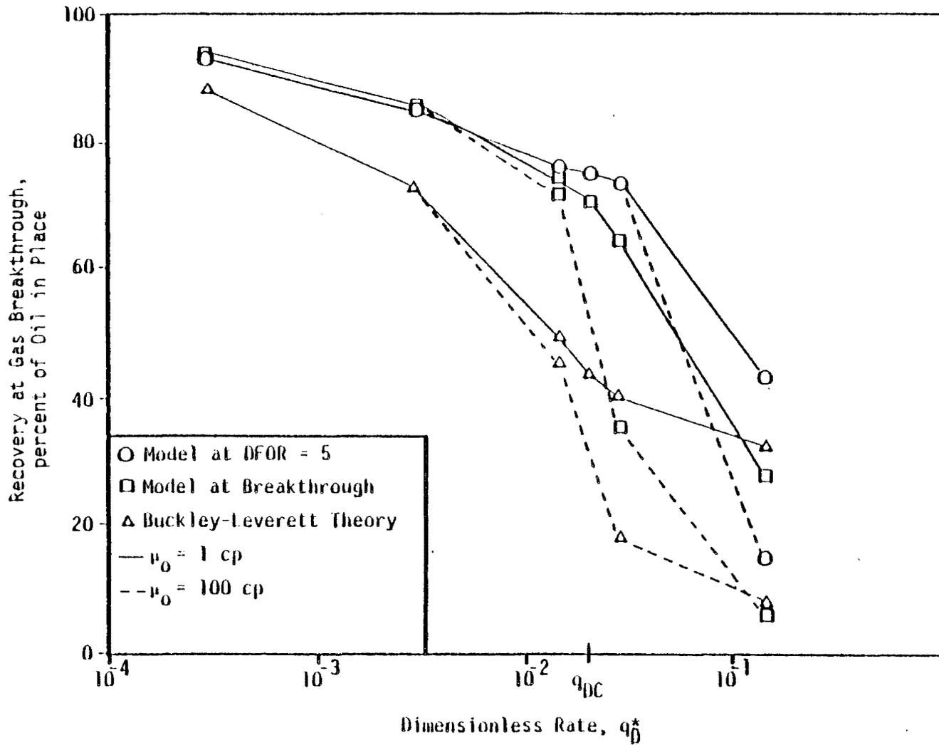
Figure 8. Comparison of Oil Recovery from Base Case Gas Injection Runs at a Dip of 45 Degrees
