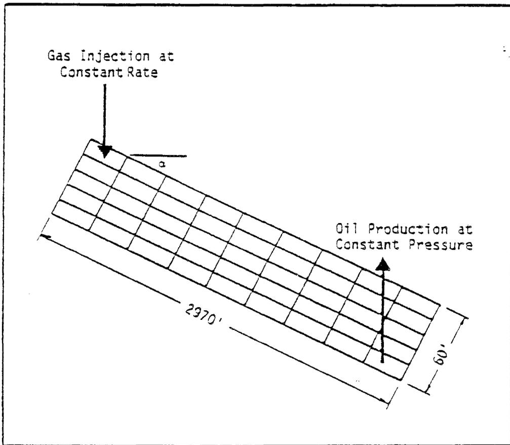
Figure 1. Diagram of Model for Base Case Gas Injection Runs
