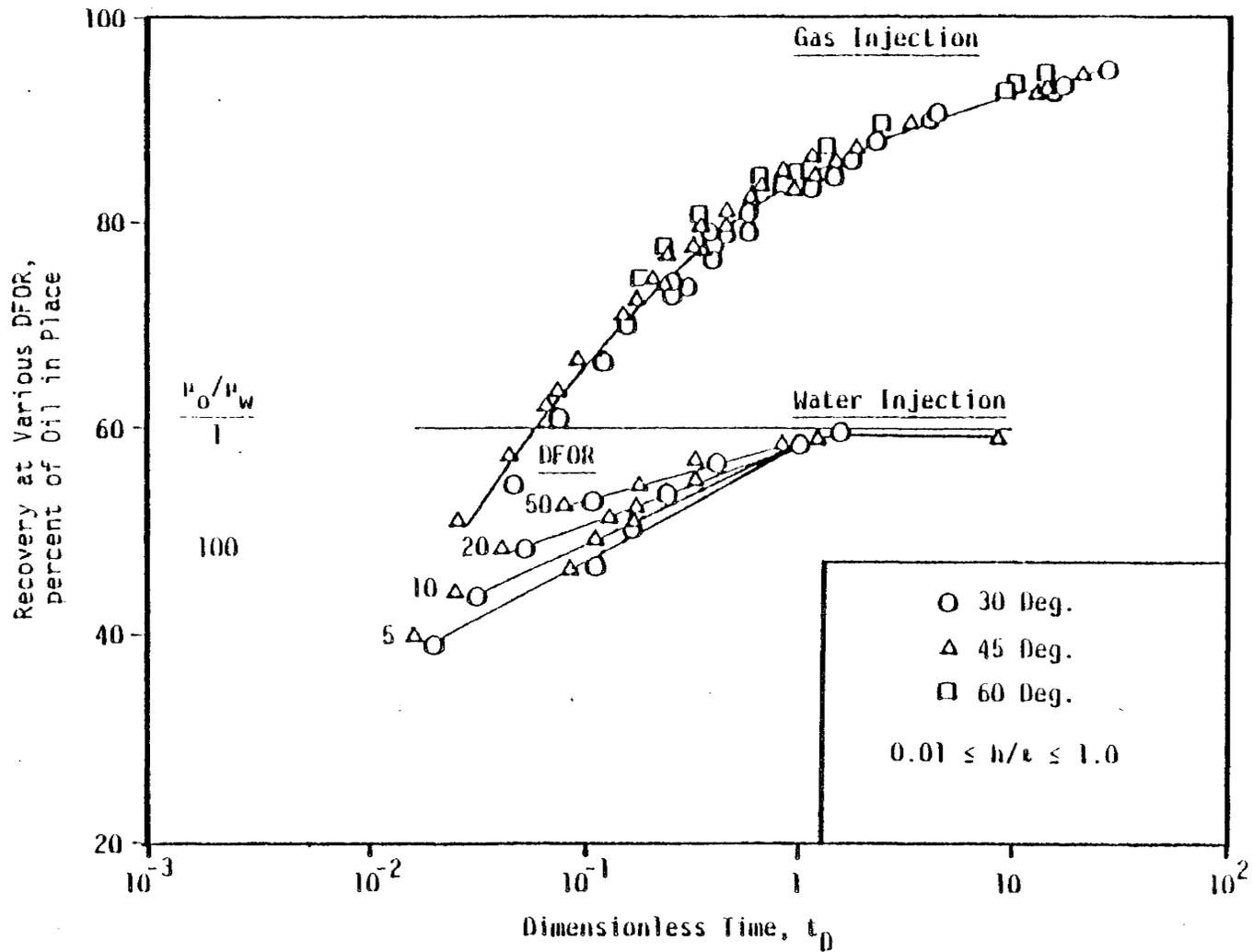
Figure 14. Correlation of Recovery with Dimensionless Time for Dip Angles Between 30 and 60 Degrees
