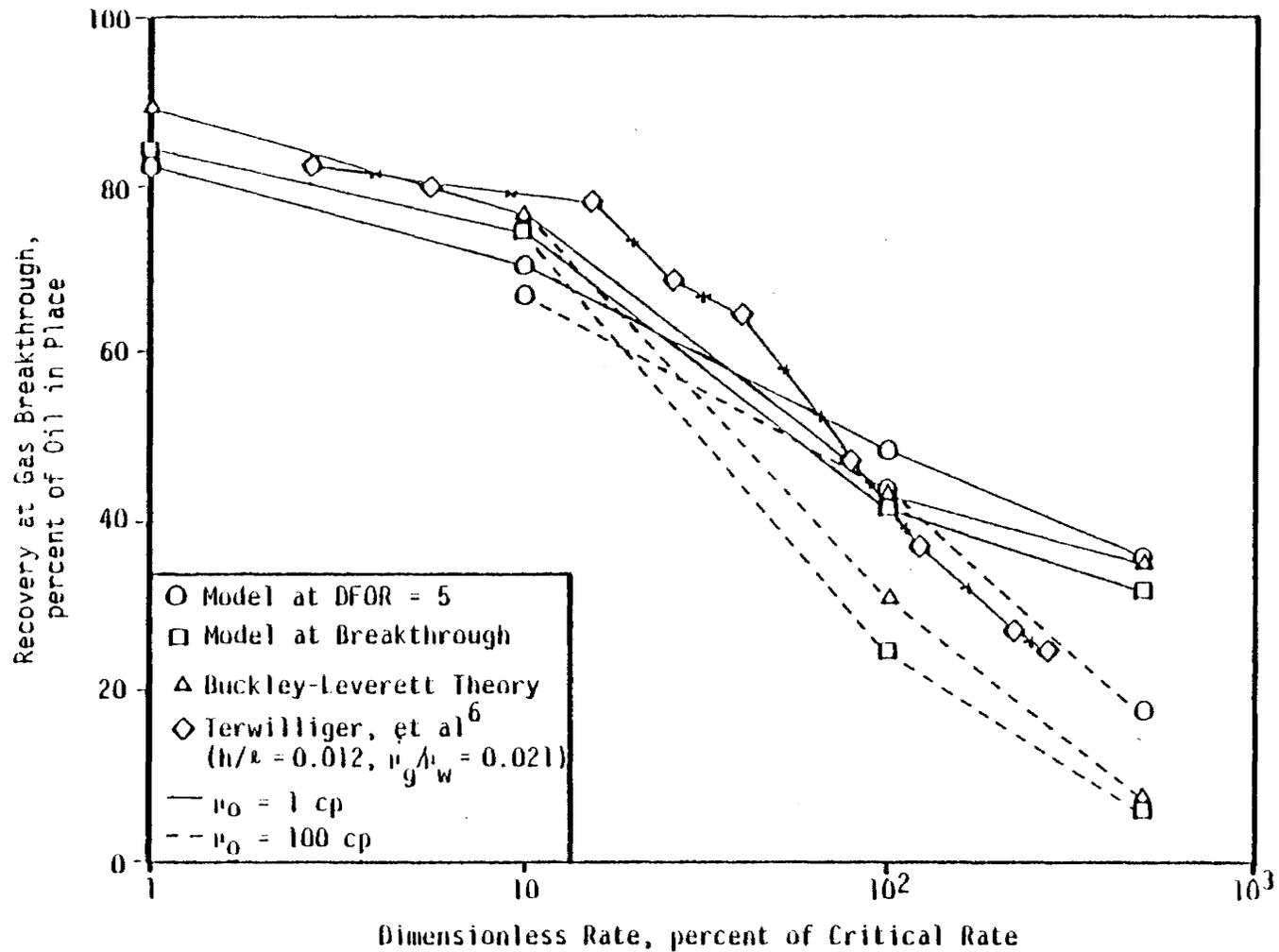
Figure 7. Comparison of Oil Recovery from Base Case Gas Injection Runs at a Dip of 90 Degrees
