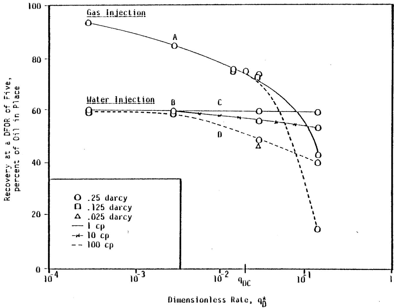
Figure 10. Comparison of Oil Recovery from Gas and Water Injection Runs at a Dip of 45 Degrees for Various Values of Vertical Permeability
