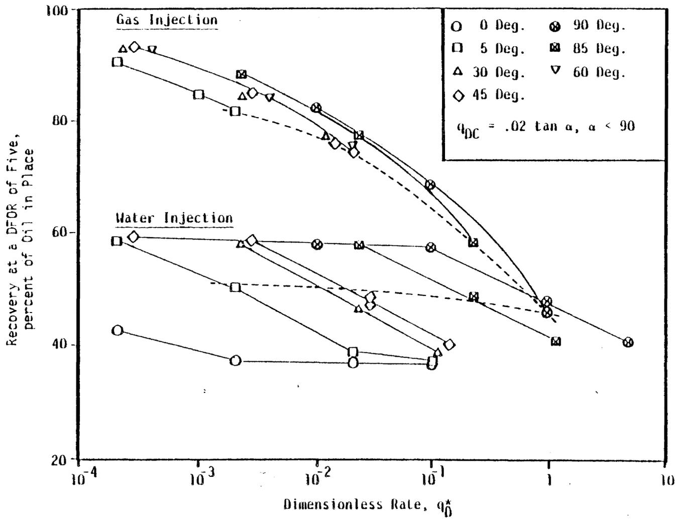
Figure 11. Comparison of Oil Recovery from Base Case Gas and Water Injection Runs at Various Dip Angles
