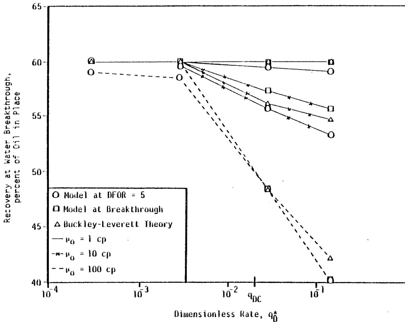
Figure 9. Comparison of Oil Recovery from Base Case Water Injection Runs at a Dip of 45 Degrees
