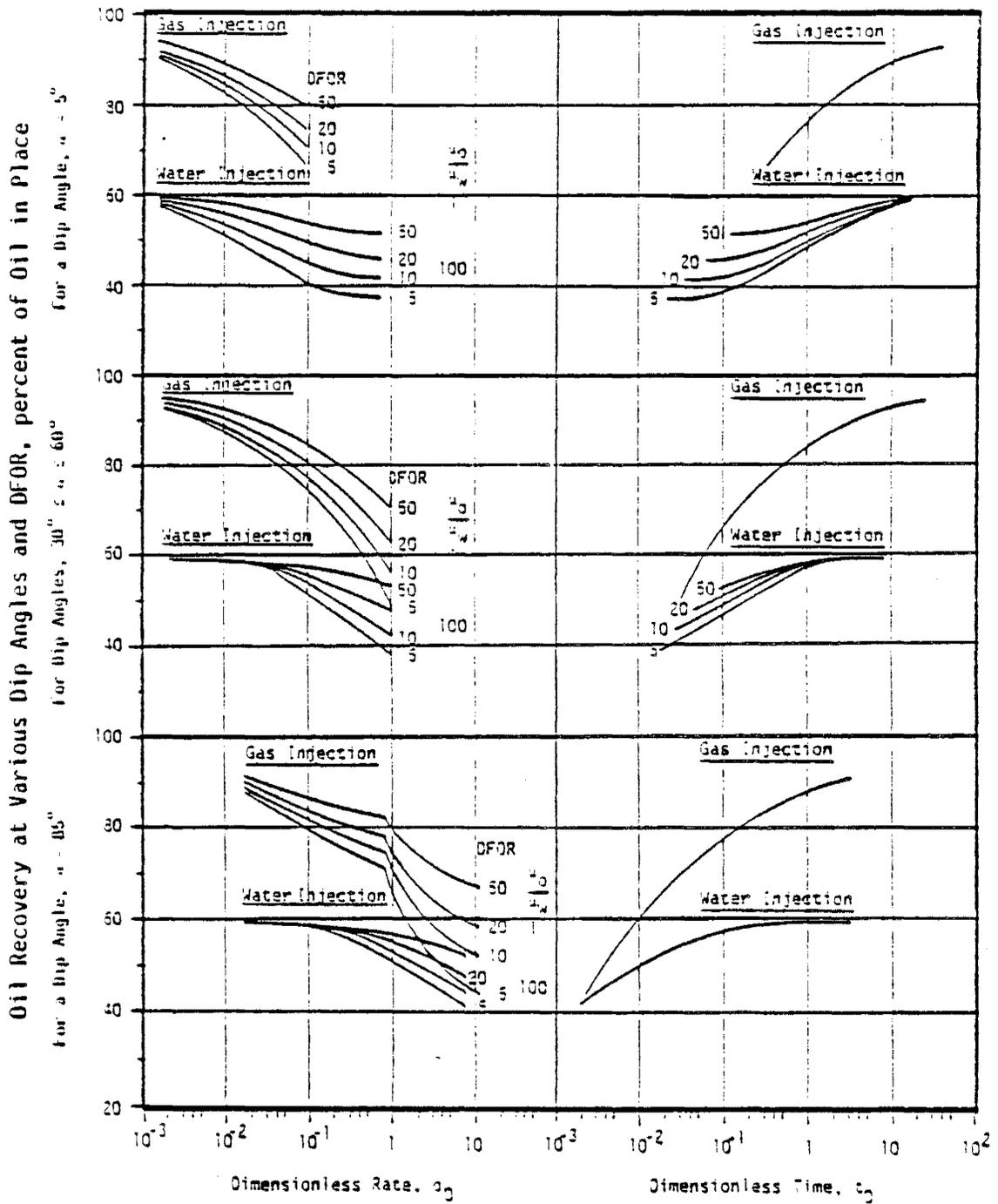
Figure 5. Correlation of Oil Recovery with Dimensionless Rate and Time
