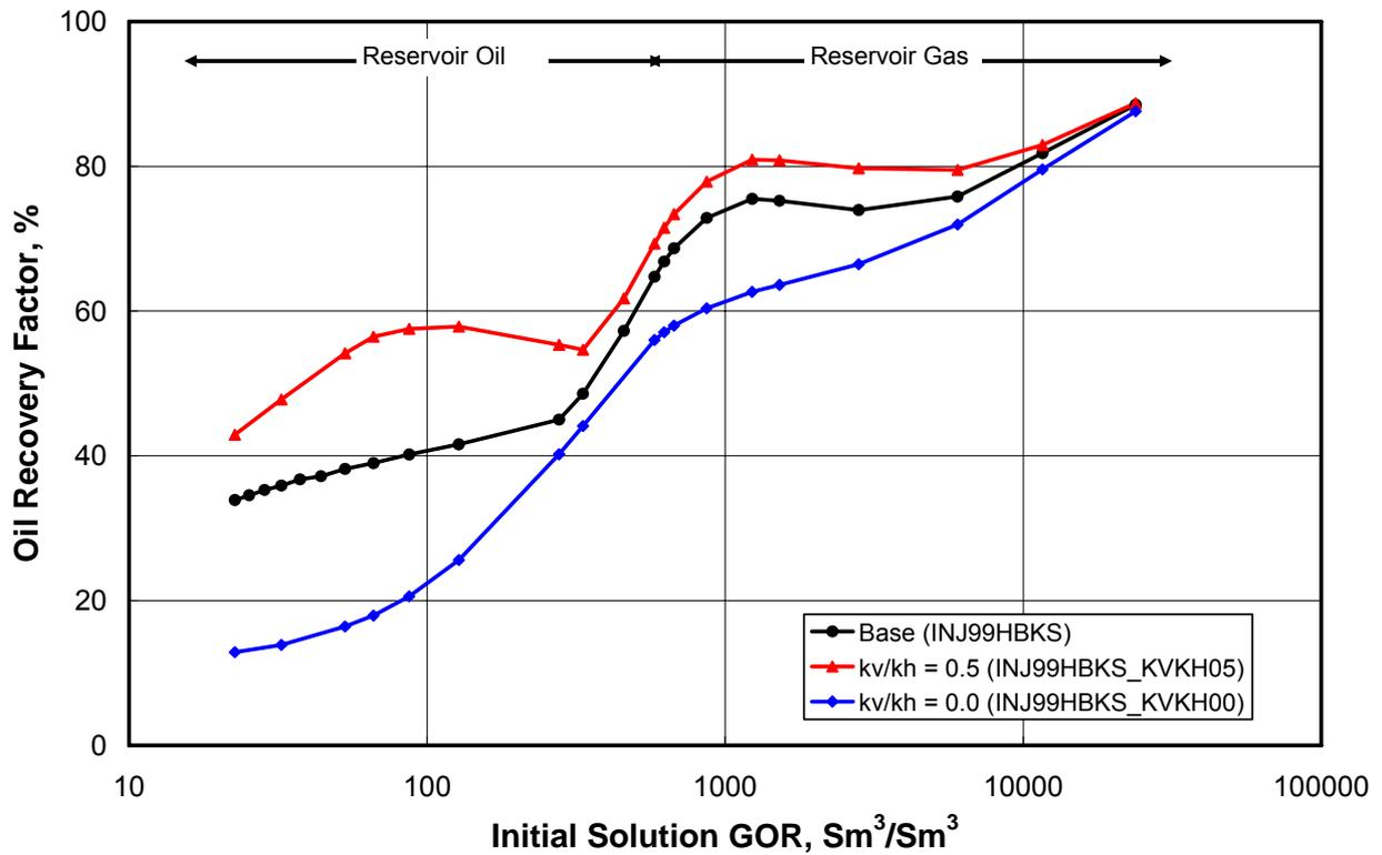
Fig. 14 — Effect of vertical/horizontal permeability ratio on the oil recovery – (a) base case:  $k_v/k_h = 0.1$  (b) sensitivity cases:  $k_v/k_h = 0.5$  and  $0.0$ .
