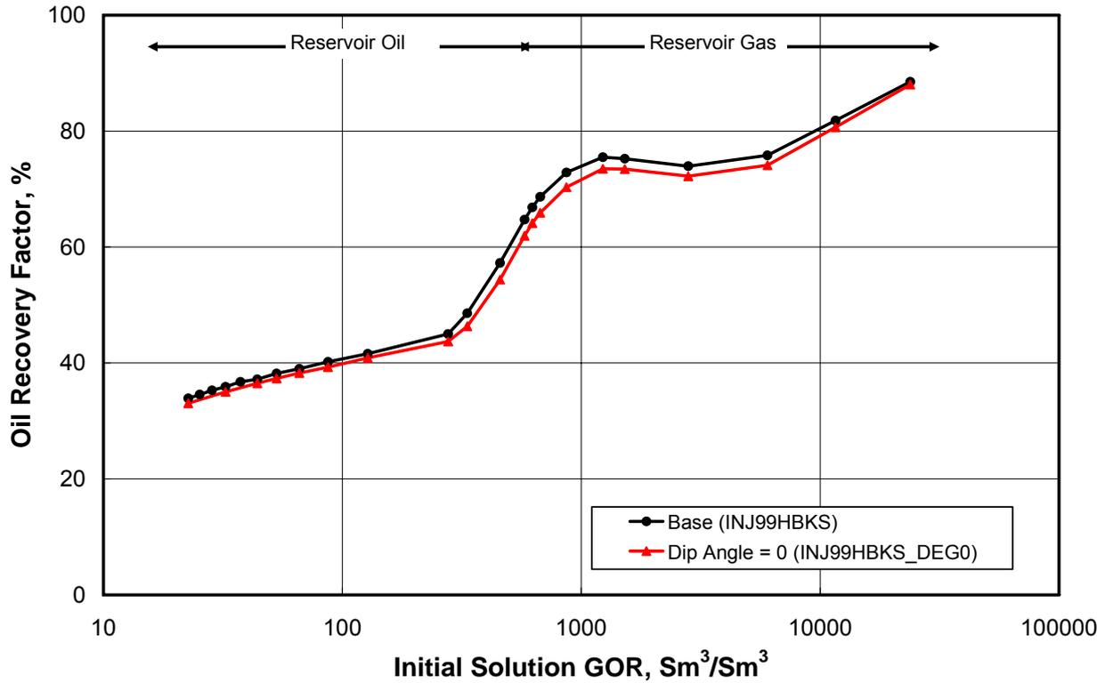
Fig. 19 — Effect of dip angle on the oil recovery – (a) base case: dip angle 3.8 degrees (b) sensitivity cases: dip angle 0 degree).
