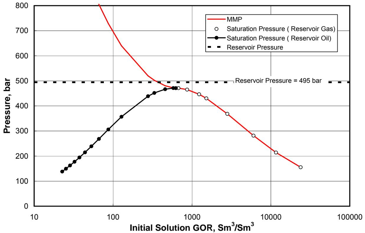
Fig. 5 — Calculated minimum miscibility (with lean injection gas) pressures for different fluid systems. The MMP of the reservoir gas system is equal to the dewpoint pressure of the gas. For oil system, the MMP is higher than the bubblepoint pressure of the oil.
