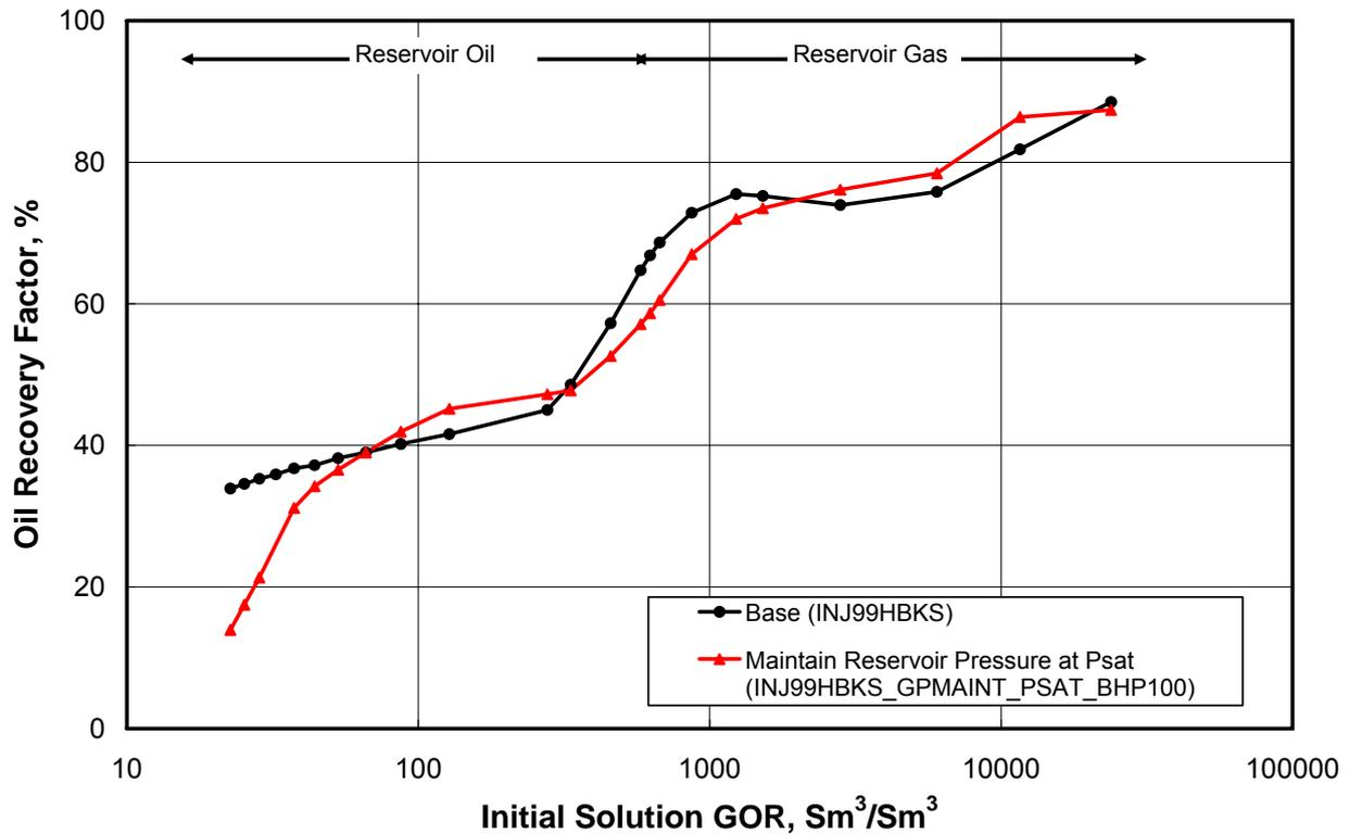
Fig. 17 — Effect of pressure maintenance at lower pressure – (a) base case: the reservoir pressure is maintained at the initial reservoir pressure (b) sensitivity case: the reservoir pressure is maintained at the saturation pressure of the initial reservoir fluid.
