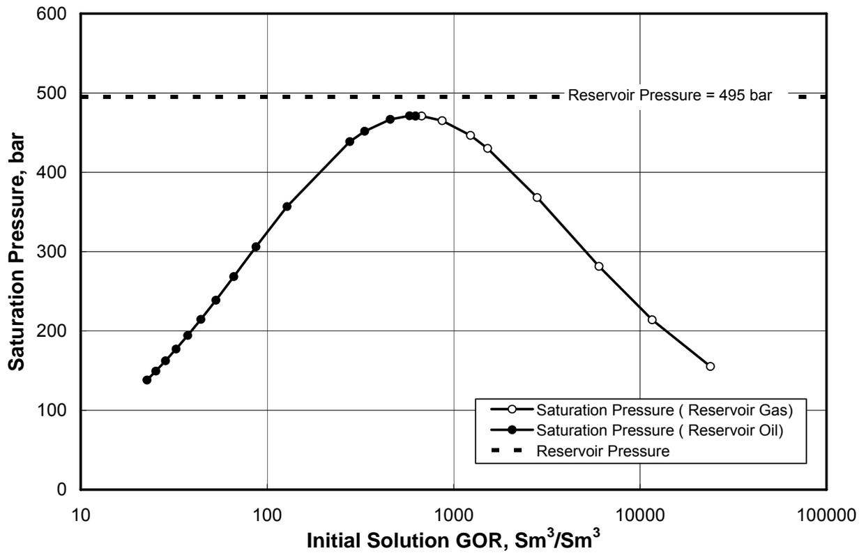
Fig. 2 — Saturation pressure variation with initial solution GOR for different fluid system.
