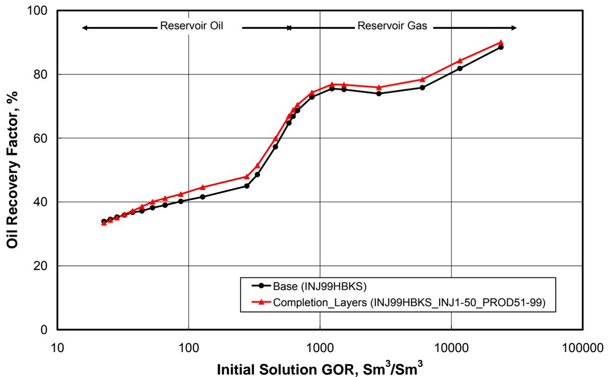
Fig. 18 — Effect of well completion on the oil recovery – (a) base case: the producer and the injector are completed in all layers (b) sensitivity case: the injector is completed in the upper half (numerical layer 1-50) and the producer is completed in the lower half (numerical layer 51-99) of the reservoir.
