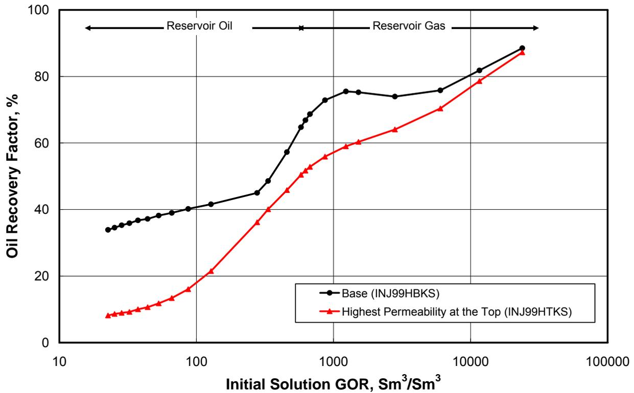
Fig. 12 — Effect of permeability distribution on the oil recovery – (a) base case: the highest permeability is at the bottom (b) sensitivity case: the highest permeability is at the top.
