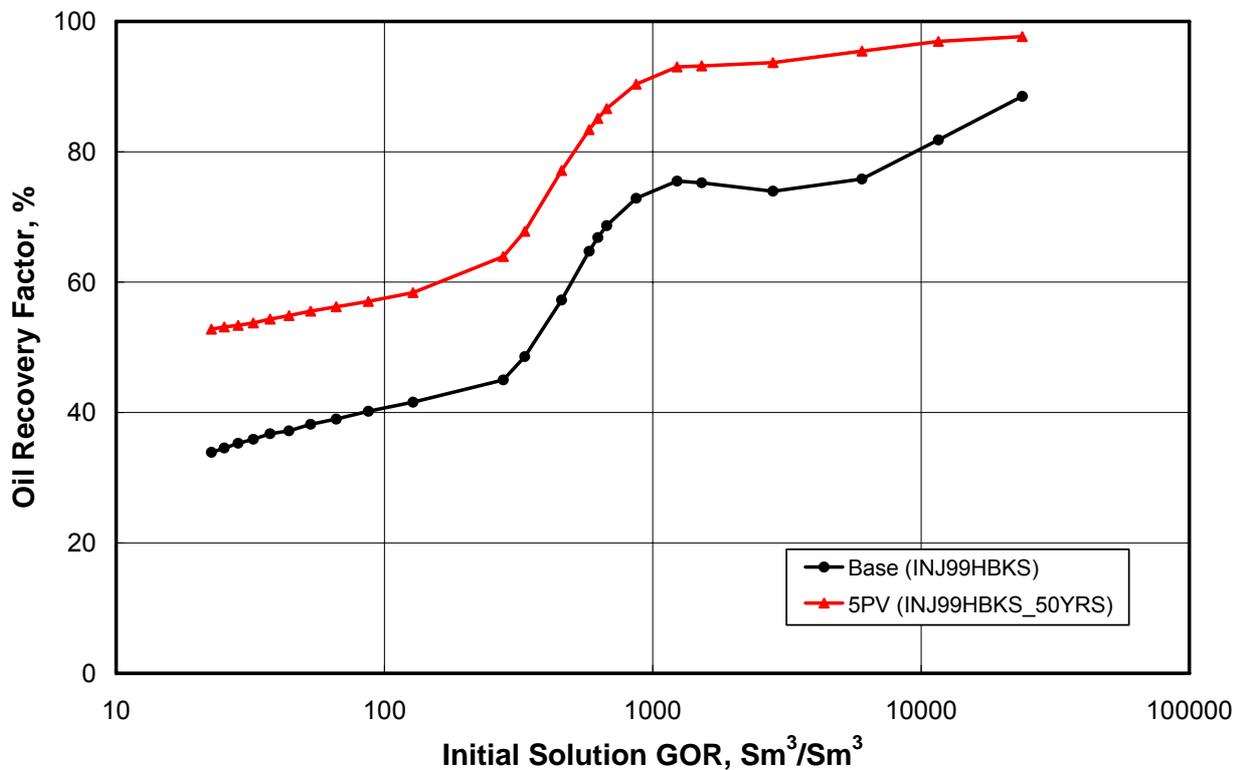
Fig. 8 — Effect of amount of gas injection on the oil recovery – (a) base case: the reservoir was simulated for 15 years i.e. 1.5 PV gas injection (b) sensitivity case: the reservoir was simulated for 50 years i.e. 5 PV gas injection.
