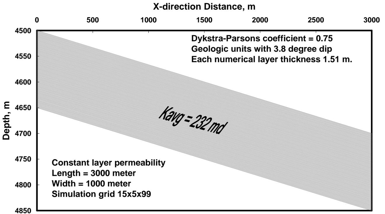
Fig. 4 — 3D 99-layers dipping reservoir simulation model. Thickness of each layer is 1.51 m. Permeability of different layers is different (in the base case, the permeability is 2500 md for the bottom layer and 4 md for the top layer).
