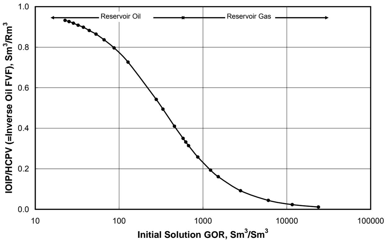
Fig. 6 — Initial oil in place with initial solution gas-oil ratio for different fluids.
