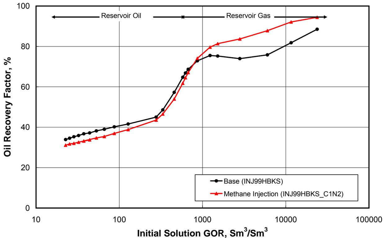
Fig. 16 — Effect of injection gas composition on the oil recovery – (a) base case: lean gas injection (b) sensitivity case: methane gas injection.
