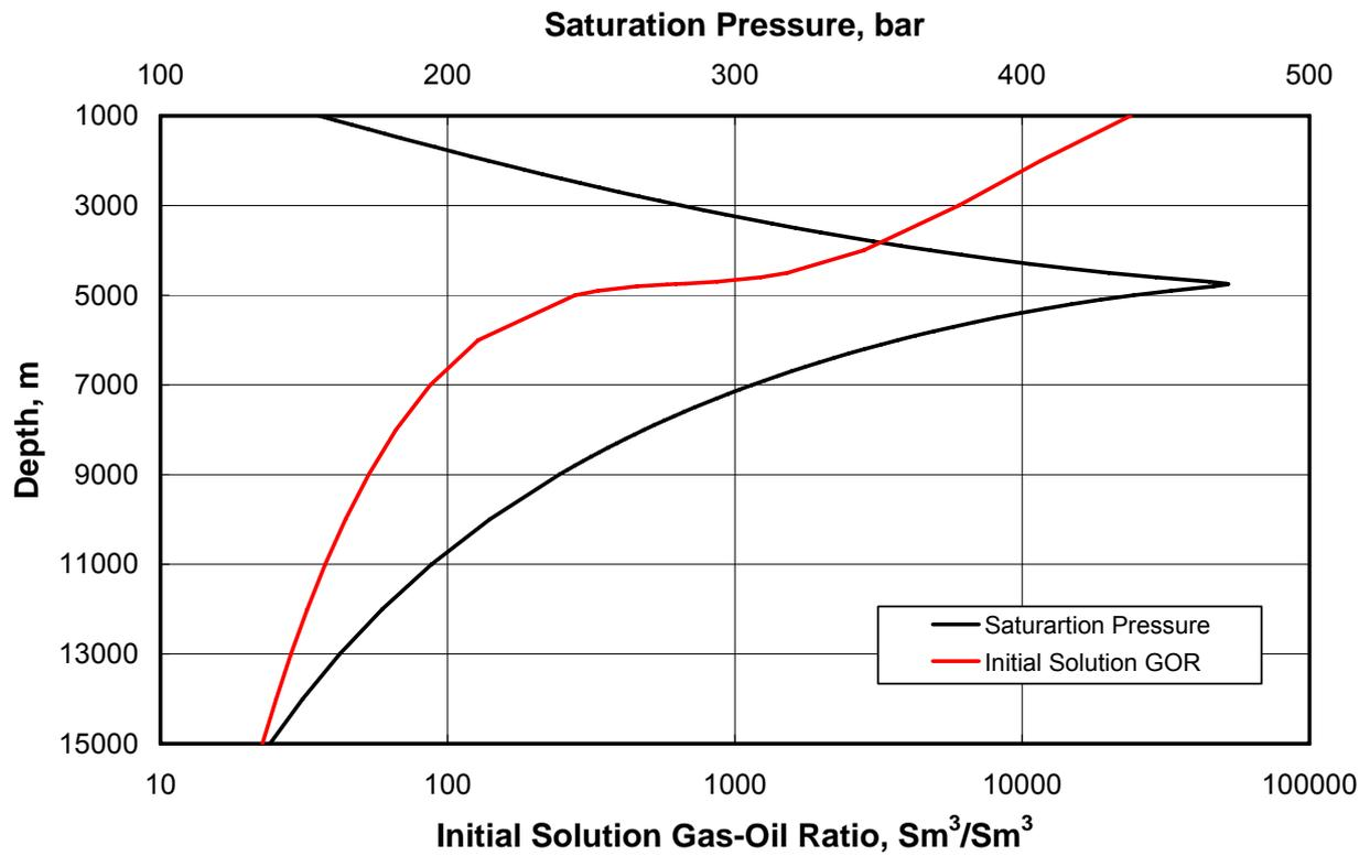
Fig. 1 — Initial solution gas-oil ratio (GOR) and saturation pressure variation with depth for different fluid system.
