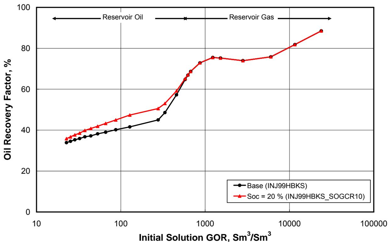
Fig. 10 — Effect of critical oil saturation on the oil recovery – (a) base case: the critical gas saturation is 22% (b) sensitivity case: the critical gas saturation is 10%.
