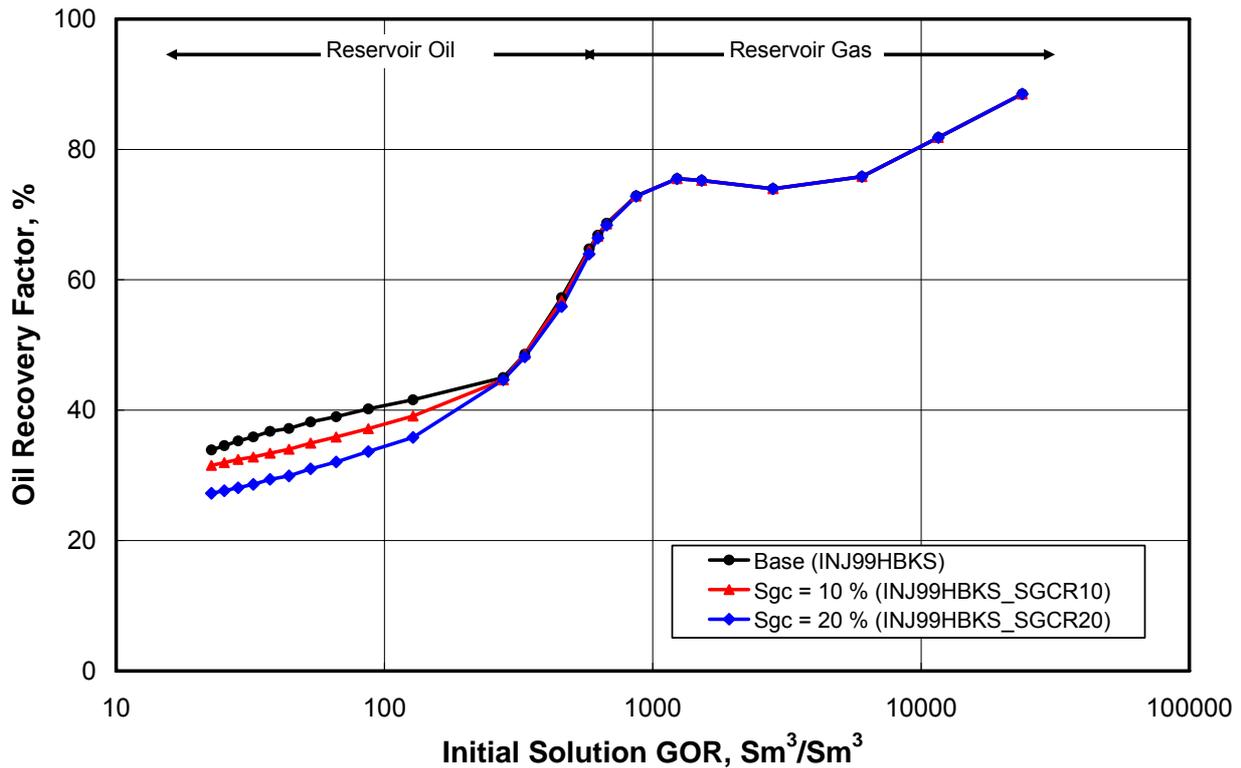
Fig. 9 — Effect of critical gas saturation on the oil recovery – (a) base case: the critical gas saturation is 2% (b) sensitivity cases: the critical gas saturations are 10- and 20-%.
