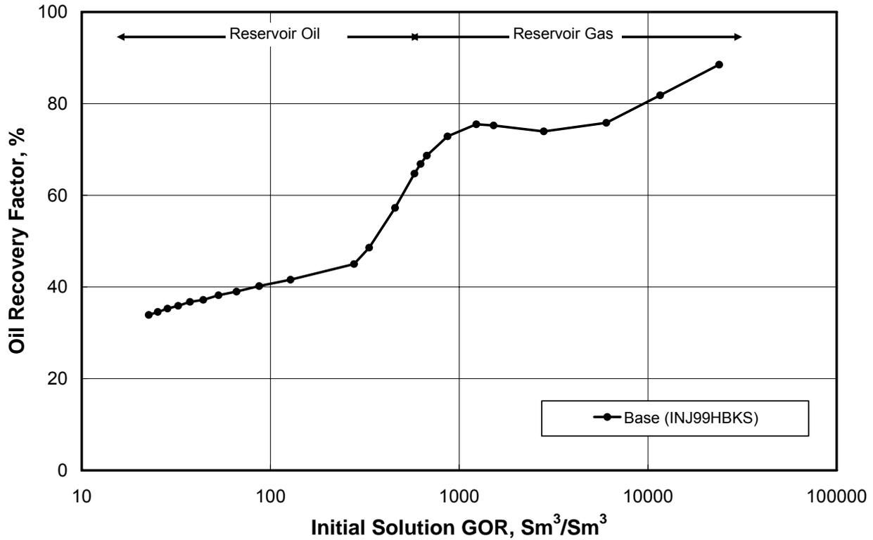
Fig. 7 — Oil recovery in the base case (99-layer case with the highest permeability at the bottom; lean gas injection to maintain the reservoir pressure at the initial reservoir pressure; injection period 15 years i.e. 1.5 PV gas injection; average reservoir permeability equal to 232 md).
