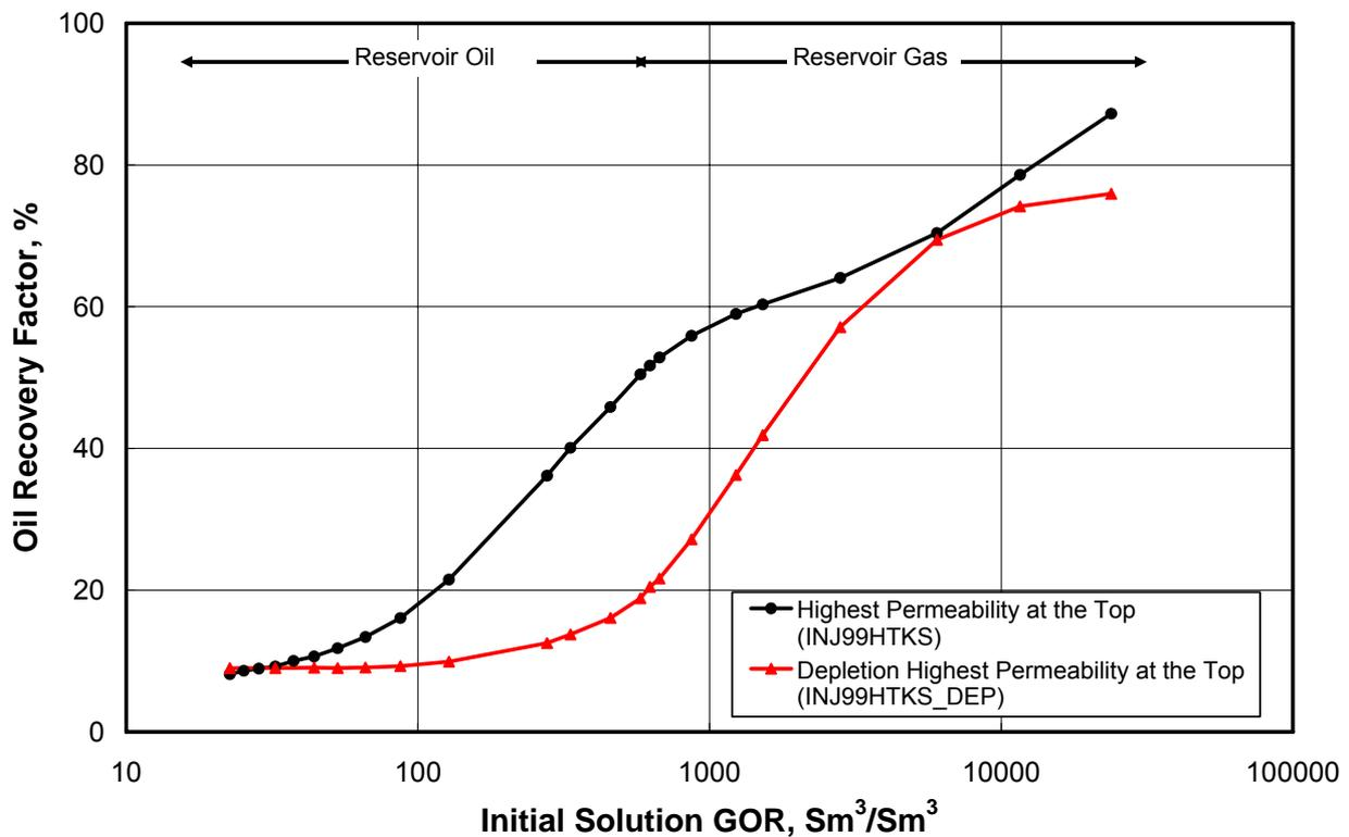
Fig. 22 — Oil recovery under depletion for the case with the highest permeability at the top– (a) full pressure maintenance at the initial reservoir pressure by lean gas injection (b) sensitivity case: depletion.
