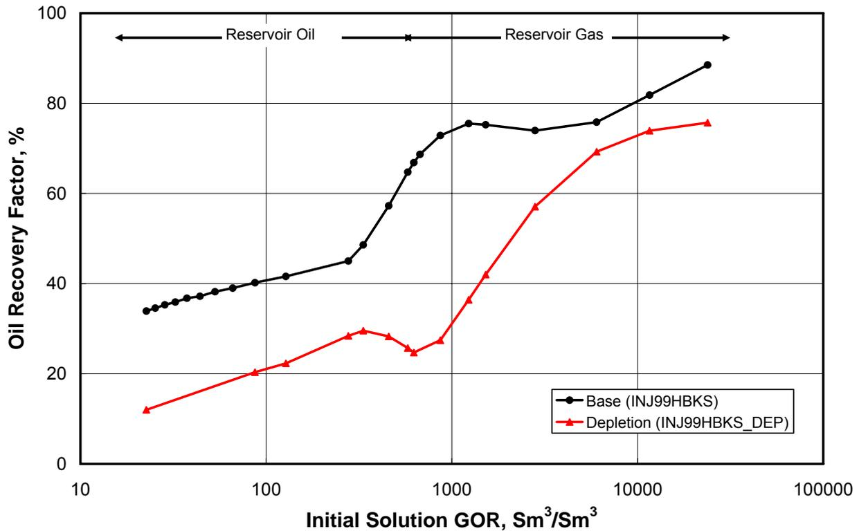
Fig. 21 — Oil recovery under depletion for the case with the highest permeability at bottom – (a) base case: full pressure maintenance at the initial reservoir pressure by lean gas injection (b) sensitivity case: depletion.
