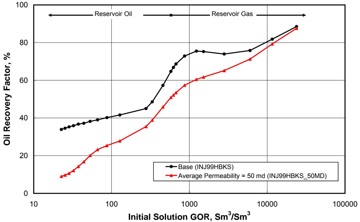
Fig. 11 — Effect of average reservoir permeability on the oil recovery – (a) base case: the average reservoir permeability is 232 md (b) sensitivity case: the average reservoir permeability is 50 md.
