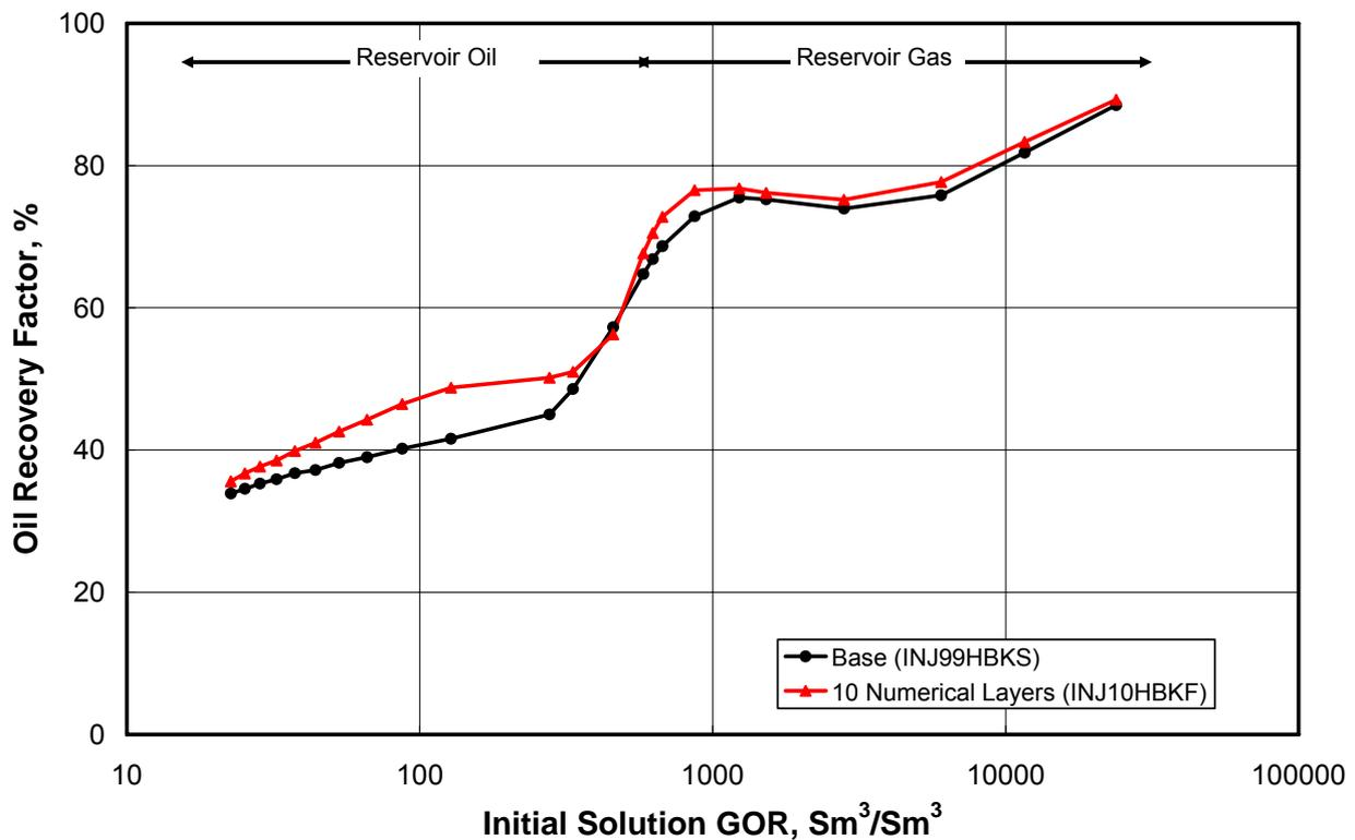
Fig. 20 — Effect of numerical layers on the oil recovery - (a) base case: 99 layers; 15x5x99; each layer with equal thickness (b) sensitivity case: 10 numerical layers; 15x5x10; each layer of equal kh but of different thickness. The total thickness is 150 m in both cases.
