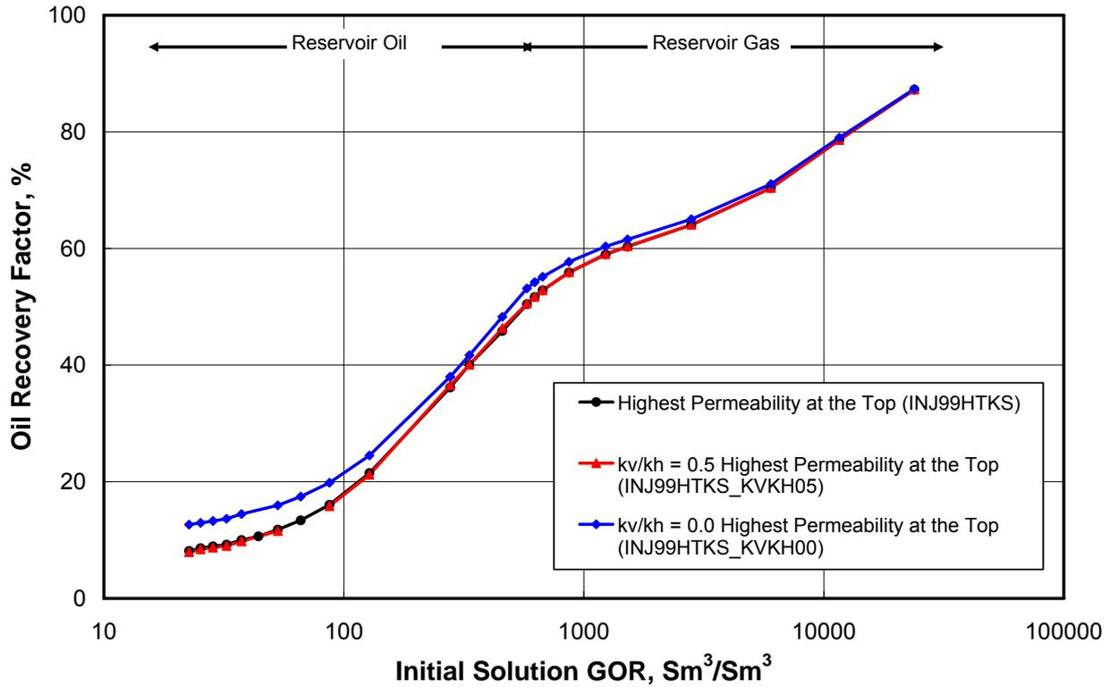
Fig. 15 — Effect of vertical/horizontal permeability ratio on the oil recovery in case of the highest permeability at the top – (a) base case:  $k_v/k_h = 0.1$  (b) sensitivity cases:  $k_v/k_h = 0.5$  and  $0.0$ .
