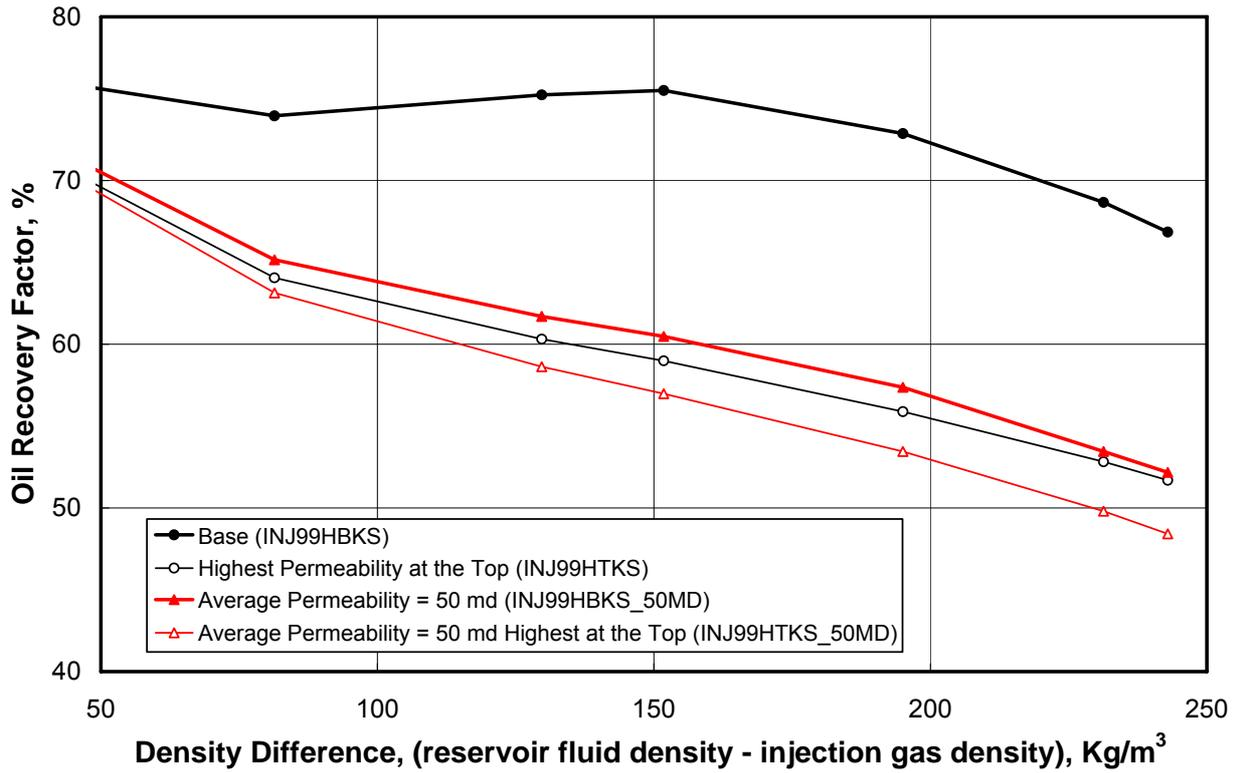
Fig. 13 — Oil recovery variation with average reservoir permeability (a) the highest permeability at the bottom (b) the highest permeability at the top.
