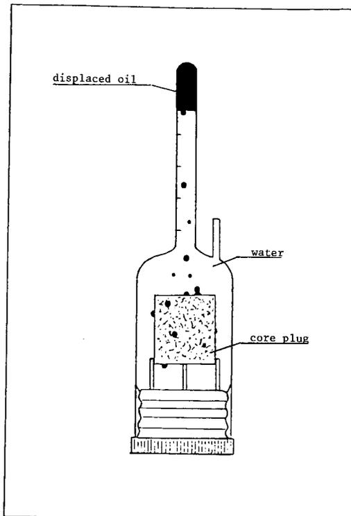
Fig. 3—Imbibition cell with oil-saturated core plug.
