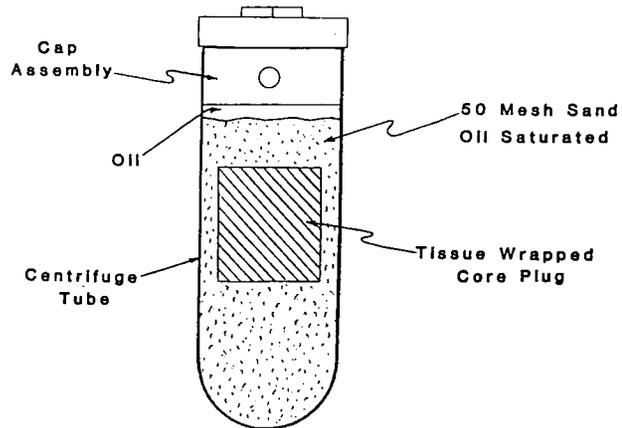
Fig. 2—Core plug loaded into the centrifuge cell for saturating with oil.
