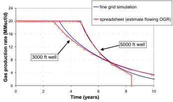
Fig. 11. Production profiles for horizontal well in rich gas condensate reservoir.
