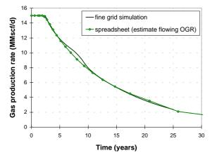
Fig. 8. Gas production profiles for vertical unfractured well, including the change in relative permeability with capillary number and non-Darcy flow.
