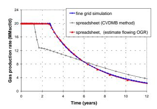
Fig. 10. Production profiles for horizontal well in rich gas condensate reservoir. Well length = 5000 ft,  $k_h$ =0.1md.
