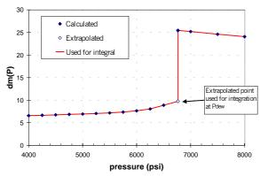
Fig D-1. Calculation of pseudopressure integral.
