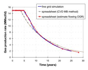
Fig. 7. Gas production profiles for vertical unfractured well, including the change in relative permeability with capillary number.
