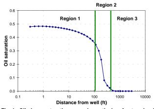
Fig. 1. Oil phase saturation around a vertical, unfractured well. Note log scale for distance from well.
