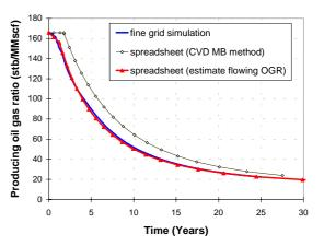
Fig. 5. Producing oil-gas ratio for vertical unfractured well, ignoring high-velocity effects.
