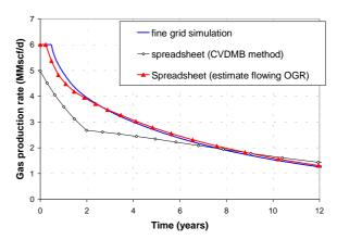
Fig. 9. Gas production profiles for fractured well, with fracture half-length = 100 ft.
