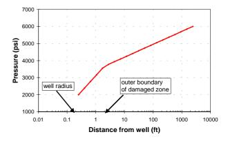
Fig C-1. Pressure distribution around a vertical unfractured well with skin from formation damage.
