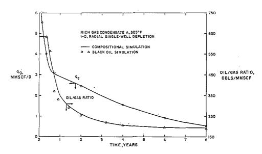
Fig. 4—Comparison of black-oil and compositional simulation results.
