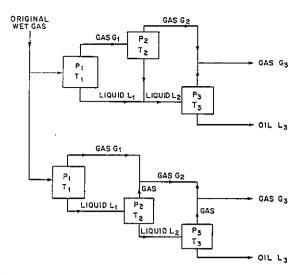
Fig. 1—Examples of gas condensate separation yielding two components—oil and gas.
