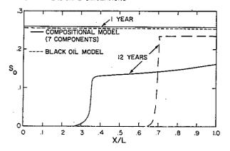
Fig. 6—Calculated oil saturation profiles after 11 years of cycling.
