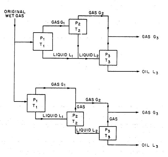
FIGURE 1 EXAMPLES OF GAS CONDENSATE SEPARATION YIELDING TWO COMPONENTS "OIL"AND "GAS" RICH GAS CONDENSATE A, BOTTOMHOLE SAMPLE, 325 °F CONSTANT COMPOSITION EXPANSION
