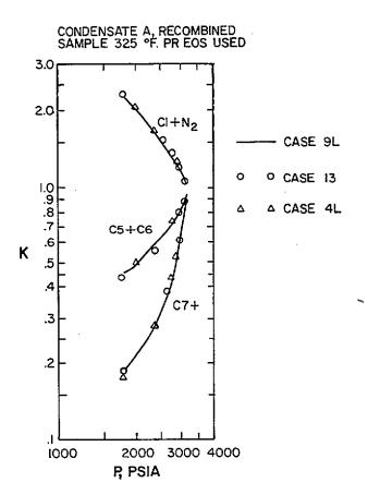
Fig. 9—Lumped fraction K values calculated from constant composition expansion.
