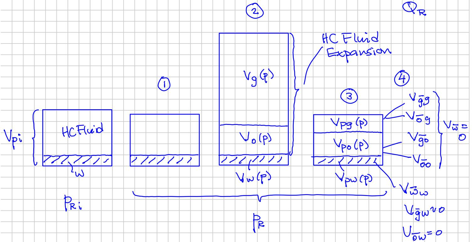
② Reservoir Fluid (Gas  $\neq$  Oil) Volumetric & Phase Behavior
