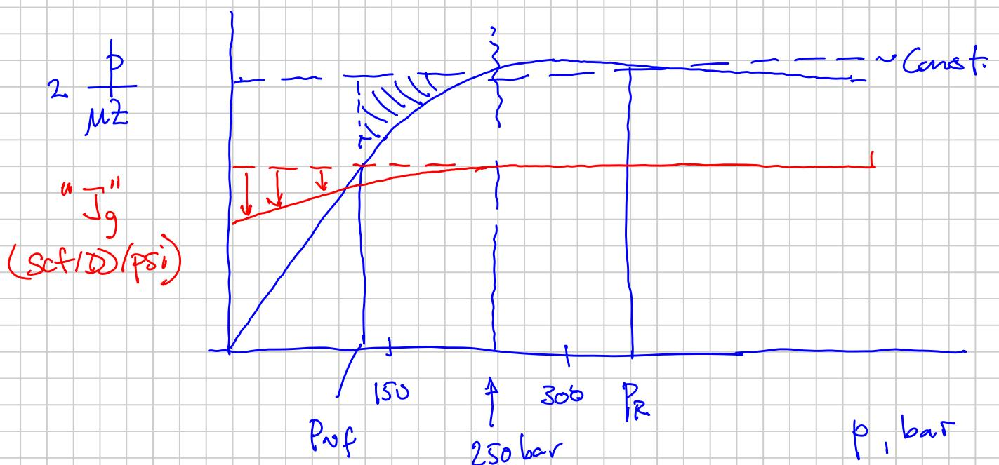
$$q_g = J_g (P_R - P_{wf}) = \frac{(\pi T_{sc})}{P_s} \frac{k h}{T_R \ln \frac{r_e}{r_w}} \left( 2 \frac{p}{Mz} \right) \cdot \int_{P_{wf}}^{P_R} dp$$
